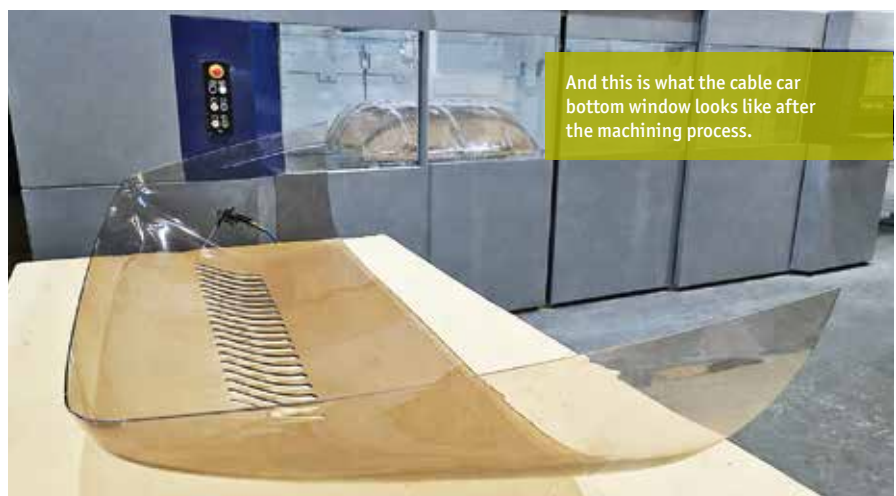
A cable car bottom window is being finalised in the 5-axis CNC machining centre.
