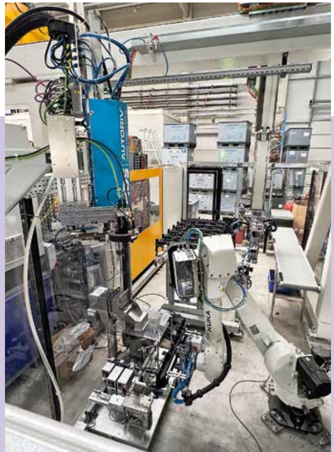
The injection moulding of the cooling air inlets and the assembly processes in an 8,000 kN injection moulding machine are also fully automated.
