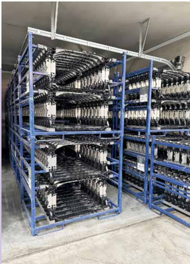
Thanks to specially designed holders, the plastic mounting brackets can be transported in the special load carrier.
