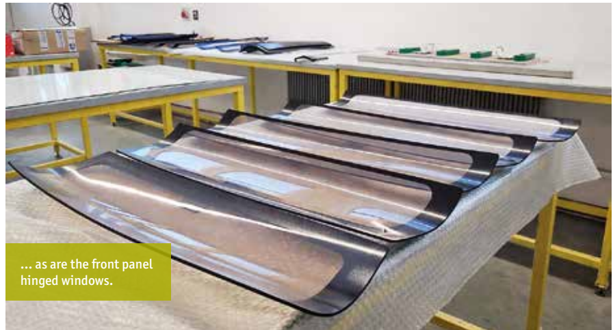
The windows of the C10 cabin are also made of PET-G ...
