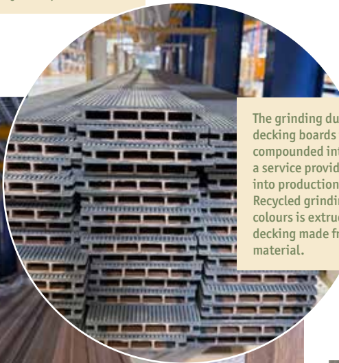
In the milling room, ttp grinds start-up waste, punching waste and production rejects, mixes the ground material, fills it into big bags and reuses it for the middle layers of profiles.
