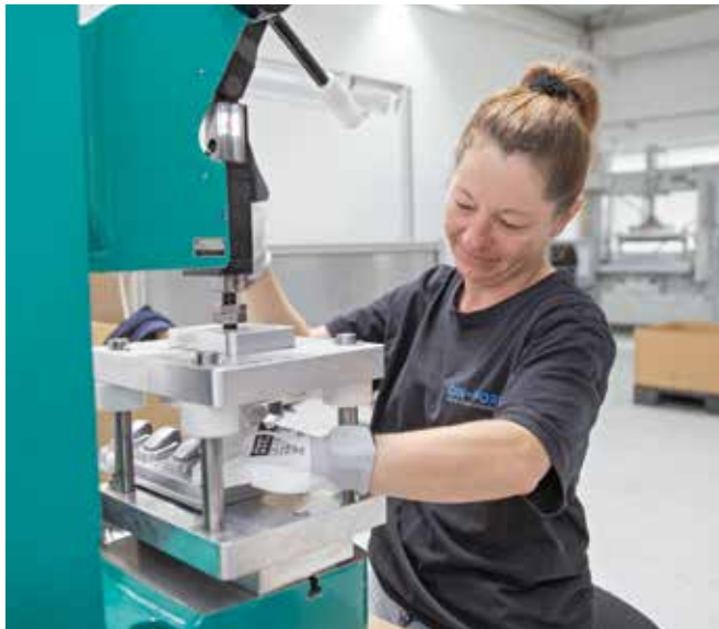
The punching machines are located in the room next to the CNC machines. An employee punches out an insert.
