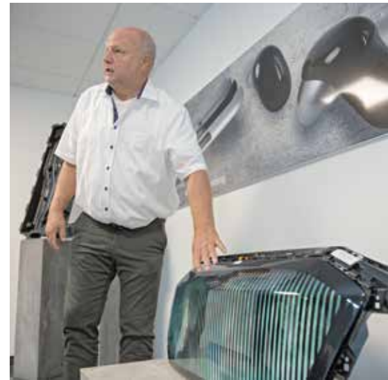
The front panel of an electric vehicle can be customised with screen-printed inserts. At injection moulding partner RESRG, the insert is pre-moulded with a 3 mm PC layer, and in the next step, the retaining edge is back-moulded.
