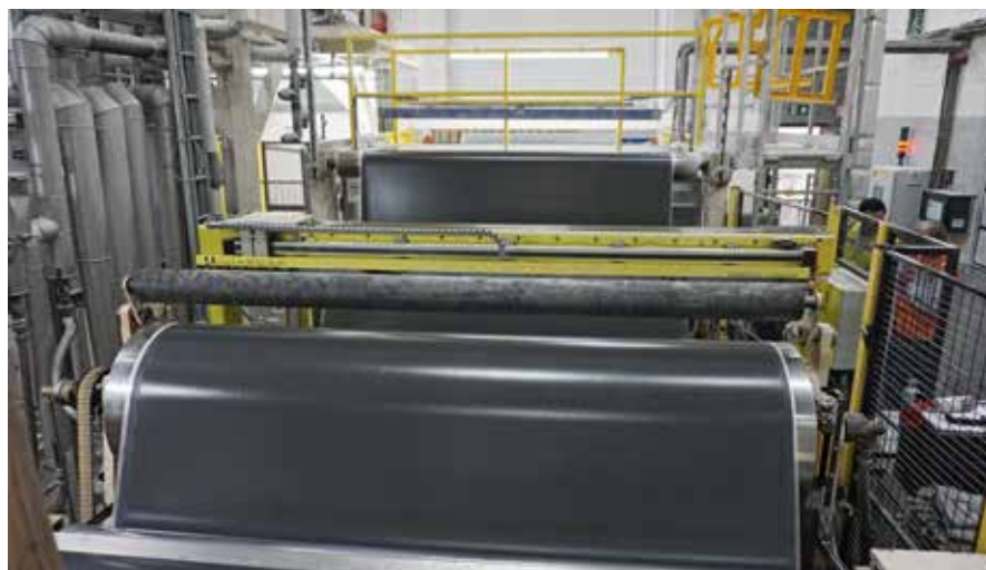
In the 3-roll calender, the thin glass fibre fabric is coated on both sides with the PVC mixture from the Entex PWE.
