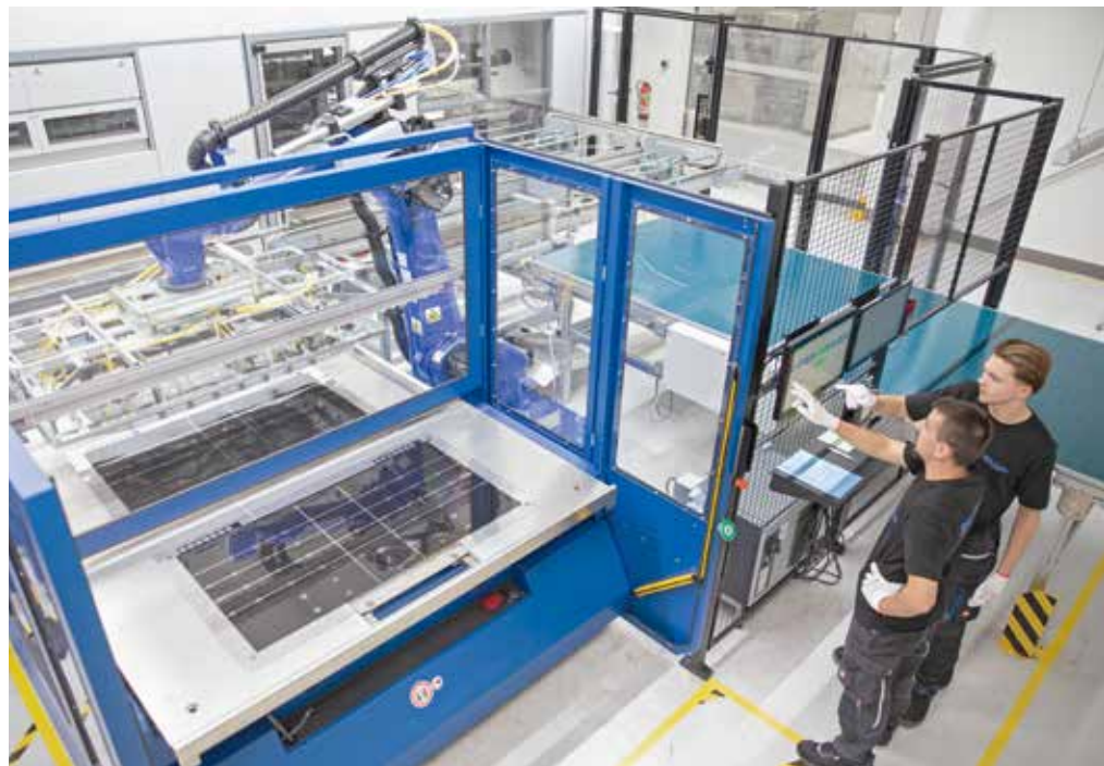
The thermoforming machine for printed sheet material is fully automated.
