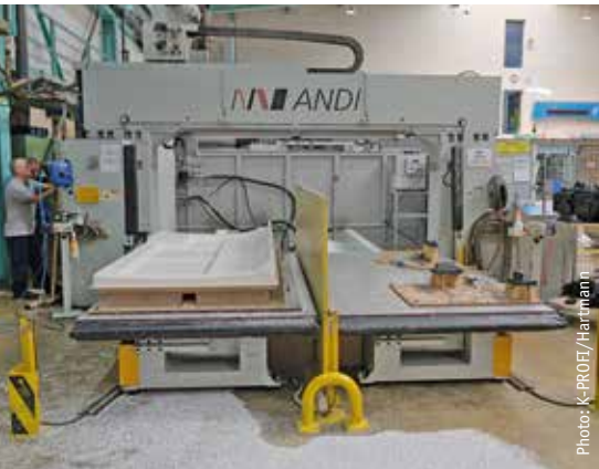
The CNC systems are designed as tandem machines. If very large components need to be milled, the tables are coupled together.
