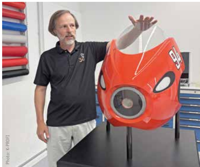
For this motorcycle mask, Cirp created the design data, constructed the models, manufactured the parts using Polyjet printing, SLS (selective laser sintering) and milling, painted and polished the surfaces, and electrified the model.
