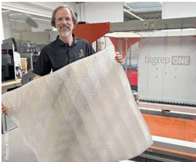
Thomas Lück is Head of Sales and Innovation, pictured here with PETG façade cladding elements from the large-format FDM printer Bigrep One, which can achieve a build volume of 1,000 x 1,000 x 1,000 mm.
