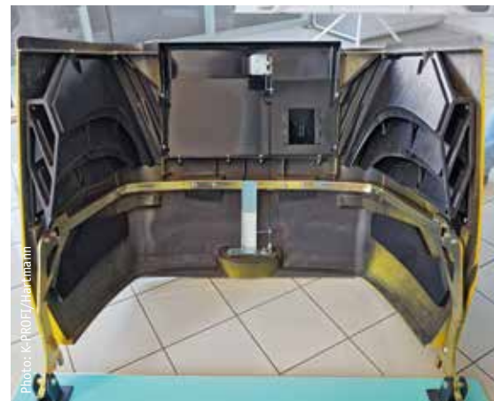
A look inside the wheel loader hood: Formtec foams core holes for subsequent thread inserts in the upper mould and thread bushings in the lower mould, as well as injection-moulded stud bolts for attaching the steel frame.
