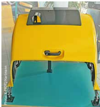
A typical PUR component is the hood for a wheel loader. The surface is painted.
