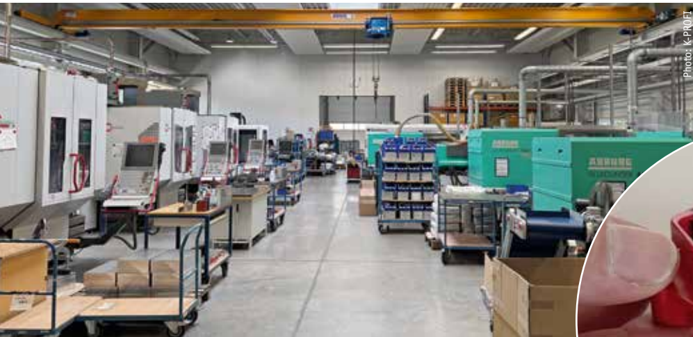
On the left, the “puzzle pieces” for the rapid tooling tools are being milled; on the right, seven injection moulding machines are ready for use. The largest, with a clamping force of 4,500 kN (rear right), is from Sumitomo (SHI) Demag.
