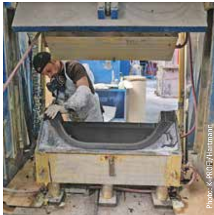
The worker manufactures fibre-reinforced PUR composite components on these special mould carriers. Currently, they are producing entry steps for the caravan industry.
