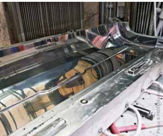
The PUR mould is polished to a high shine, as this is where rear upper parts for a caravan are produced using the in-mould coating process.
