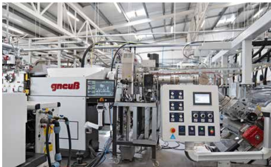
The combination of high degassing performance in the extruder and good filtration in the rotary screen changer means that even recycled material is no problem.
