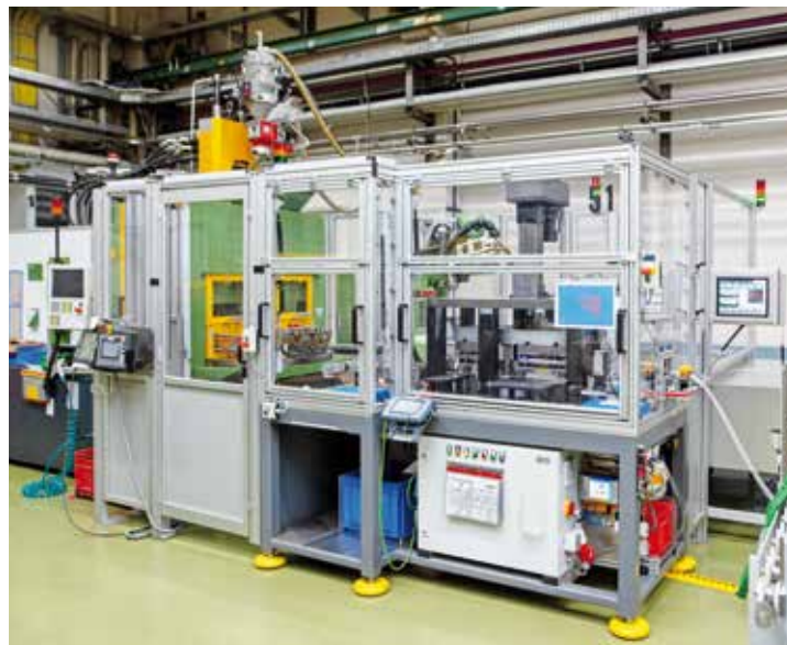
The production cell for overmoulding stamped and bent parts with a vertical machine was realised by Arburg and its partners.
