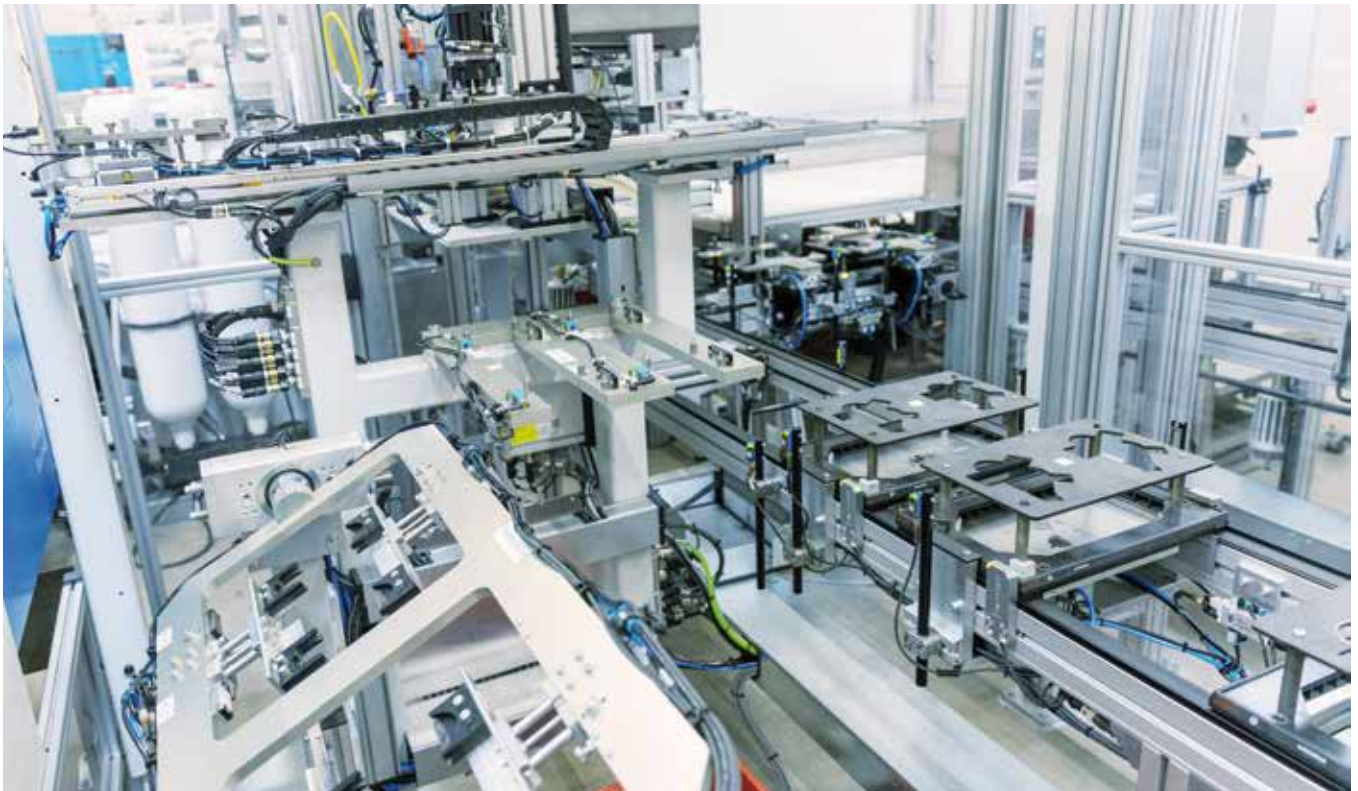
The fully automated laser welding system produces 600,000 oil suction tubes in variants with four different connections.
