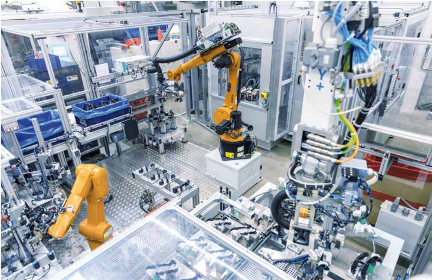
Injection moulding – hot gas welding – assembly – testing – packaging: Here, all process steps are coordinated and interlinked.
