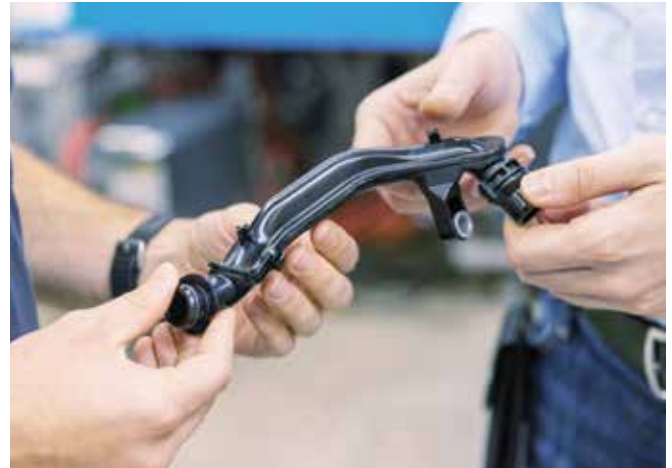
Hot-gas welding is often the first choice for tight radii and high demands on freedom from particles – as in the case of this coolant line.
