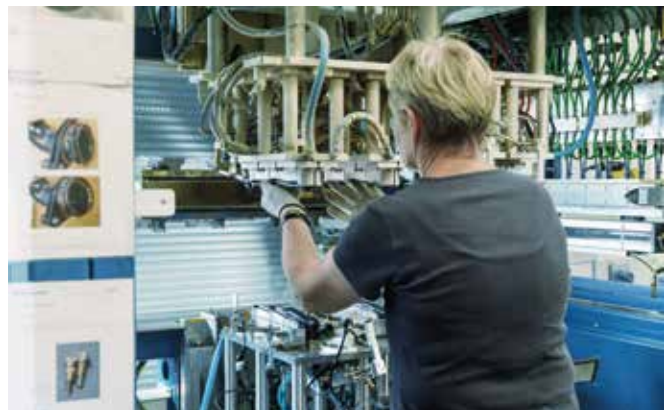
It can also be done manually: K-Tech also uses hot gas welding to produce up to 600,000 units of the individual workstations.
