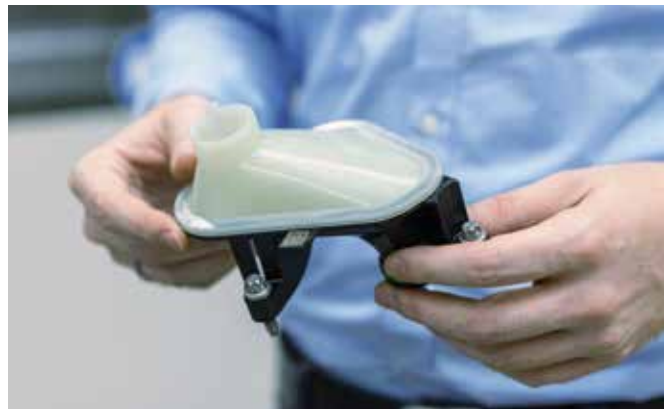
The top shell of the oil suction tube is made of laser-transparent polyamide. Both halves lie flat on top of each other and form a 2D contour.
