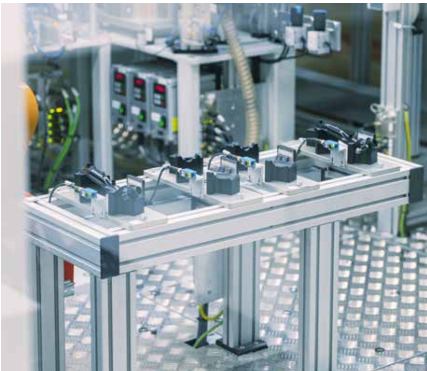
After hot-gas welding, before assembly: the coolant line lies in the intermediate tray.
