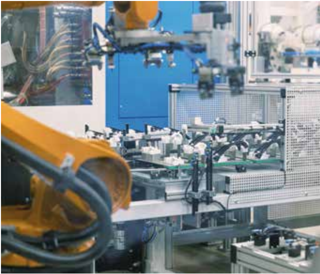
The two halves of the coolant line from the injection moulding machine are removed by a linear unit and placed on the transfer belt.
