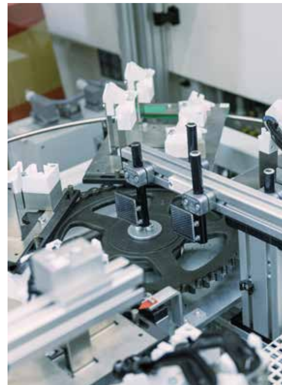
Always 2+2 halves are ready on the transfer belt.
