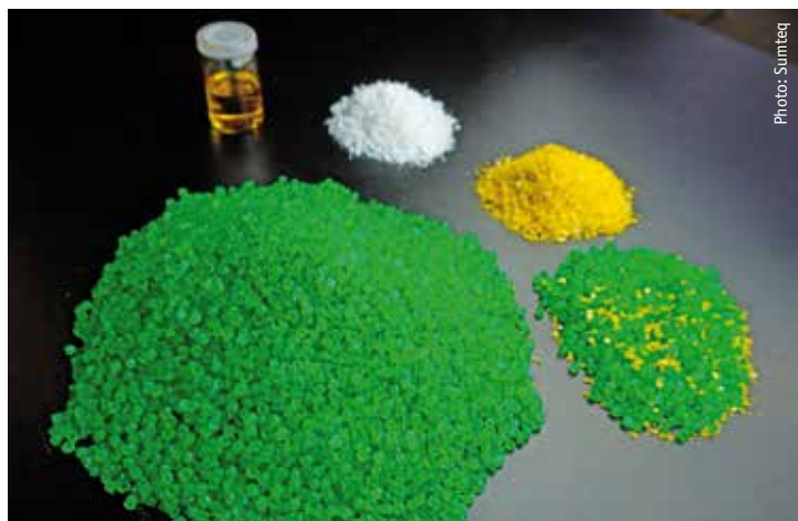
Substances from left to right: yellow-dyed plasticiser, Sumfoam flakes, Sumfoam with absorbed plasticiser, plasticiser-loaded Sumfoam plus waste PVC. In the foreground: PVC.
