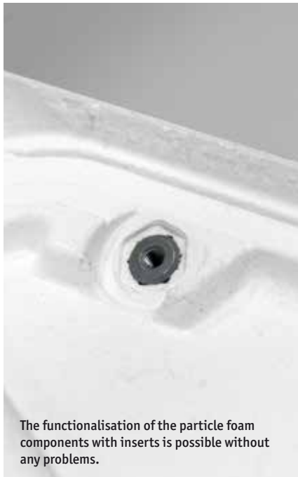
Reinforced with particle foam, the side part of the caravan bonnet is around 40% lighter than its LFI counterpart.
