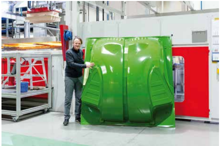
The mudguard of the enormous tractor in green for Fendt has dimensions of 1,870 x 670 mm.
