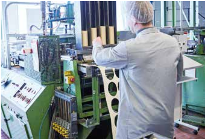
The “oldies” from the 1970s are still working reliably and are currently producing 2-chamber yoghurt cups made of PS.
