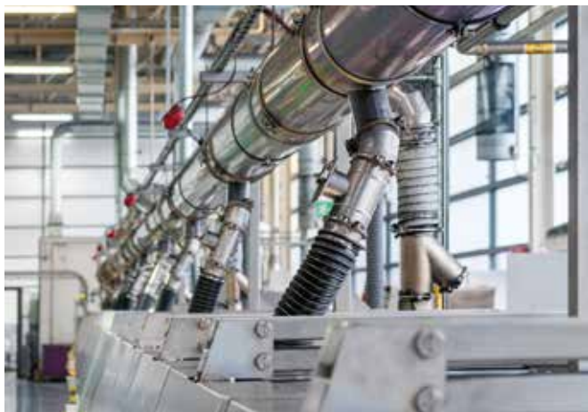
The exhaust air is extracted at several points above the salt bath vulcanisation system.
