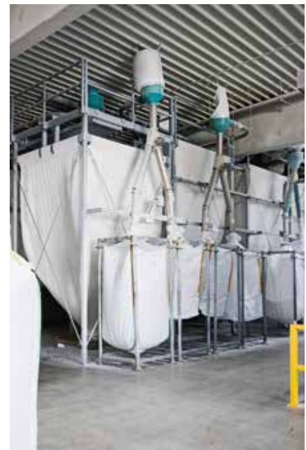
Eight sack silos are available for the regrind produced offline.
