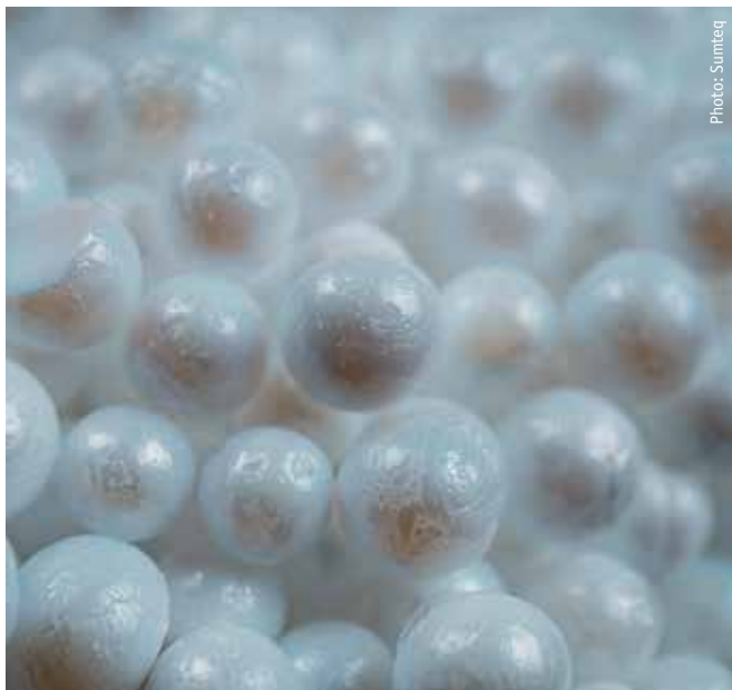
Originally foamed granulate with a grain size between 5 and 10 mm, it can be further ground into flakes or powder.
