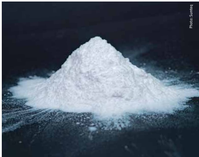
The finest form of Sumfoam. Even with the finest grinding down to 0.05 mm, each particle contains countless pores.
