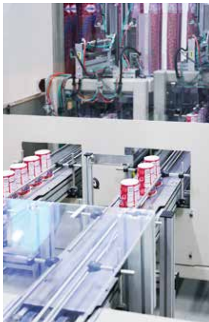
A Netstal machine produces 500 g yoghurt cups from PP on an 8-cavity mould.
