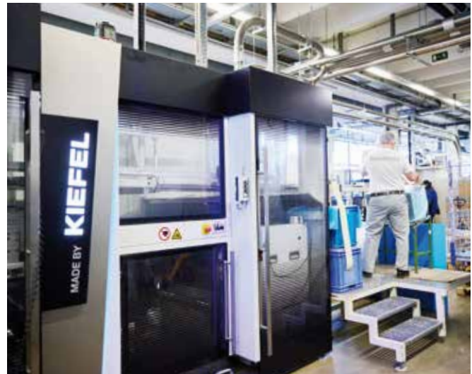
The lids are created on a KMD 78.2 Speed from a 360-µm PP film on a 10-cavity mould. The machine moulds and punches the lid in one station.
