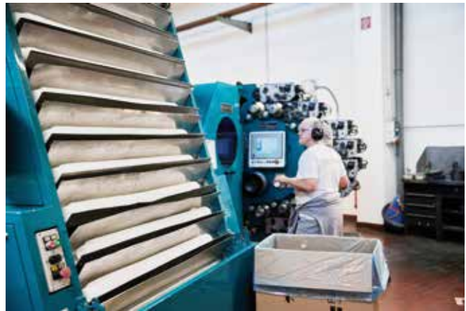
Dry offset printing provides logos, lettering and decoration. At 460 cycles per minute, the machine passes a lot of cups per day.
