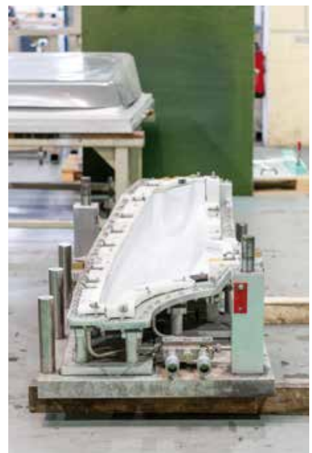
The concept of the temperature-controlled closed aluminium mould for particle foam technology was developed by Parat in-house and has also been patented.
