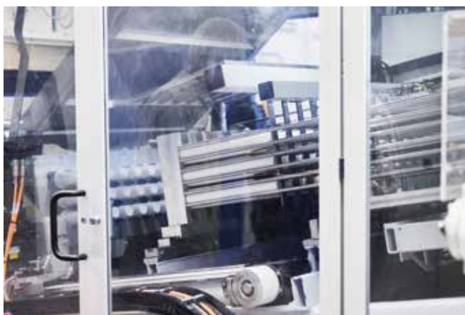
Many machines work with inline extrusion. PP film is produced here, which the RDM 73 K forms into cups on a 24-cavity mould.
