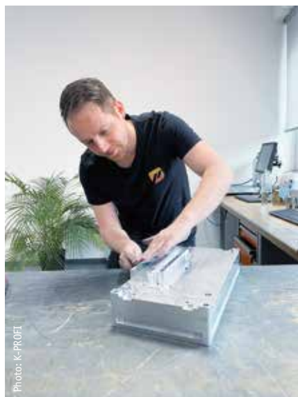
Manual work: Milled parts are assembled into the mould in the workshop.
