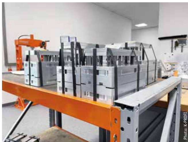
Complete mould kits: Priomold builds 500 new moulds a year, samples them and transfers them to the injection moulding machine.
