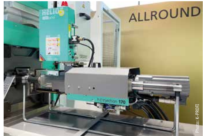
A hydraulic injection unit is robust and reduces the purchase costs of the Allrounder 470 H anniversary machine. Splitting the delivery flow of the hydraulic pump enables simultaneous driving of an additional auxiliary axle.
