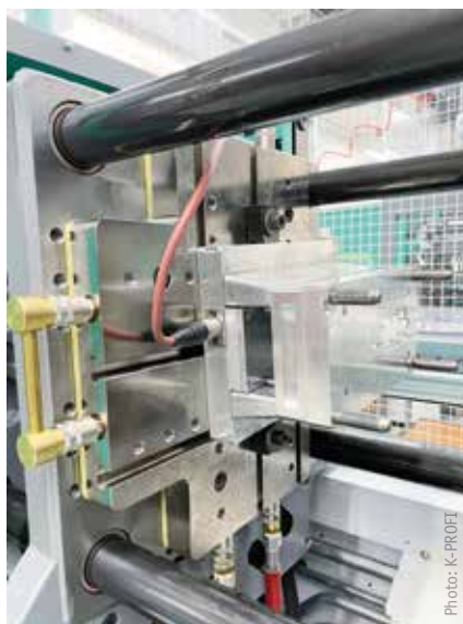
Priomold has developed its own master mould system with standardised mould plate sizes for its injection moulds. The temperature control system is housed in the master mould.
