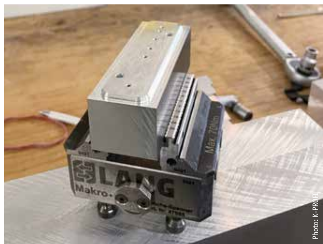
Prefabrication of blanks: Holes for ejectors, threads and fits for later screwing into the master mould are made before the contours are machined.
