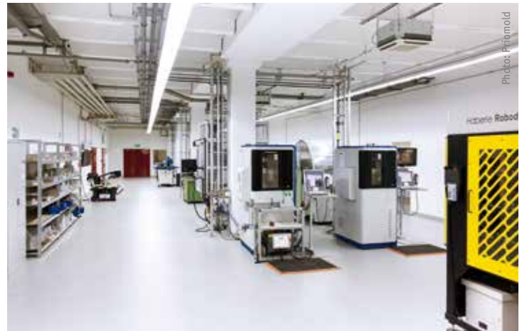
Instead of large machining centres: compact HSC milling machines produce high surface qualities with their fine cutting tools.
