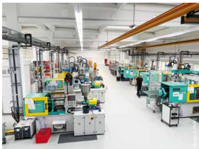
Priomold operates 17 injection moulding machines. The media lines are currently being laid for a further 20 injection moulding machines in the rear section of the hall.
