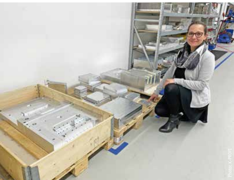
Ellen Wilhelm (Marketing) points to the standardised mould plate sizes and the high degree of prefabrication of the moulds made of high-strength aluminium.
