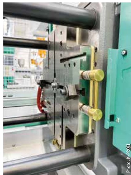
Priomold has developed its own master mould system with standardised mould plate sizes for its injection moulds. The temperature control system is housed in the master mould.
