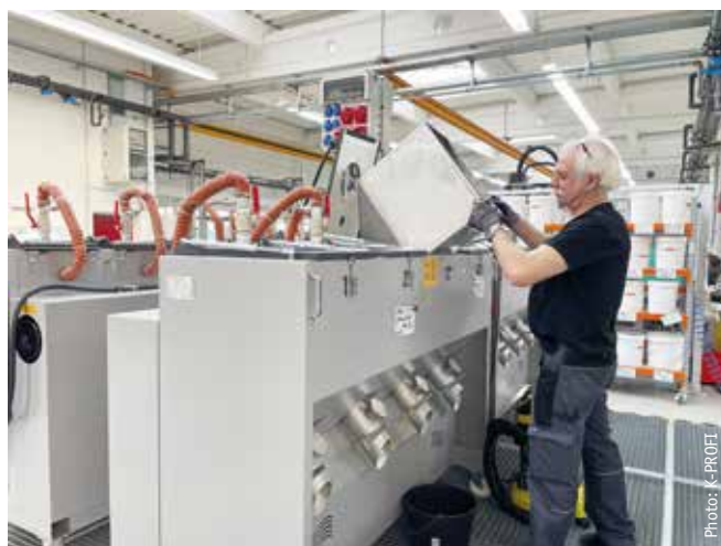
Separately temperature-controlled multi-chamber dryers from Gerco with small containers that can be hooked on offer a high degree of flexibility for the frequent changeovers.
