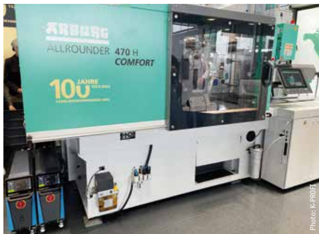
Pneumatics and central lubrication on the operator side as well as inwardly offset storage technology and hydraulic block open up more flexibility for options and peripherals at the rear of the anniversary machine.
