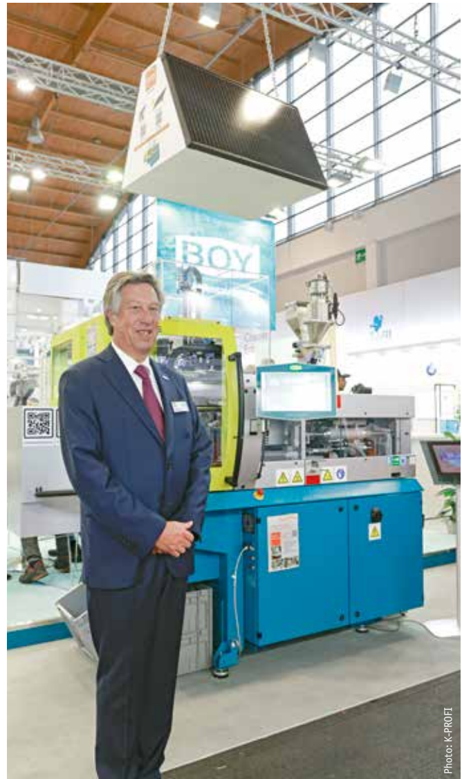
Managing Partner Alfred Schiffer sees the Boy 35 E, which is supplied via a DC grid, as a solution for saving energy.
