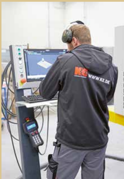
The worker starts the programme stored in the software for the counterpart of a rail guide ...
