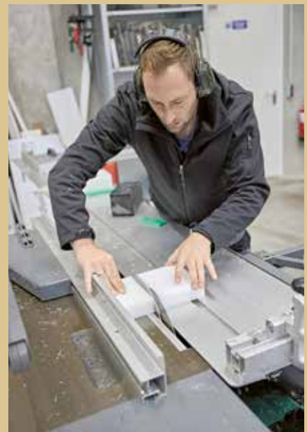
Here, an employee cuts the blank for the production of a spacer guard.
