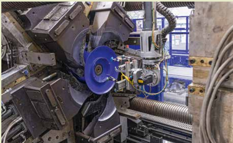
The 15,000 kN machine produces the impeller for centrifugal fans from the “ZAbbluefin” series with a diameter of 560 mm. The component is difficult to demould and works with numerous slides.
