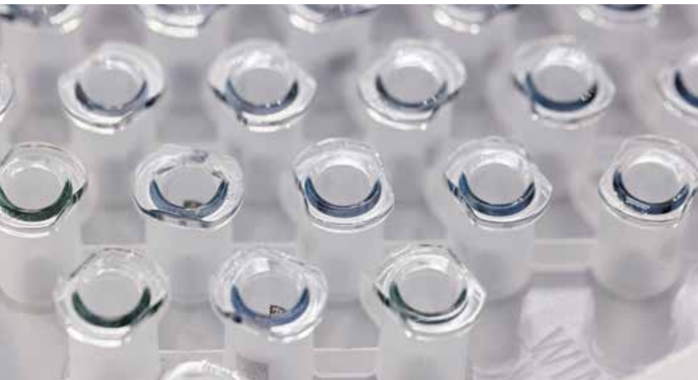
Crystal clear: During high-precision injection moulding, the syringe barrels made of transparent, specially additivated cyclo-olefin copolymer (COC) are 100% quality-controlled.
