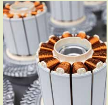
The vertical range of manufacture at Ziehl-Abegg is high: the motors are also produced in-house.
