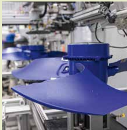
The blades are fitted into the impeller on the assembly line.
