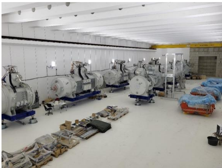
Figure 87: Sc-multiplets (on the left) and nc-dipoles halves (on the right) in the hall at the end of the low-energy branch.
