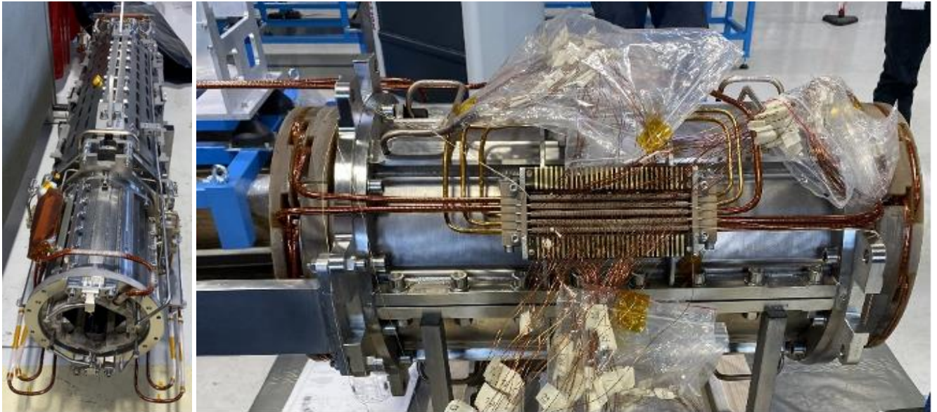
Figure 78: Left: prototype SIS100 quadrupole unit (left) and multipole corrector magnet. Right: manufactured in industry.
