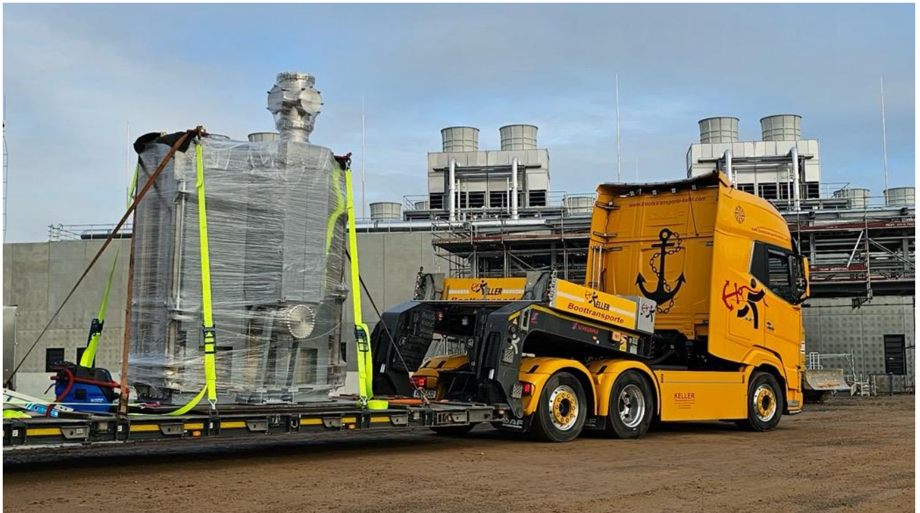
Figure 82: The Super-FRS target chamber, transported to FAIR.
