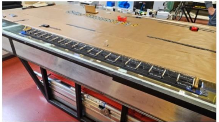
Figure 25: Left: Prototype air-cooling channel with air inputs/exits and flow return. Right: Fully assembled stave with two cooling channels on a carbon-fiber spaceframe.
