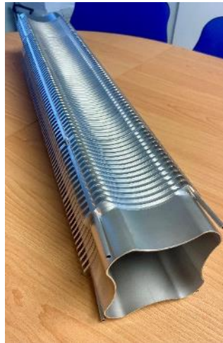
Figure 79: FOS star-shaped thin wall quadrupole chamber.
