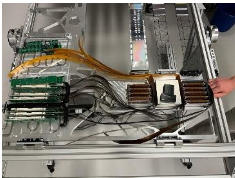
Figure 31: Prototype STS Half Unit on its Assembly Turntable.
