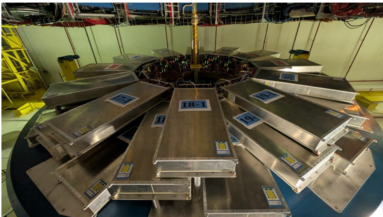
Figure 68: eTOF modules of STAR. Our electronics is located in the middle.
