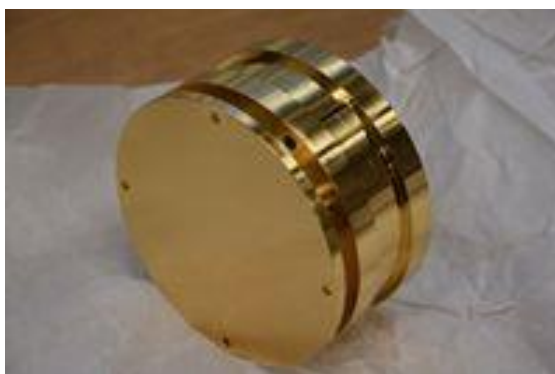
Figure 92: Gold-plated stopper block for SIS100 beam stopper
