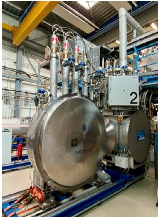
Figure 80: FOS current lead box at acceptance test at the GSI STF (Series Test Facility).
