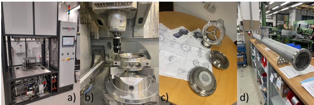
Figure 109: a) Inner part of the high-vacuum soldering oven, b-c) miniaturised accelerator structure during and after post-processing, d) beam pipe for connection between GSI and FAIR high energy beam transport.
