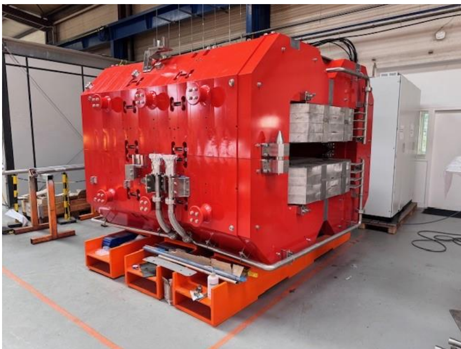
Figure 84: A normal conducting dipole.
