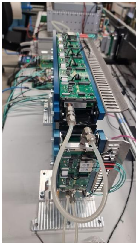
Figure 67: 6 SCIFI modules are chained for one SCIFI-detector.
