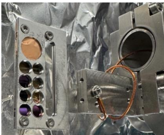
Figure 105: The sample ladder for the G0057 experiment at HITRAP.
