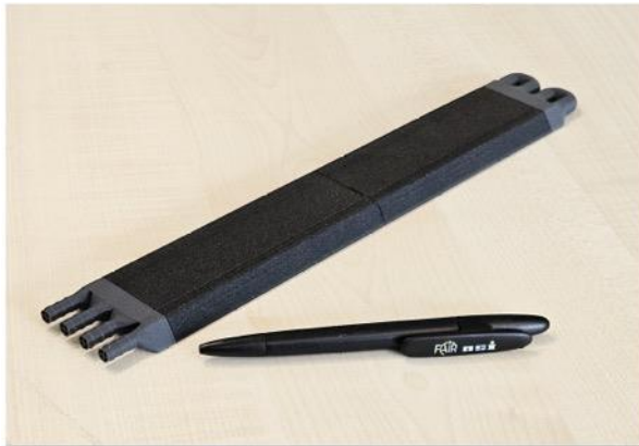
Figure 25: Left: Prototype air-cooling channel with air inputs/exits and flow return. Right: Fully assembled stave with two cooling channels on a carbon-fiber spaceframe.
