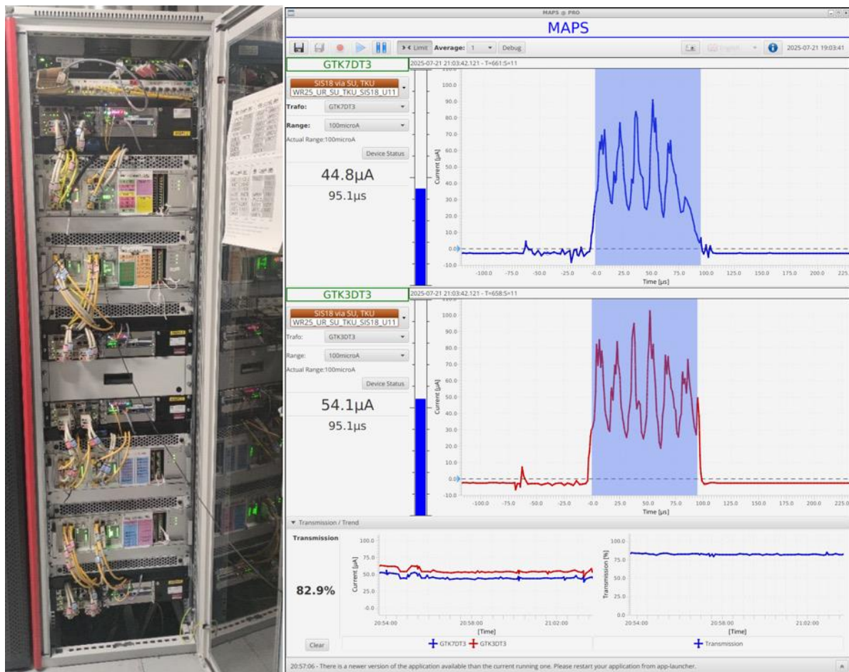
Figure 90: Electronic rack with MAPS data acquisition hardware (left) and MAPS graphical user interface (right).
