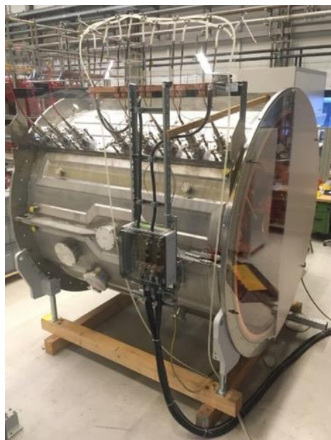
Figure 113: Cavity section Alla-1 equipped with the electrical supply system to be tested at the GSI Testing Hall (TES).
