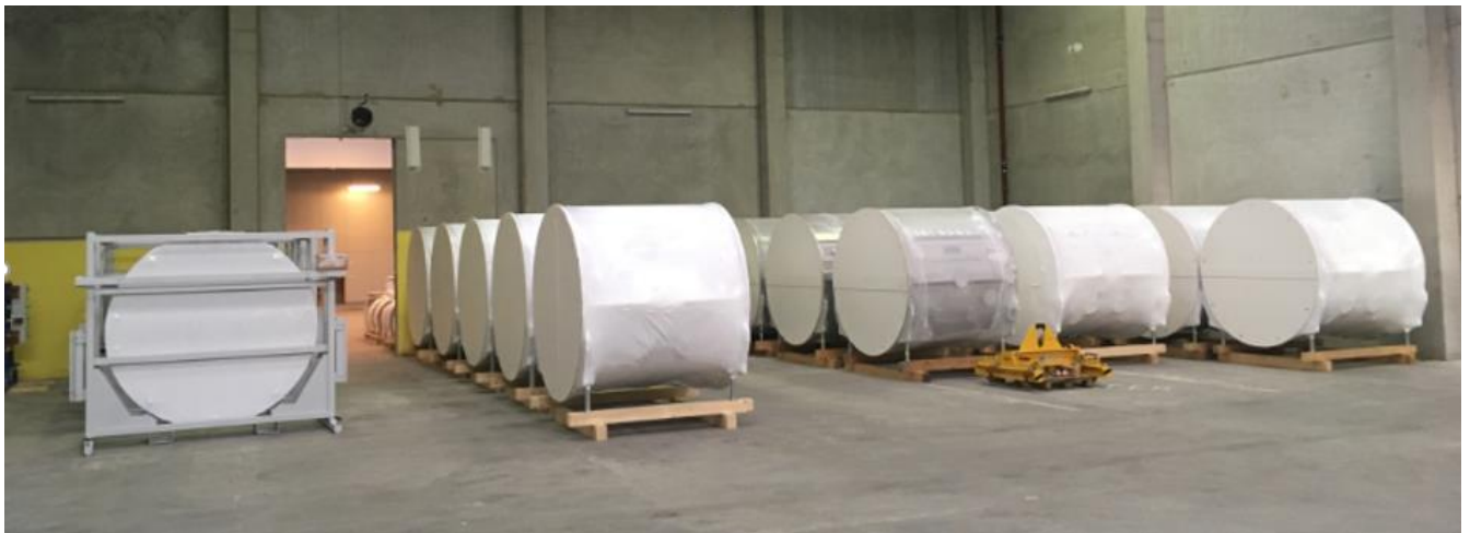
Figure 111: External storage area in Pfungstadt for the large-scale components – cavity sections and end plates.
