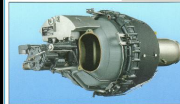
The turbojet engine KHD T 117 is installed in the reconnaissance drone CL 289
