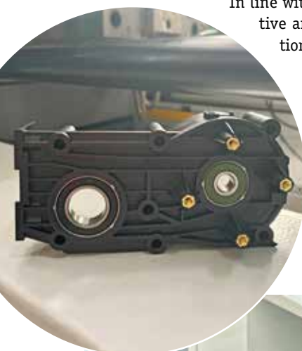
Two ball bearings plus six screw and threaded bushings are inserted manually and overmoulded for this housing. The metering pump gearbox is completed at the assembly plant in Poland.
