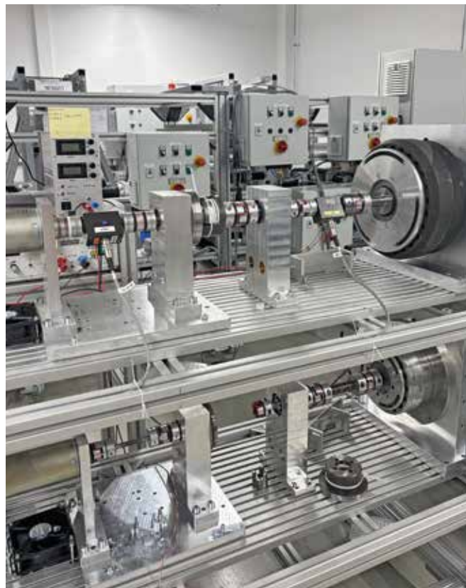
On this test bench, various plastic combinations of a new planetary gear design are tested for service life and performance, for example, how unfilled and filled materials behave when in contact with each other.
