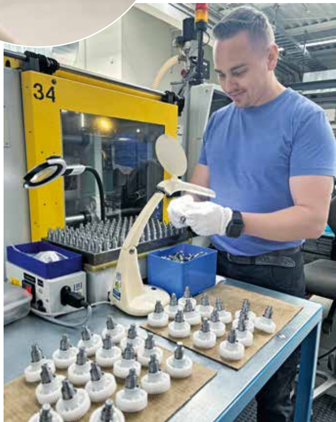
The small quantities do not justify automation here: the metal shaft is heated before manual insertion. After overmoulding, the components are visually inspected.
