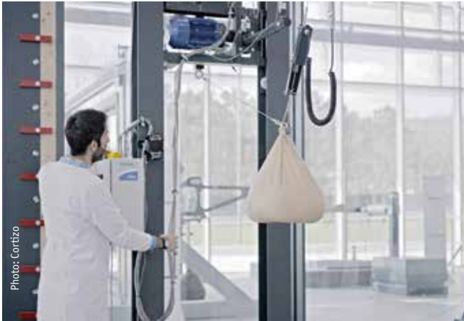
The windows undergo numerous tests. This involves mechanical parameters such as bending modulus, breakage test and impact resistance.
