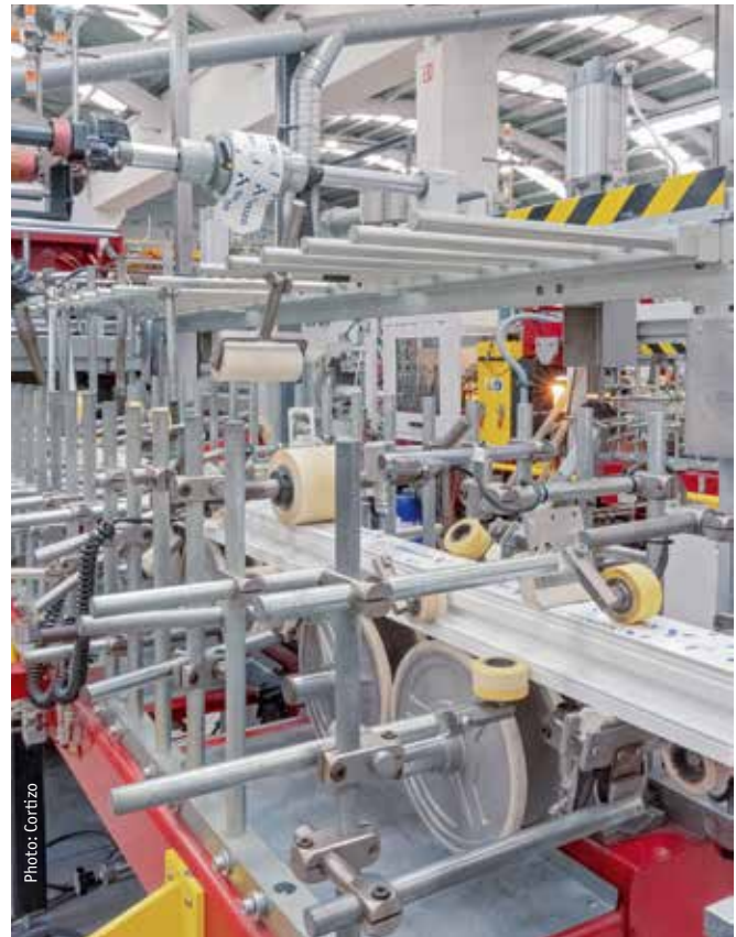
Nine laminating systems apply the films to the profiles.
