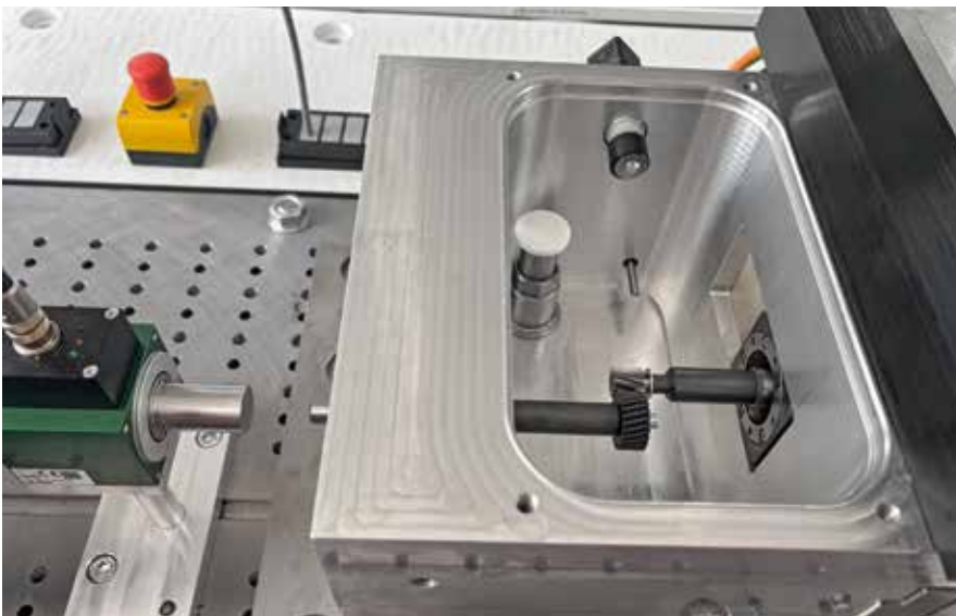
The gear test bench was developed in-house to determine the characteristic values of various plastics required for gear design.
