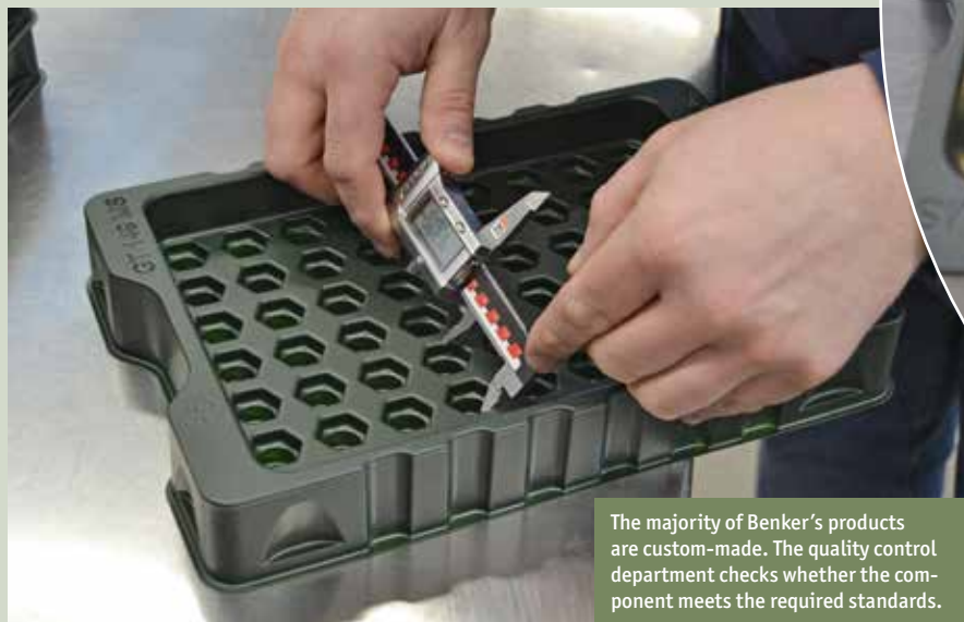
The transport packaging for the compressed air nipples weighs just 60 g itself but can easily handle the entire 1,200 g load. Up to ten of the trays can be stacked on top of each other.
