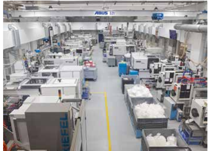
In several clean rooms, 70 injection moulding machines are in operation with automated moulded part removal and integrated test routines.
