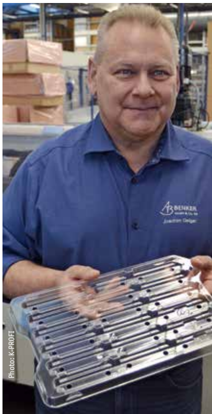
"We do not punch the holes in the bottom of these trays on the thermoforming machine during operation because the trays could get stuck at high production speeds," explains Joachim Geiger.
