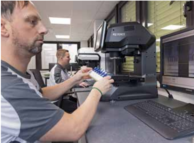
The precision and quality of the mass-produced goods is not only checked visually on the injection moulding machine, but also in the laboratory, by touch and by computer tomography.
