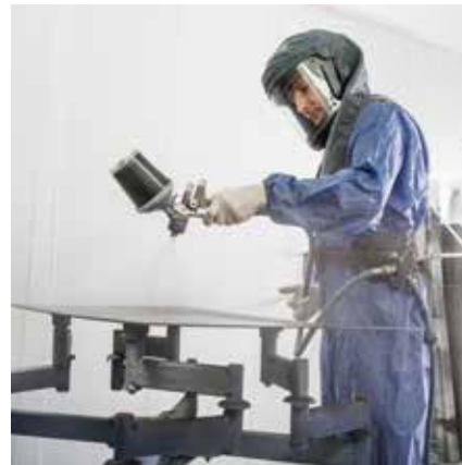
Pre-formed components are given the desired colour design in the paint booth.
