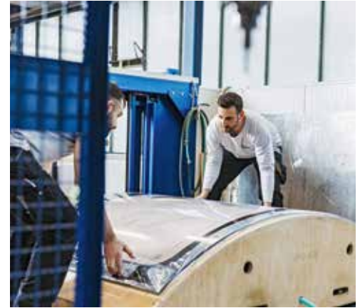
Two employees remove a finished milled component from the workpiece holder of the CNC machining centre.
