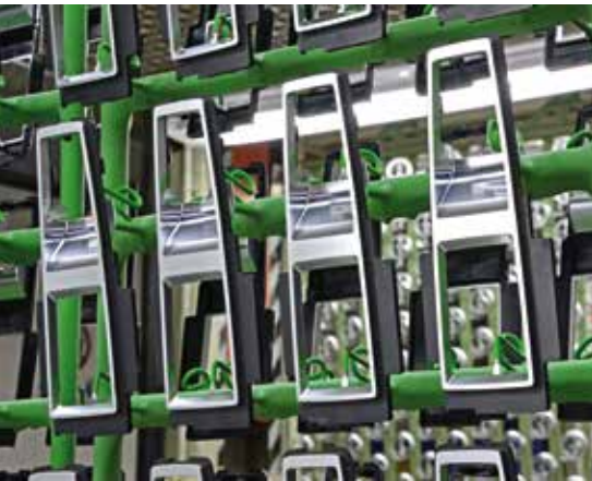
For chrome plating, the parts are mounted on support frames.
