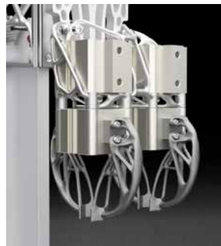
Compared to the previous aluminium milled component (left) weighing 0.33 kg, the plastic gripper additively manufactured using SLS weighs only 0.05 kg (one of the four components in each case).
