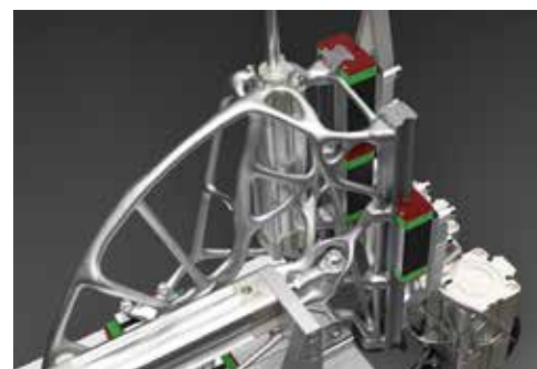
The moving axes of the pick-and-place unit before (top) and after the topology optimisation, which reduces the weight by 29.8 kg and combines eleven components into four.
