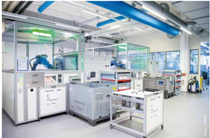
The fully automated production cells with Yaskawa six-axis robots are designed to work also in ghost shifts.
