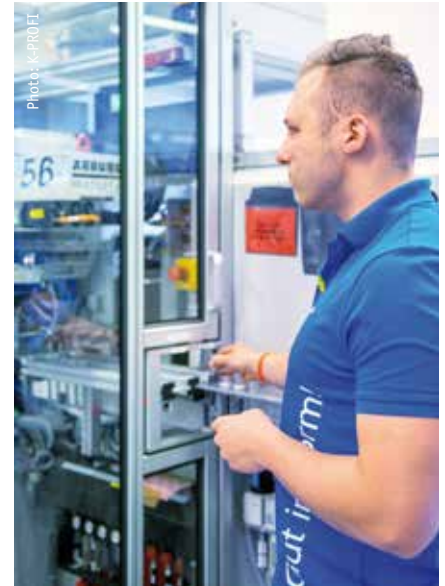
Process Manager Lucas Heuchele at the micro injection moulding machine from Arburg, which is used for smaller series when high-cavity moulds are not profitable
