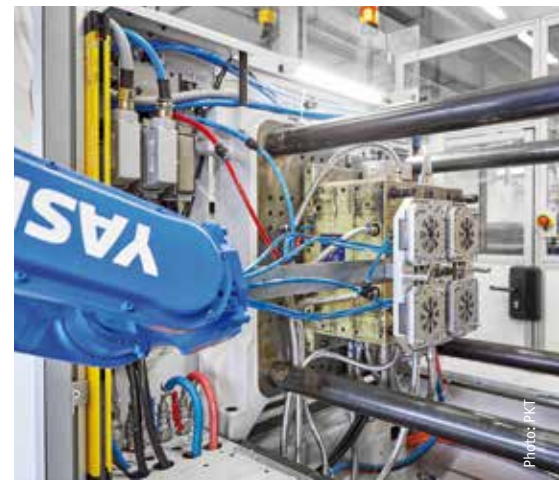
Six-axis robot with gripper plate for removing micro-injection moulded parts from the high-cavity mould.
