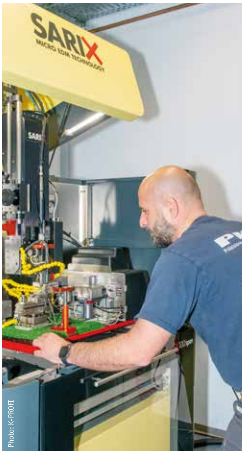
Rarity: This high-precision micro EDM machine from Sarix enables repeat accuracies below 1 µm and surface finishing with Ra values below 0.1 µm.
