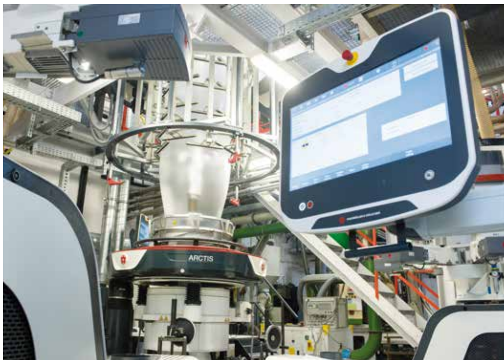
Depending on the product, the film specialist operates its PE blown film lines in short-neck (photo) or long-neck mode.
