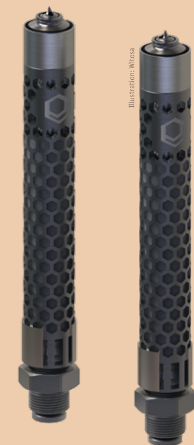
The 3D-printed Monolith nozzles are available with take-off bodies of 16, 20, 22 or 24 mm diameter (and fixed flow channel diameters of 4, 5, 6 or 8 mm respectively). A 28-mm variant with a 10-mm flow channel will be launched before the end of 2021.
