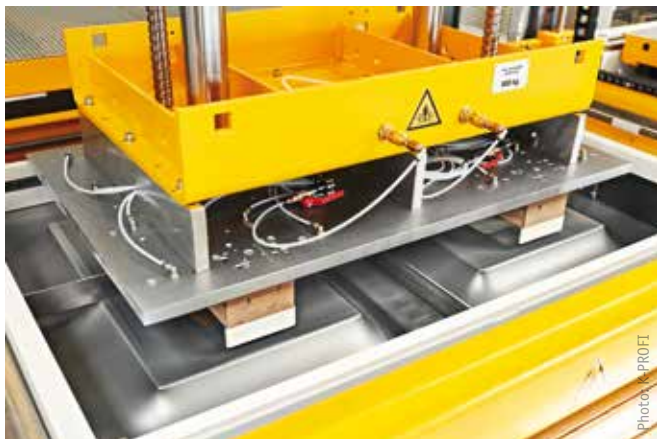
The ABS/PMMA semi-finished product is heated, and the mould moves into the mould.
