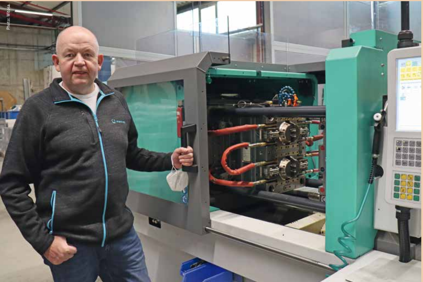
Manfred Göke from Industrial Engineering at Oventrop tested the 3D-printed nozzle on an electric injection moulding machine.
