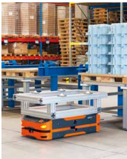
To pick up the pallets in the station, the driverless transport system raises its loading platform by a few centimetres; to set it down, it lowers it. Wirthwein built the pick-up devices itself.
