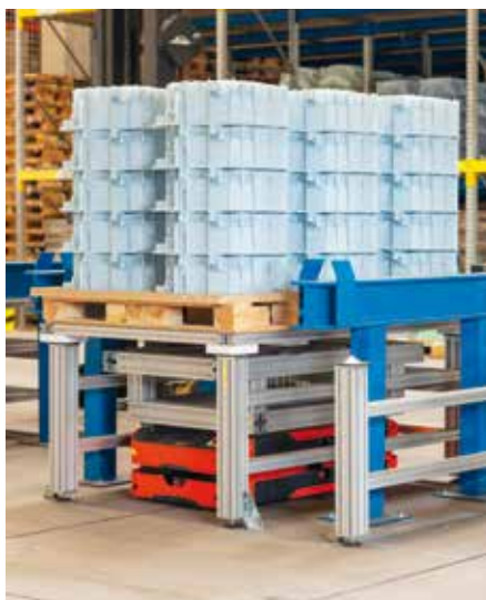
To pick up the pallets in the station, the driverless transport system raises its loading platform by a few centimetres; to set it down, it lowers it. Wirthwein built the pick-up devices itself.
