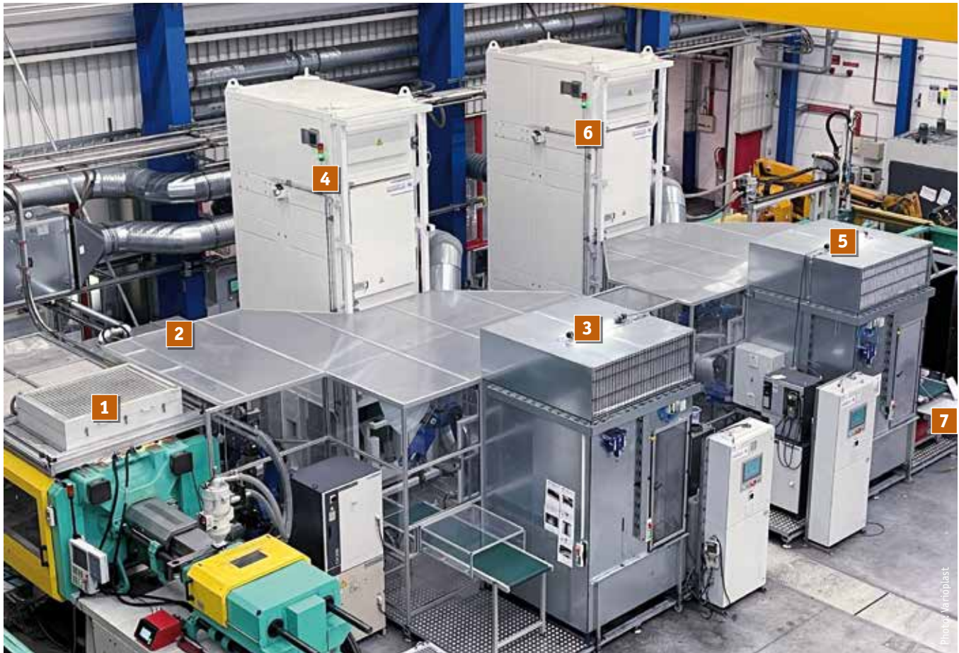
Inline linking of all process steps via six articulated-arm robots, among others: 1 injection moulding, 2 CO 2 pre-cleaning, 3 priming, 4 drying, 5 effect painting, 6 drying, 7 visual inspection by workers.
