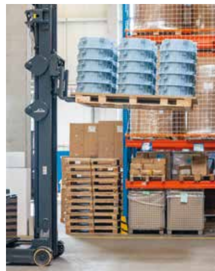
To lift the 204 x 120 cm special pallets into the buffer store, the tines of the forklifts were extended by 70 cm.
