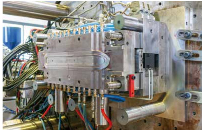
Cascaded sandwich injection moulding allows a continuous core and edge layer to be produced without partial interruption.
