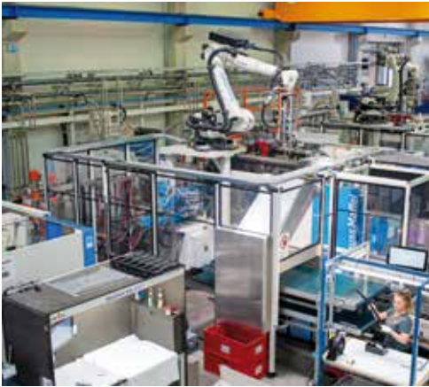
Production cell for the decorative strip: 2C injection moulding machine GXL 651-3000/750 with rotary table and six-axis robot for film and part handling.
