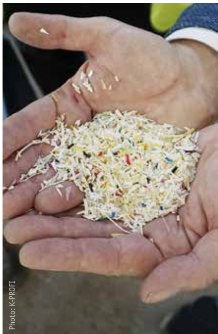
High-quality flake fractions from only one raw material and with as uniform a colour as possible are the result of the pilot plant.
