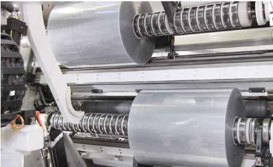
Five slitters implement the customer's specification in the slitting centre and produce the desired end products or reels.
