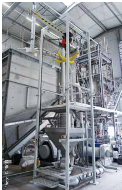
In what is currently the last process step, in the superclean plant, adhering odours are removed from the flake fractions.
