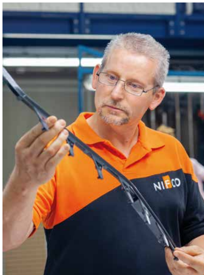
Joachim Schinke, head of the injection moulding department, inspects the 2K/IML decorative strip, which is challenging in terms of gap dimensions and surface.
