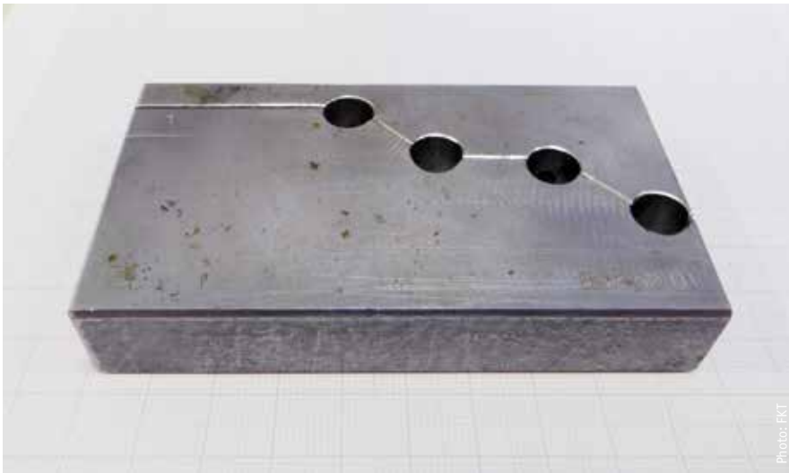
Diffusion-welded insert made of two parts with cooling holes and angled shoulders in the joining zone (top: underside), on whose mirror-smooth surface (bottom) the joining seam is not visible.
