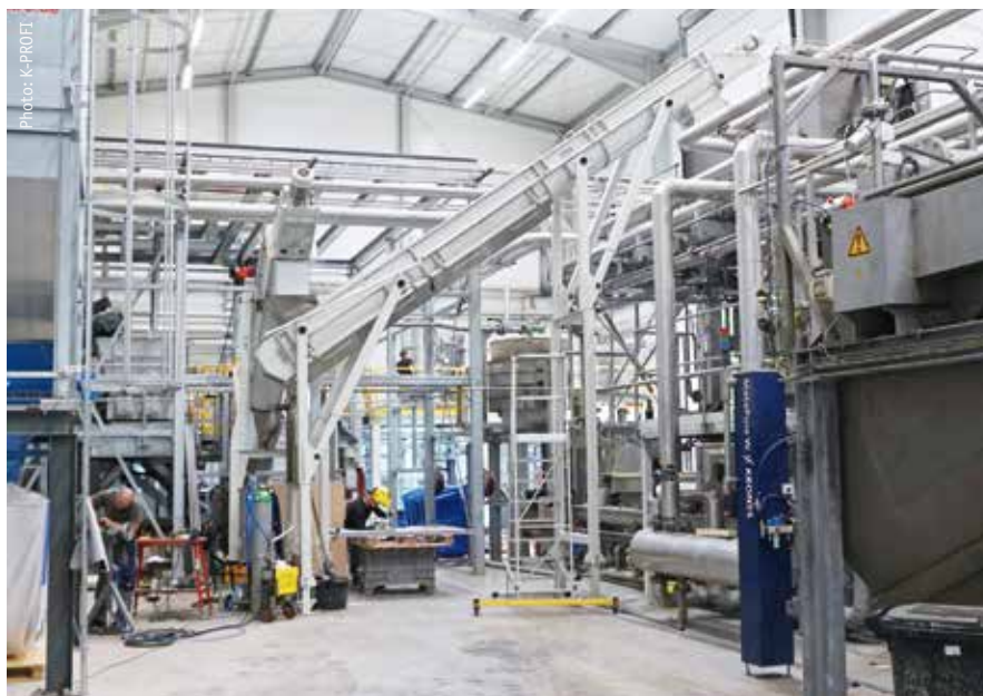
The preparation process begins after pre-sorting in the washing plant, which consists of pre-washing and main washing.
