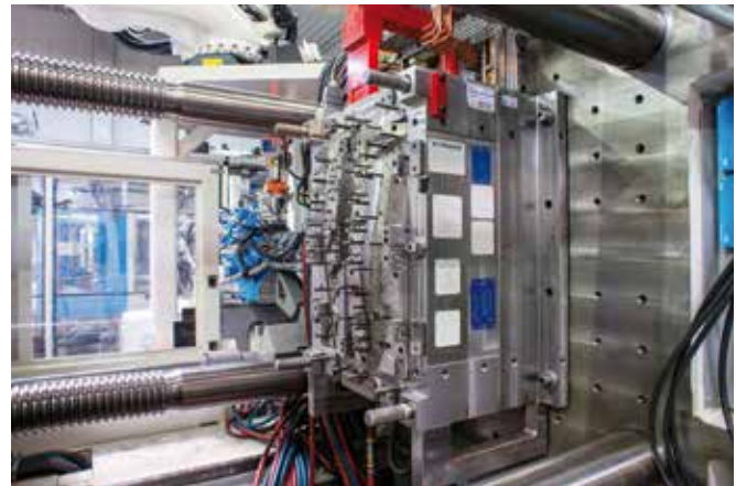
Injection-side mould half of the 2C decor strip with insert-holding slides for holding the preformed decor foil.
