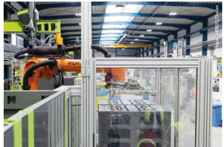
Production at Formex: each pallet is given an individual label, checked and stacked outside the machine.
