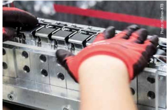
Button sets for the centre console of passenger cars are assembled fully automatically in Marktoberdorf.
