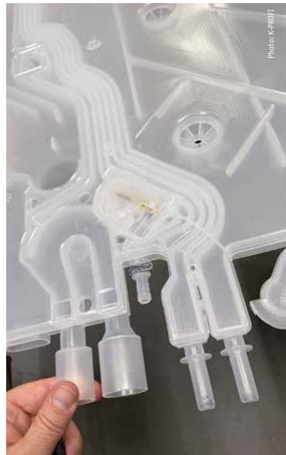
The 2+2-cavity stack mould runs with an effective clamping force of 9,500 kN on a 15,000 kN injection moulding machine from Engel, the largest of a total of 21 injection moulding machines at BSH in Dillingen.
