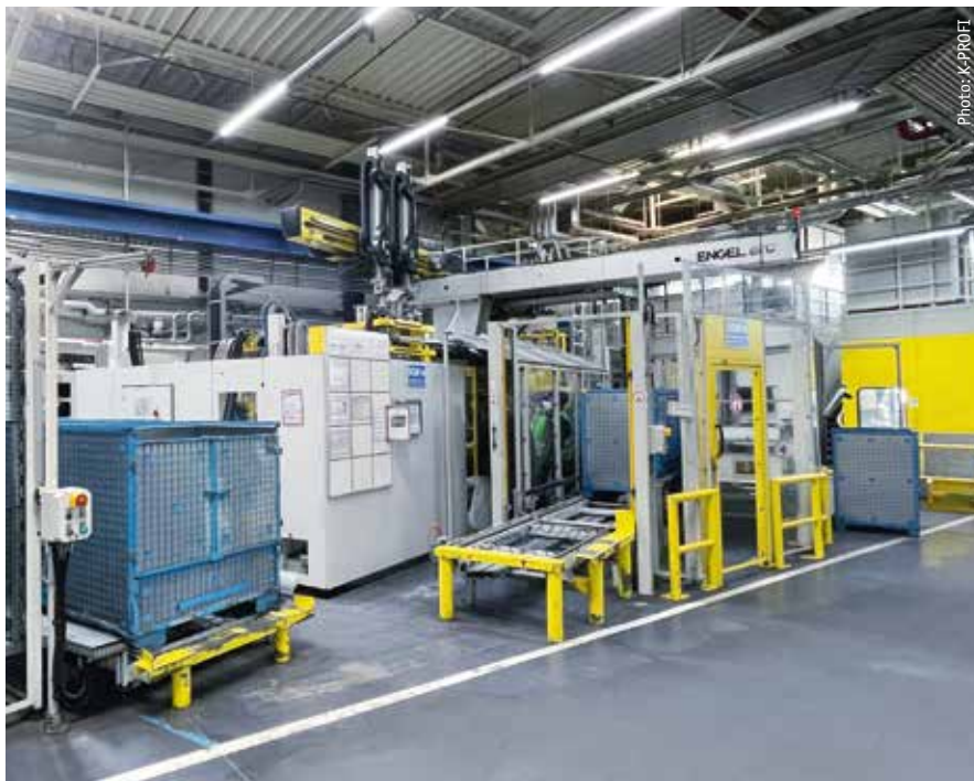
The 2+2-cavity stack mould runs with an effective clamping force of 9,500 kN on a 15,000 kN injection moulding machine from Engel, the largest of a total of 21 injection moulding machines at BSH in Dillingen.
