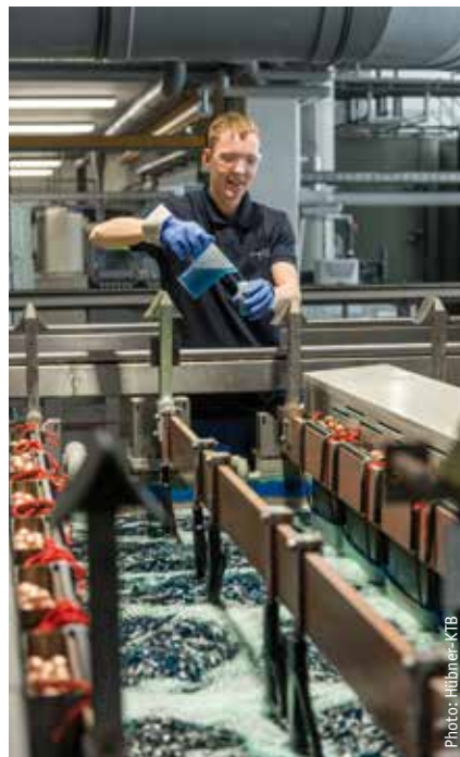
One of the two lines in Kaufbeuren (photo) as well as the one in Marktoberdorf are already equipped with modern chrome(III) baths.
