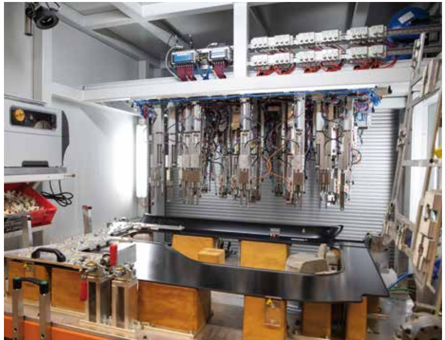
Above left: Here, too, a folding frame ejects the interior trim from the machine so that the employee can remove it easily.
