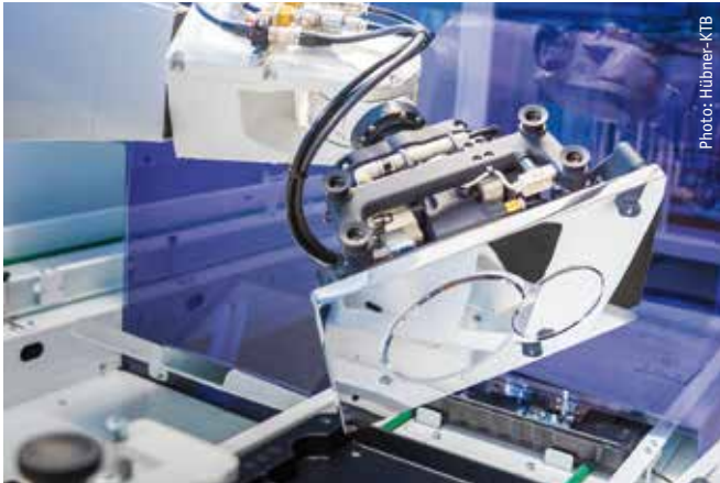
The fully automated camera-based surface inspection of high-gloss chrome parts is an important step in quality assurance.
