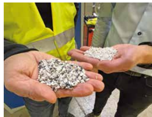
Output streams from the recycling plant are a white fraction, which can be fed directly back into the profile extrusion process, and a coloured fraction, which is first regranulated.
