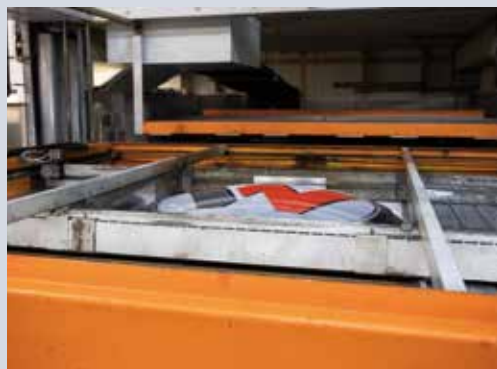
Above: Slow and controlled heating before the forming process is indispensable to avoid damaging the print.
