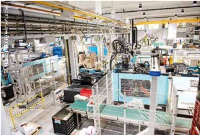
In Kaufbeuren, 25 machines up to 6,500 kN mainly inject automotive parts. The 1K machines are gradually being converted to fully electric models.
