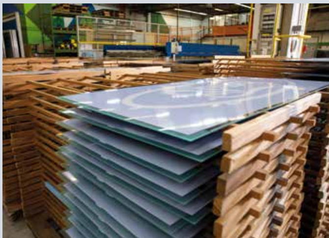
After the printing process, the semi-finished products must dry completely before going to the thermoforming department.
