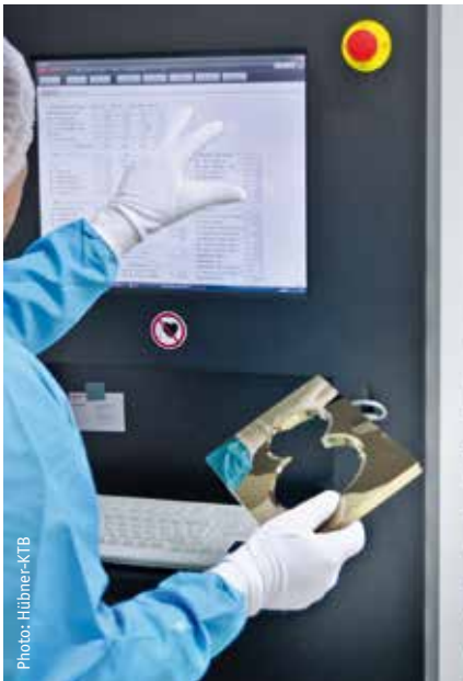
Photo: Hübner-KTB With PVD, Hübner-KTB achieves colour variations of chrome actuator plates for dual-flush toilets ...
