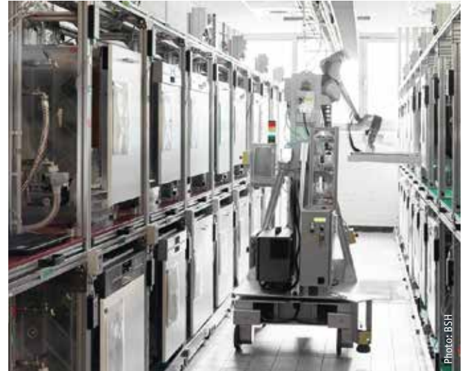
In continuous operation: During the extensive quality tests, a dishwasher runs around 3,500 times – which corresponds to a service life of twelve and a half years.
