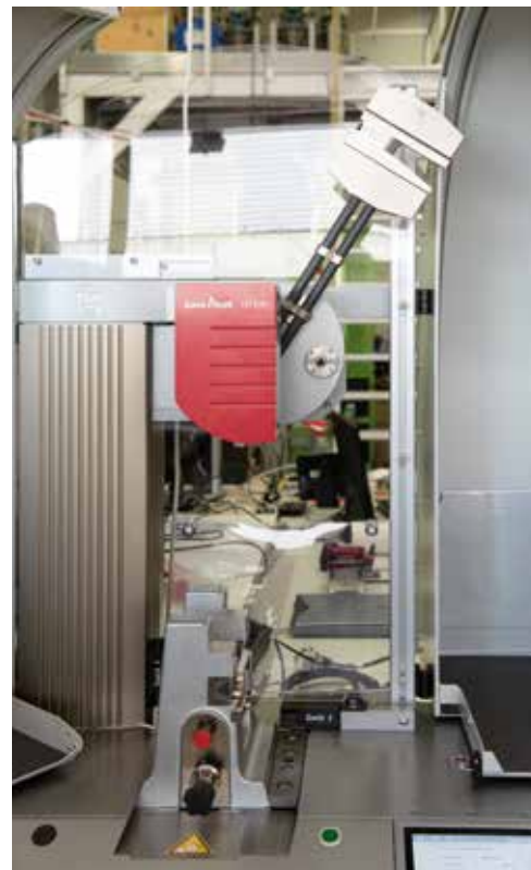
During K-PROFI's visit to Kaufbeuren, a new notched bar impact testing machine from Zwick-Roell is being commissioned.
