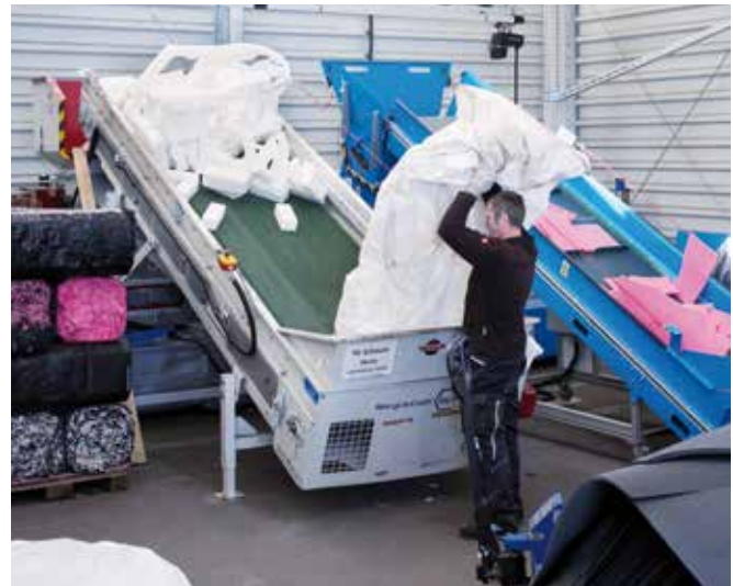
The conveyor belt takes the production waste to the shredder and then to the compactor.
