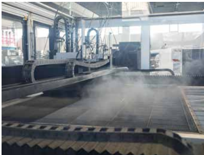
For internal contours, waterjet cutting is still the method of choice.
