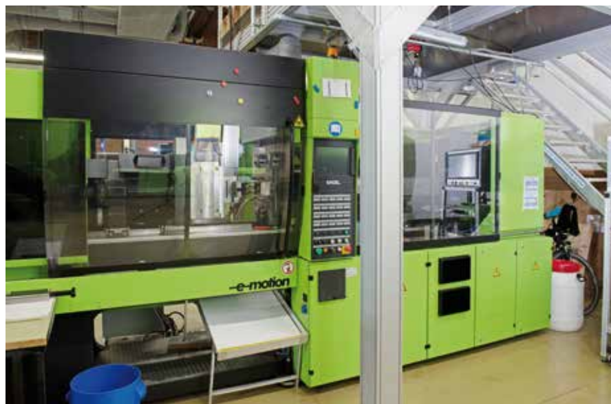
Two fully electric 2K injection moulding machines from Engel produce test specimens for the computer-defined batches.
