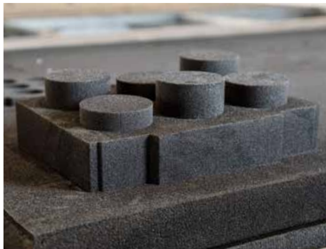
The result of waterjet cutting: packaging for containers in the chemical industry.
