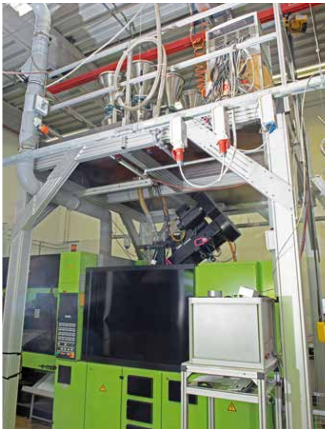
All injection units of the machines are supplied via gravimetric direct metering carousels for up to eight raw materials each.
