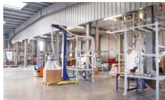
Finally, the cleaned granulate slides down to the ground floor where, after metal separation, it is filled into the container requested by the customer.
