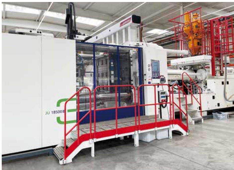
The 18,500 kN machine from Haitian's Jupiter series marks the upper clamping force limit of the machine park, which starts at 200 kN.
