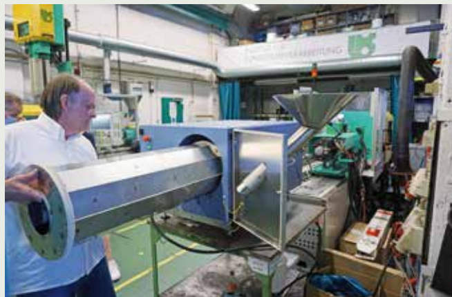
Thanks to its lightweight construction, the drying unit is quickly ready for use again: simply remove the rotary tube from the housing and replace or clean it.
