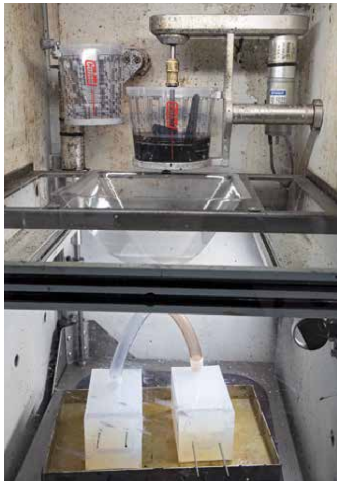
Light trap manufactured by vacuum casting. The tolerances in vacuum casting are largely comparable to those in injection moulding.
