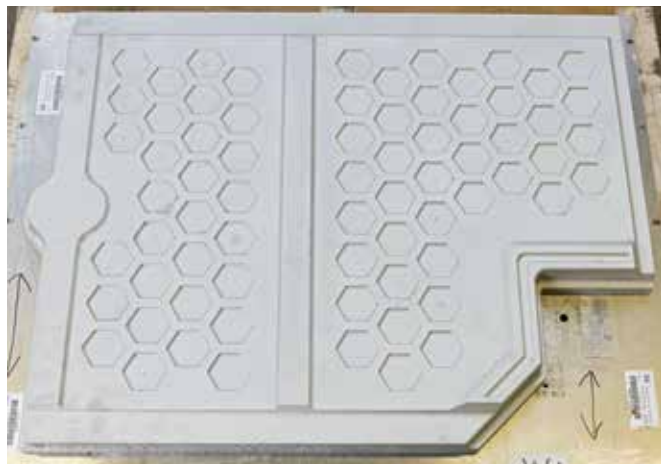
The underbody panelling for a construction machine is created using this mould.
