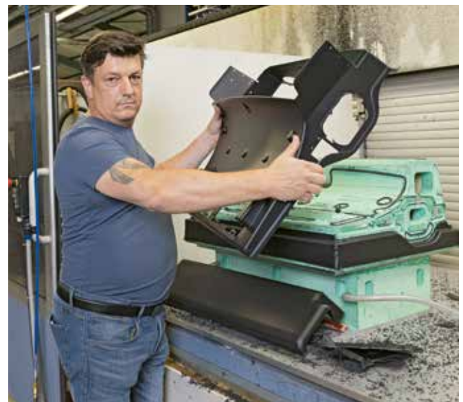
After CNC processing: Uwe Schupp removes the milled component – part of an air duct – from the clamping device.
