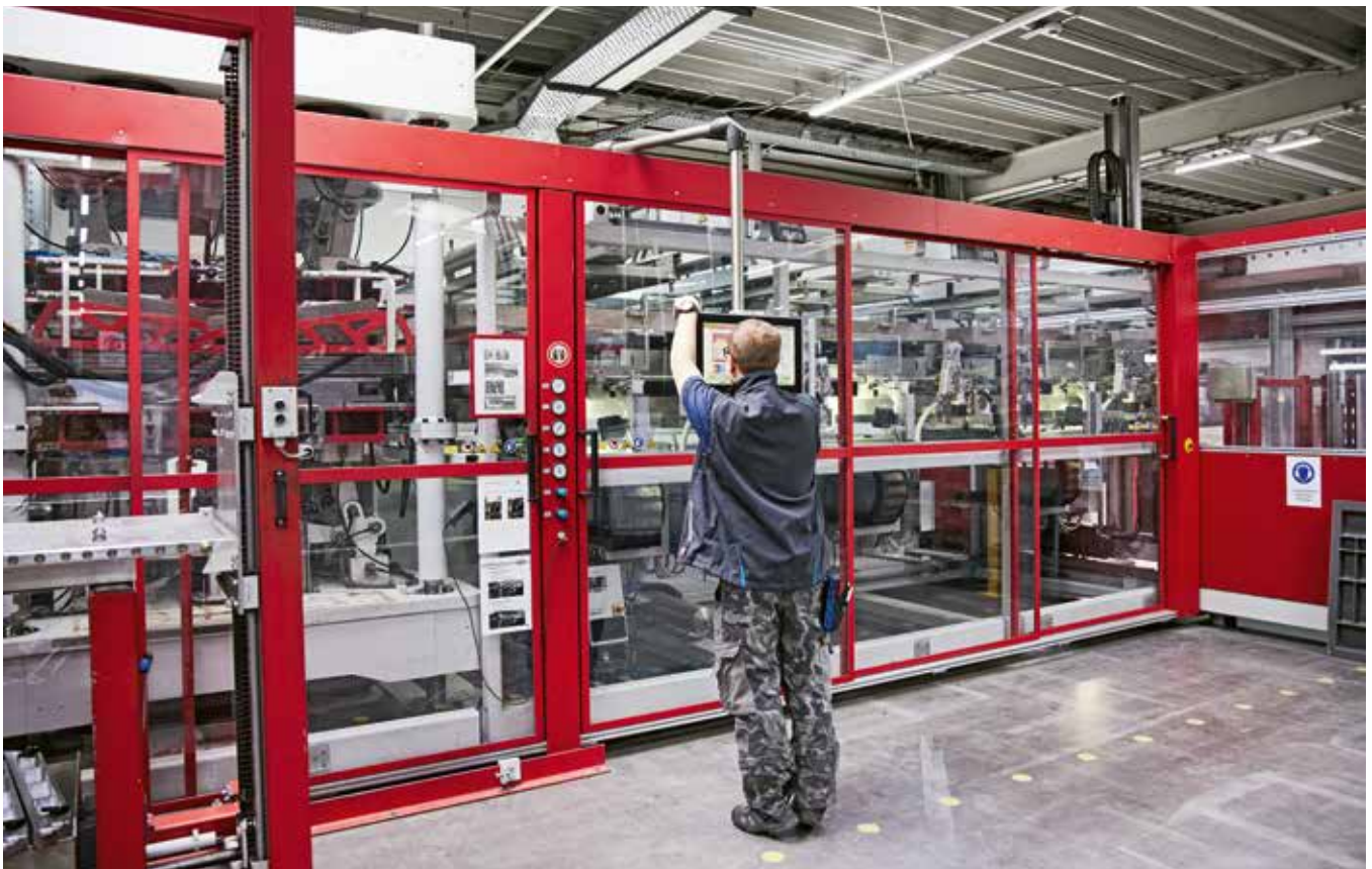
High-speed machines process both roll and sheet material into product carriers and drawer inserts.
