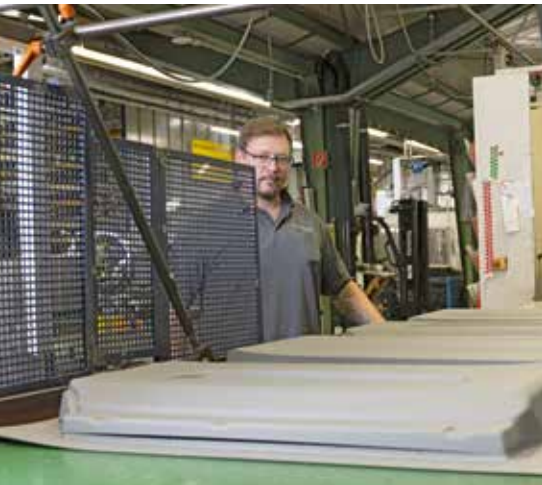
The horizontal band saw on the large Illig UA 250 4G is also controlled by the machine. Here, ABS door panelling is being cut from the clamping edge.
