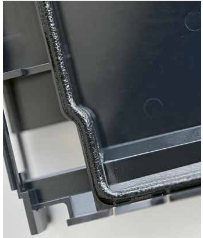
View into the housing of the mainboard before (left) – and after (right) – the sealant is applied. The seal is firmly bonded to the PC housing material.
