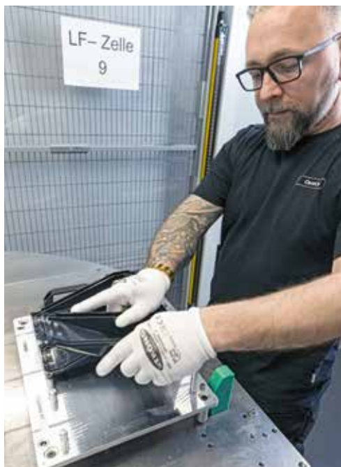
The rotary indexing table is fitted with three housings per run.
