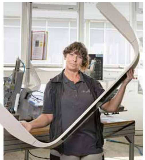
Top: The fully assembled dashboard panelling consists of three elements.
