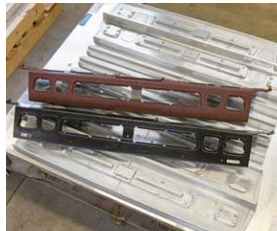
Storage floor laminated with leather (red) and unlaminated (black), plus the 4-cavity mould for thermoforming.
