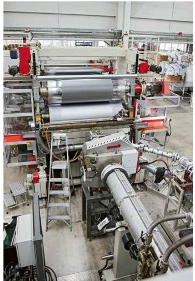
View from above of the extruder with mould and cooling section.
