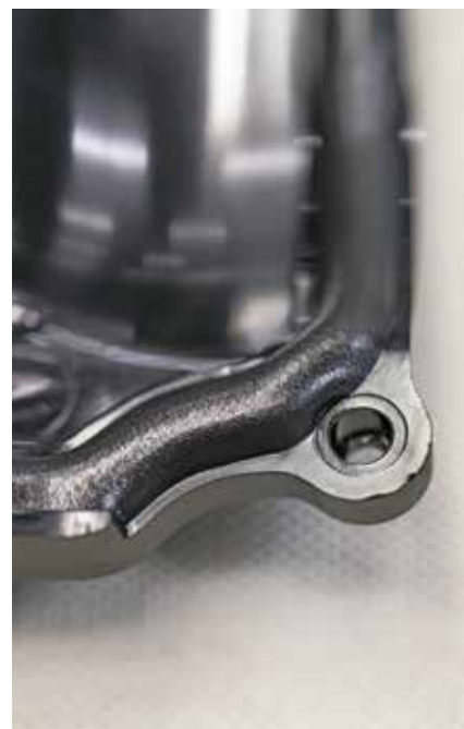
The housing of the frequency converter before foam application (left) and afterwards (right). The seal fits snugly around the edge of the housing.
