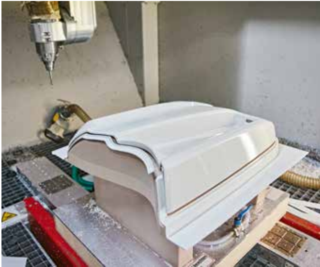
The company uses a tempered 1+1 mould made of ABS/PMMA to produce the light supports.
