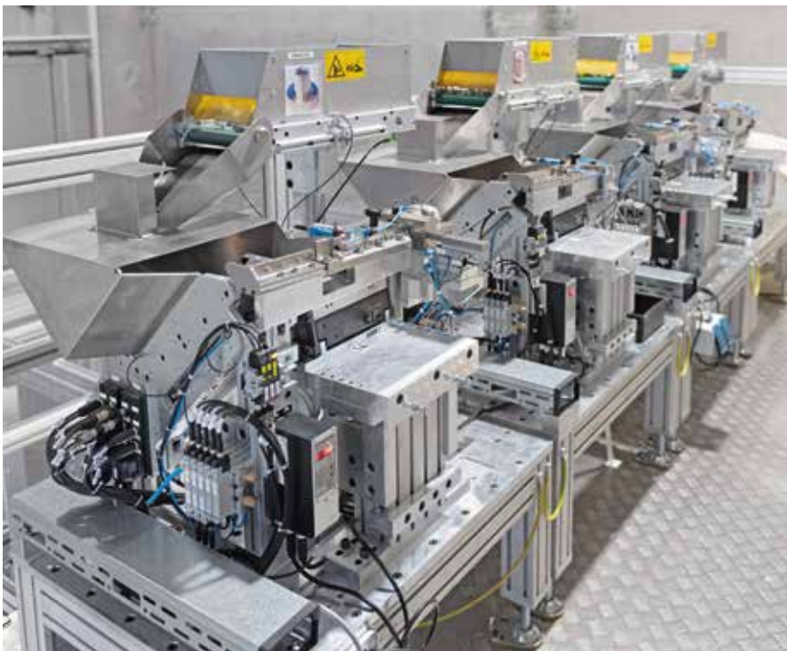
With efficient utilisation of space, 2R has divided an assembly system over two floors: From the upper floor (photo), the metal parts are separated, aligned and fed downwards via profiled hoses.
