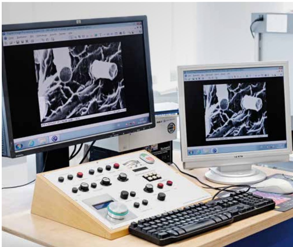
2R uses its own SEM to get to the bottom of fibre orientation in injection-moulded parts, for example.
