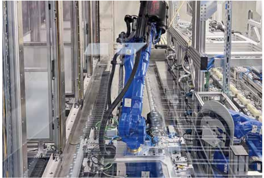
The pressure plates, which are produced on several injection moulding machines, are completed with fastening elements and dimensionally checked in an assembly system.
