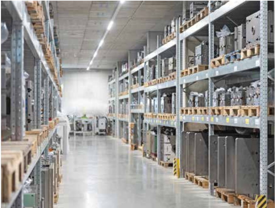
2R keeps around 500 active moulds in a brand-new tool warehouse – for current models as part of the supply obligation for at least 15 years after EOP.
