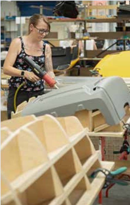
An employee applies the adhesive to the forklift bonnet with a glue gun to glue the yellow bonnet to the grey inner part.
