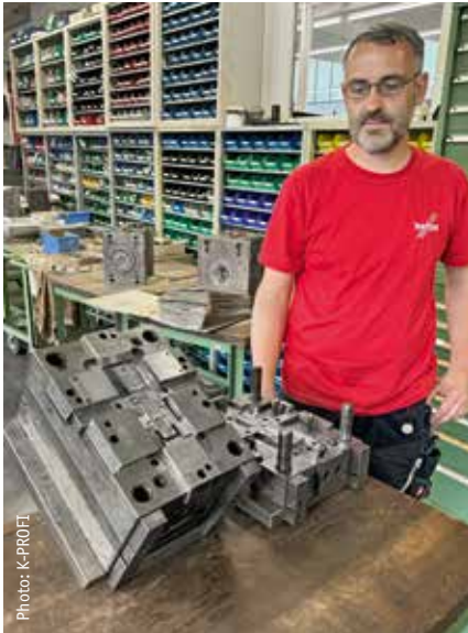
Holger Maier shows a modularised injection moulding tool with exchangeable inserts.
