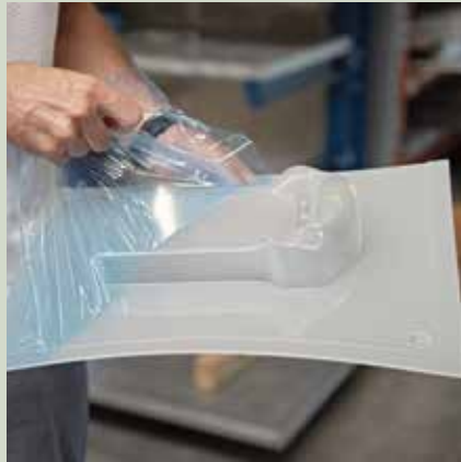
The film-formed upper shell for an orthodontic appliance is made of PMMA.
