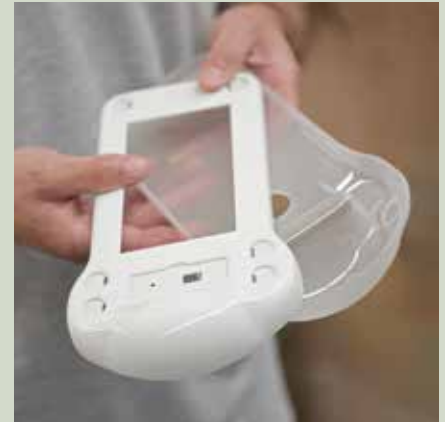
Here the same component after milling, together with its counterpart – the lower shell made of ABS-PMMA.
