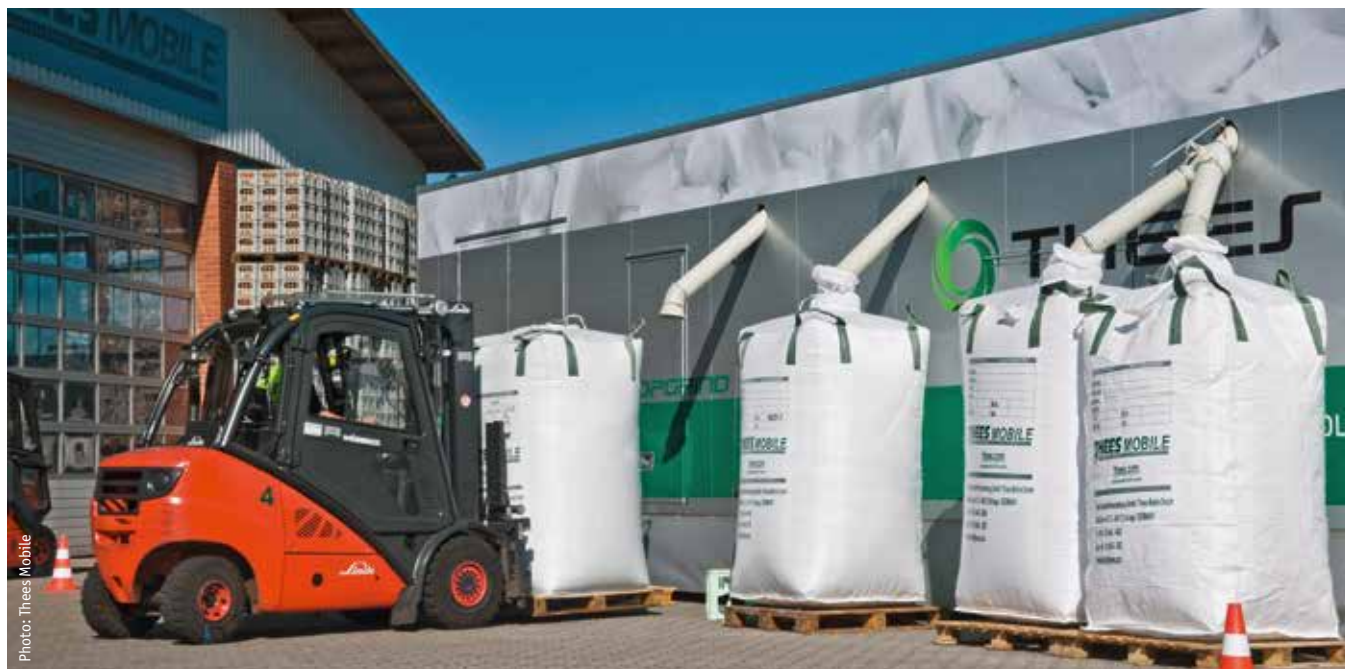
The mobile team of experts has everything they need with them: a soundproof container with the mill, pallets, big bags, outlet pipes and an electric forklift truck.
