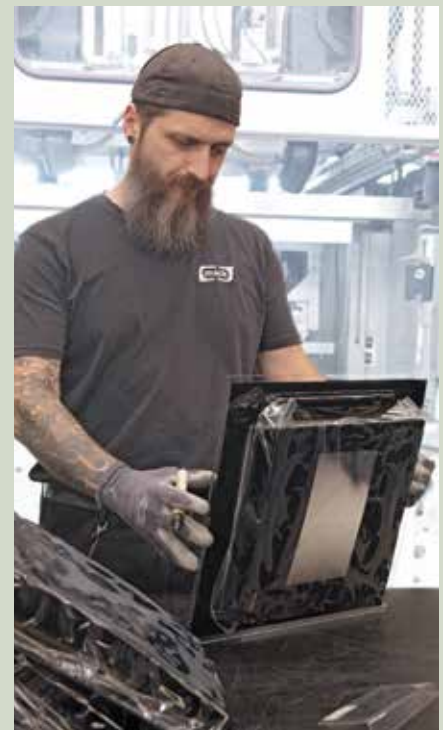
To avoid damaging the delicate surface, an employee covers the components with a film. After the subsequent hardcoat coating, the surface is scratch-resistant.
