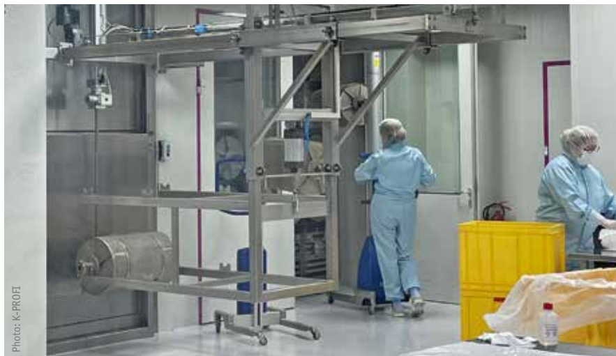
The trend is moving towards temperature-free LSR parts, but not for all applications. In addition to complete networking, the annealing process in the clean room at 200 °C also ensures germ-free nature.
