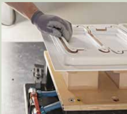
From a black-lacquered PC sheet, the company forms the component with a viewing window for a medical measuring device in a piano-black finish. The mould has a folding mechanism to allow the undercuts to be demoulded.
