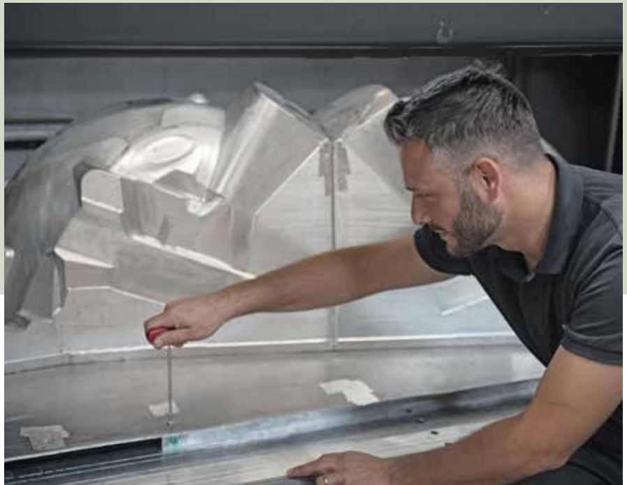
The employees are equipping the T10 with the 2-cavity mould for the wheel arch of the sports car.
