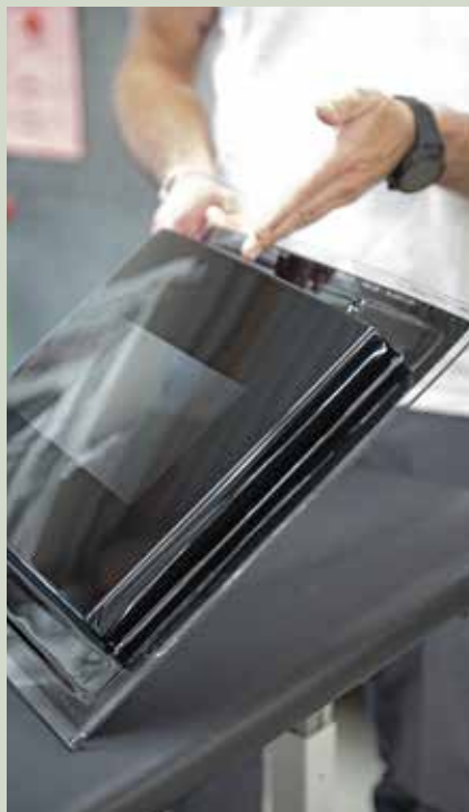
From a black-lacquered PC sheet, the company forms the component with a viewing window for a medical measuring device in a piano-black finish. The mould has a folding mechanism to allow the undercuts to be demoulded.
