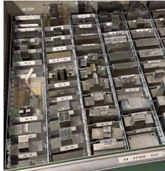
Herpa uses interchangeable inserts to limit the frequency of changeovers and ensure efficient injection moulding production.
