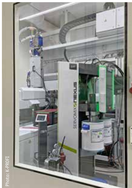
Trelleborg uses the variant of LSR metering directly in the newly established fourth clean room at the site, primarily for a blood glucose measurement application. Here at the validation run of the plant.
