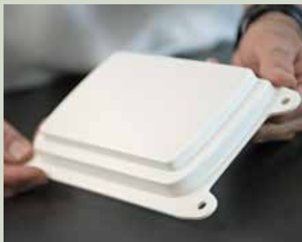
Bezel for an ART measuring device made of ABS: negatively drawn with a high-gloss surface and absolutely consistent radii before milling ...
