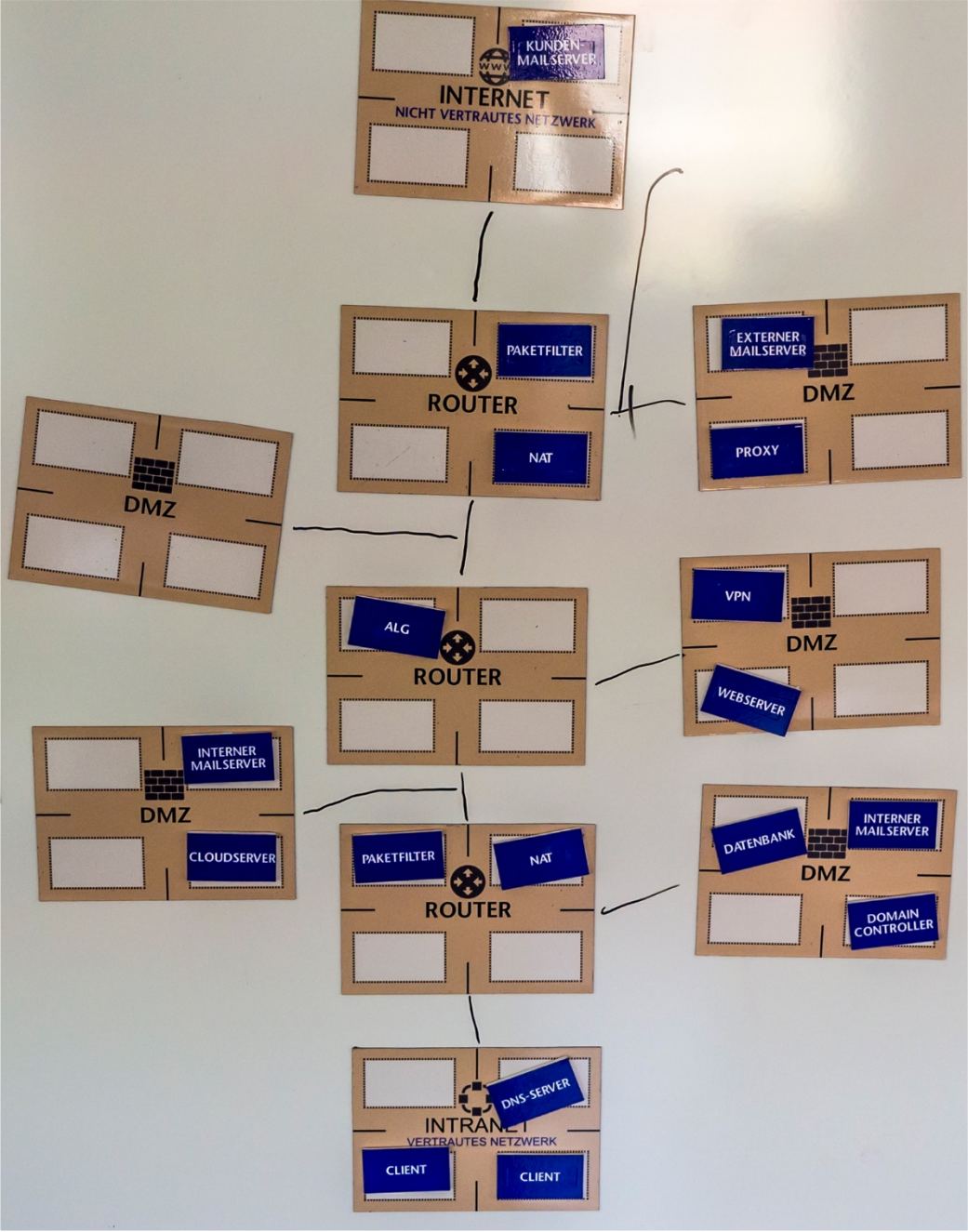
Fig. 90 TH Wildau’s analog learning scenario “Secure network architecture/network domains” for use in ISO trainings. It is used to illustrate the single- and multi-level architecture of secure gateways and consists of magnetic transparencies and signs that symbolize the individual technical components of networks. Routers use IP addresses to transport the data packets in the direction of the target network, while switches forward data blocks within a network to devices using hardware addresses. A distinction is made between packet filters and ALG (Application Level Gateways) as the basic components of a firewall. A DMZ (“demilitarized zone”) is used to protect other components in a separate, isolated environment (e.g., web server, mail server, guest Wi-Fi, etc.).
