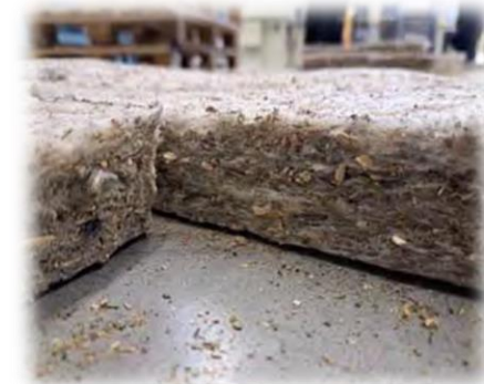
Insulation panel made with green waste
