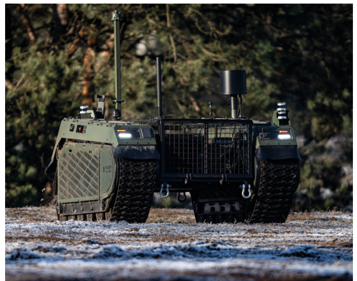
A TheMIS (Tracked Hybrid Modular Infantry System) from manufacturer Milrem Robotics takes part in a demonstration of the EU-funded iMUGS project. In Greek mythology, Themis is the goddess of justice. Photo: © picture alliance/dpa | Fabian Sommer.
