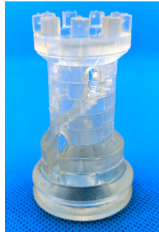
Figure 352: 3D printed tower with internal staircase. (Image Roser)
