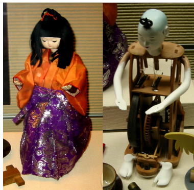
Figure 354: Inside of a Karakuri doll (Image World Imaging in public domain)
