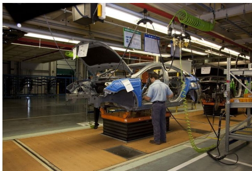
Figure 132: Hyundai assembly line with moving, walkable platform (Image Carol M. Highsmith in public domain)
