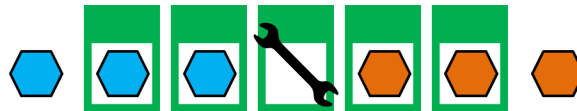
Figure 203: Sequential changeover while line running. The animated image can be found at https://www.allaboutlean.com/running-changeovers/ (Image Roser)
