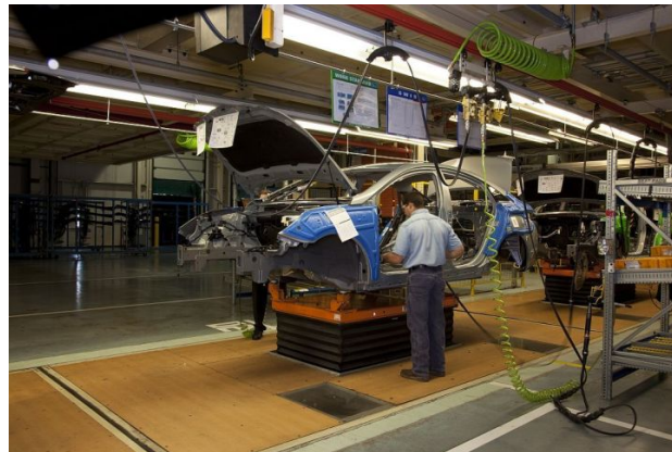
Figure 303: Hyundai moving walkable platform assembly line (Image Carol M. Highsmith in public domain)
