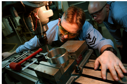
Figure 25: Batch size one part – milling (Image Kitt Amaritnant in public domain)
