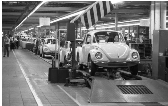
Figure 131: VW Beetle assembly line with underground pulling system (Image Schaack, Lothar under the CC-BY-SA 3.0 Germany license)
