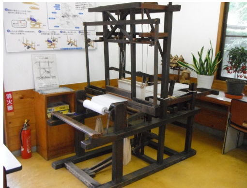
Figure 51: 1890 loom by Sakichi Toyoda (Image Yanajin33 under the CC-BY-SA 3.0 license)
