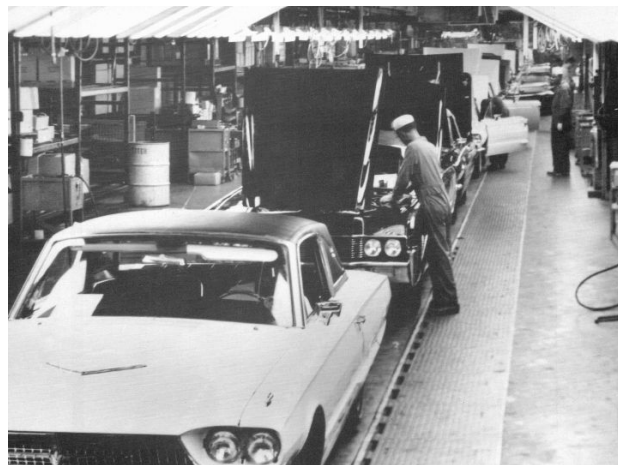
Figure 133: Ford Thunderbird assembly with pulling system (Image unknown author in public domain)
