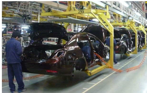
Figure 128: Continuously moving assembly line with hanging carriers (Image Siyuwj under the CC-BY-SA 3.0 license)
