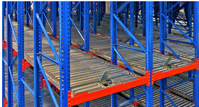
Figure 400: Warehouse rolling rack (Image praethip with permission)
