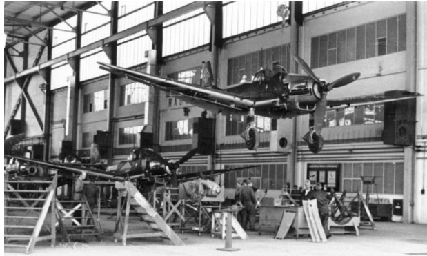
Figure 125: Junkers JU 87 pulse assembly line (Image Seuffert under the CC-BY-SA 3.0 Germany license)
