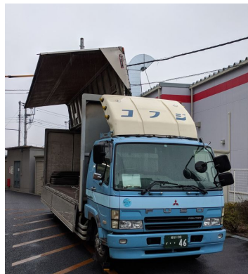
Figure 367: Gullwing truck with one wing open (Image Roser)
