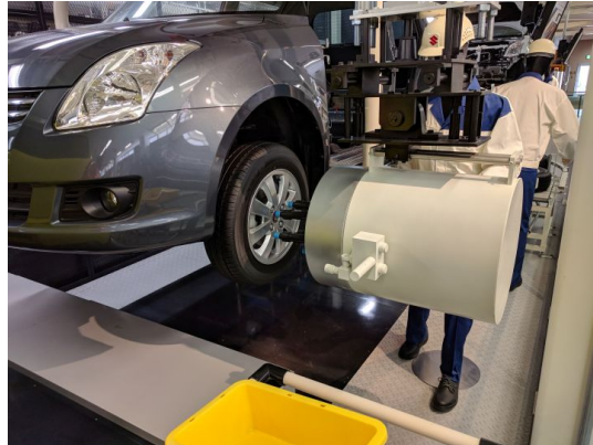
Figure 128: Wheel installation (Image Roser)
