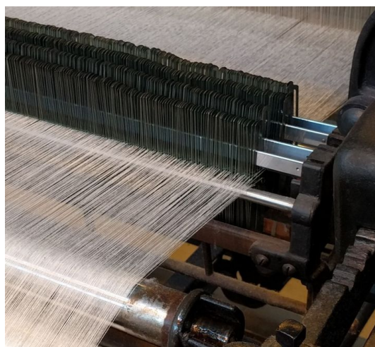
Figure 264: Toyoda Model G Automatic Loom Detail Warp Break Stop (Image Roser)
