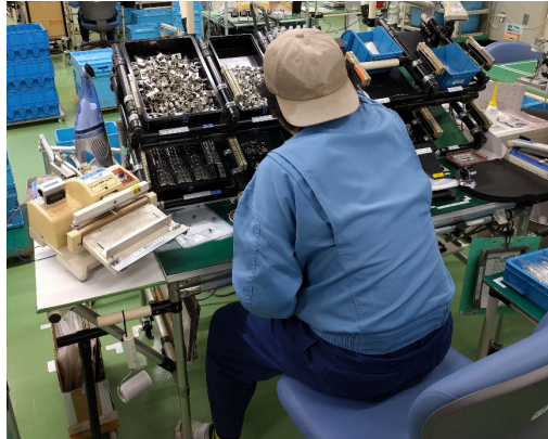
Figure 190: Pick by Light at Omron Kyoto at 130% of the speed of a non-disabled worker (Image Roser)
