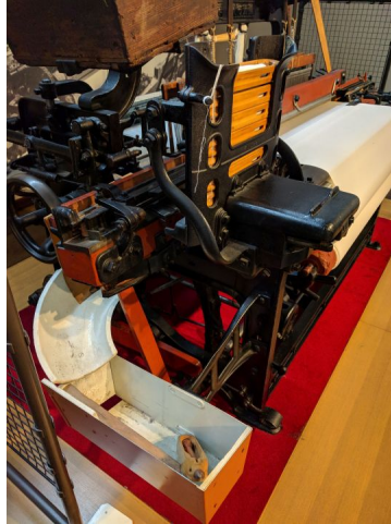
Figure 265: Toyota Model G Automatic Loom Detail Automatic Shuttle Change (Image Roser)
