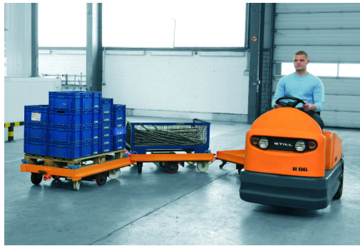
Figure 328: Electric Tractor Train (Image Still under the CC-BY-SA 3.0 license)
