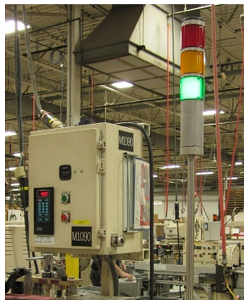
Figure 99: Stack light with three colors (Image Ktm250-1150gs under the CC-BY-SA 4.0 license)
