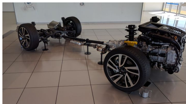
Figure 135: Subaru 4W Drive Train and Flat Engine (Image Roser)
