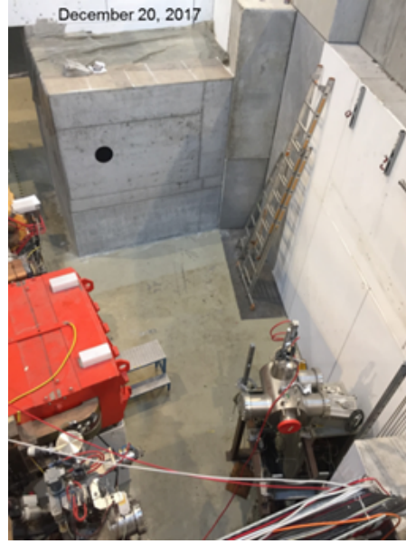
Figure 6: Cave of the mCBM experiment. A new beam dump surrounding the nominal beam position visible as a black circle had to be designed and constructed to enable the planned beam particle flux of 10^8 Au - ions per second at the highest SIS18 energy.
