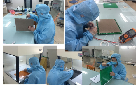
Figure 2: clean room and clean desk for MRPC mass production at the USTC site.
