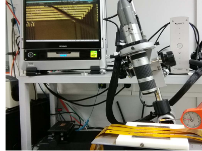
Figure 2: Test setup for destructive bonding force measurements.
