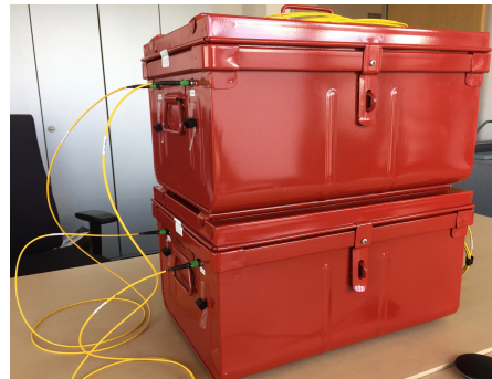
Figure 3: Long-haul optical connection test stand. Each box houses two strands of 8-fiber, single mode ribbon cable with 400 and 800 m.
