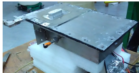
Figure 4: Photo of the sensor housing with the cover plate and the Al collimator/shield on top.
