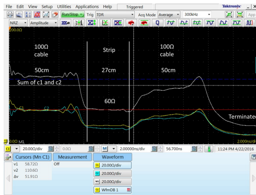
Figure 2: The impedance of the MRPC3a counter can be measured by the TDR method. It is 60 \Omega , which can be matched with the 50 \Omega PADI to eliminate the reflections.
