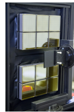
Figure 2: The proximity focusing setup with a 3 mm thick quartz glass radiator (left), and a typical integrated 2d hit map obtained with this setup.
