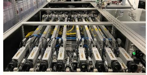
Figure 3: Photograph of the laser main amplifier stage.
