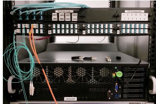
Figure 1: CRI setup in Gießen: Optical patch panel with 48 duplex LC connectors and FLES Input Node server.
