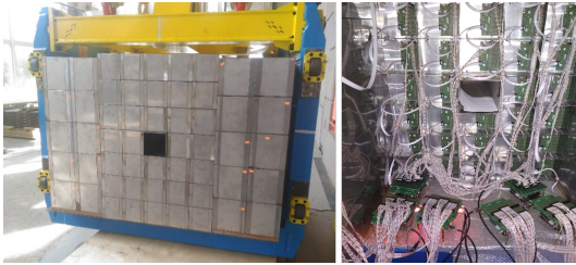
Figure 1: Left - front view of the BM@N FHCAL. Right – the backside of the FHCAL with installed FEE and readout electronics.
