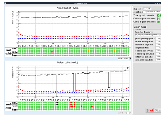
Figure 2: GUI: bonding of a microcable to 6x2cm sensor.
