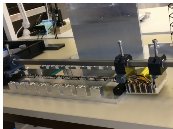
Figure 2: (a) Module positioned onto the ladder; (b) Prototype ladder assembled with five non-functional modules.
