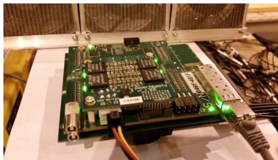
Figure 2: Photo of ADC64s2 board.
