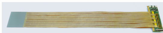
Figure 6: Full STS module assembled, awaiting to be fitted with the external microcable shield layer.
