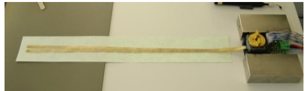
Figure 2: Test of TAB bonds between STS-XYTER-ASIC and microcable.
