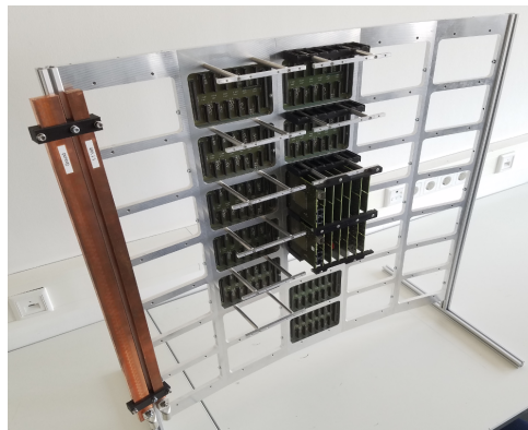
Figure 2: The first small scaled prototype of the CBM RICH camera with readout electronics. All electronic readout modules are fixed by using special clamps. On the left side you can see solid copper rails, these are going to be used for the low voltage / high current distribution.
