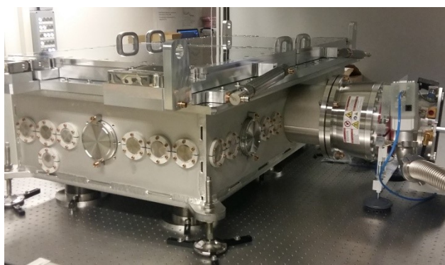
Figure 1: Vacuum chamber setup, which will host a femtosecond enhancement cavity for converting the infrared frequency comb into the XUV.
