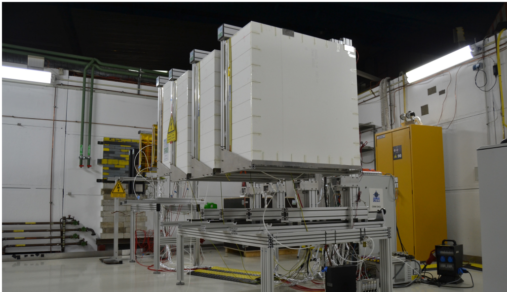
Figure 4.17: Picture of the four large TRD prototypes with radiators of type H in the experimental area at DESY.
