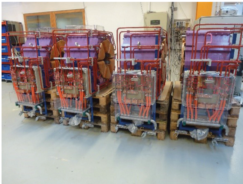
Figure 39. Resonance sextupole magnets manufactured at DANFYSIK
