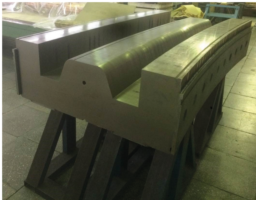
Figure 47. Yoke half of dipole magnet dip15_0.
