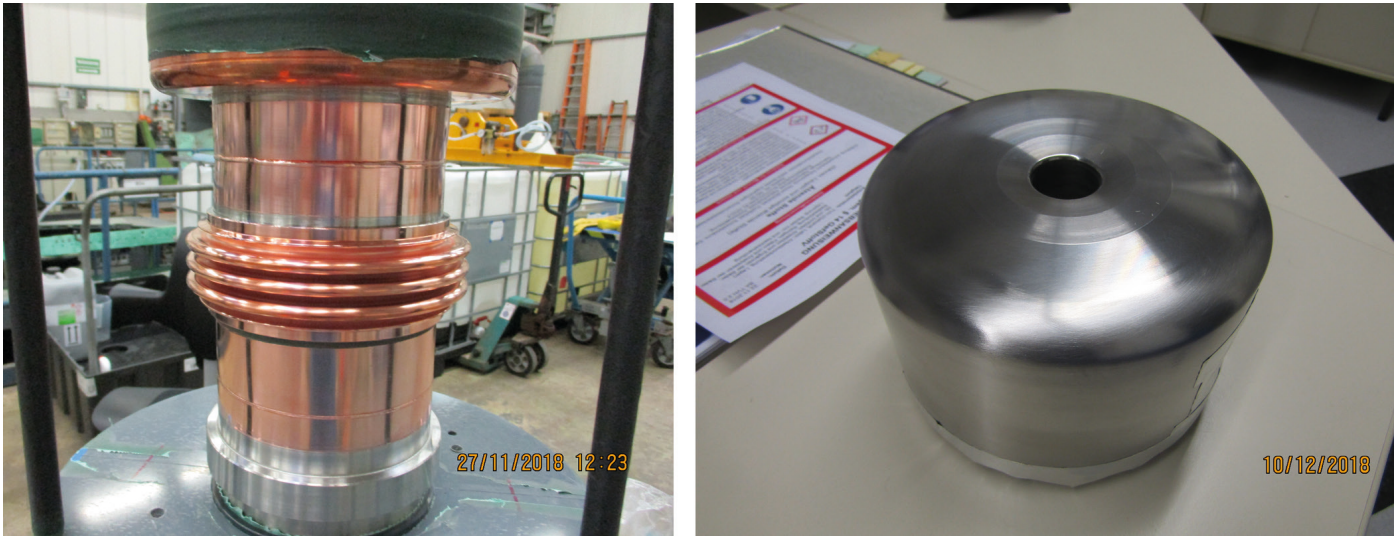
Figure 77. a) Left side of figure shows the Cu-plated so-called 'Spillglättungskavität' for SIS18, b) on the right side the a first drift tube for the Unilac post-stripper FOS is shown before Cu-plating.
