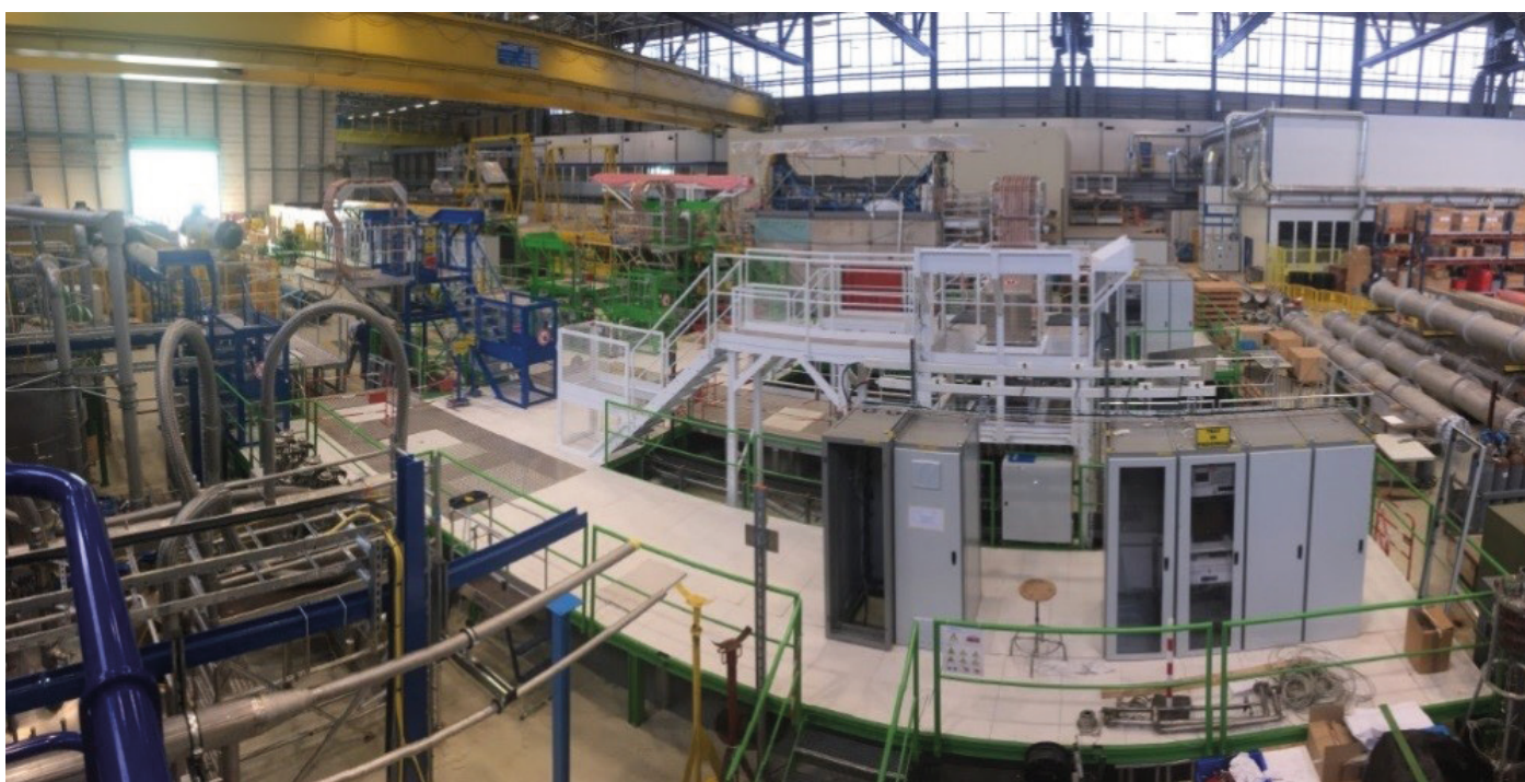
Figure 40. Testing facility at CERN for the SAT of super FRS SC magnets
