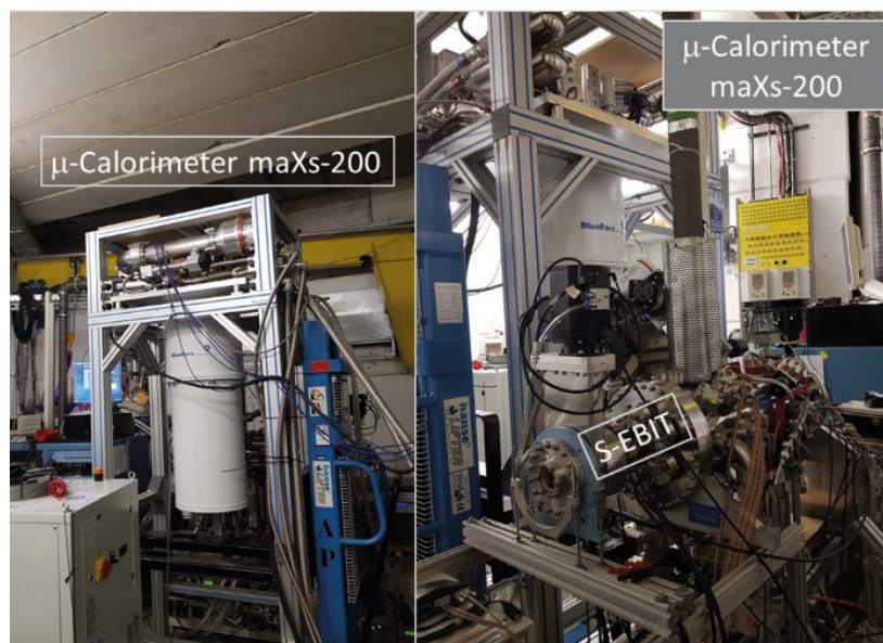
Figure 7. Pixel \mu -calorimeter developed at the University of Heidelberg.
