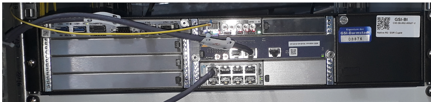
Figure 49. CUPID DAQ system: 6-Slot MTCA.4 setup with White Rabbit timing receiver (FTRN-AMC) and 8-Channel GbE Switch AM217 from Vadatech for GbE camera readout
