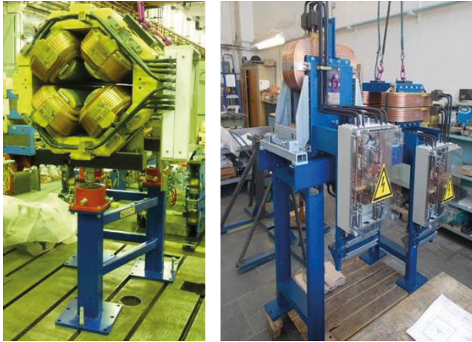
Figure 46. Quadrupole magnet quad2 and steering magnets s100h/v at BINP.
