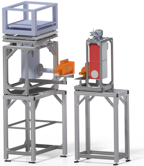
Figure 1: Left: Detector assembly used at the 180° port with Blufors cryostat. Right: Detector assembly for use at the 0° port using a compact MiniMix cryostat. Bright orange: accompanying Ge(i) detectors.
