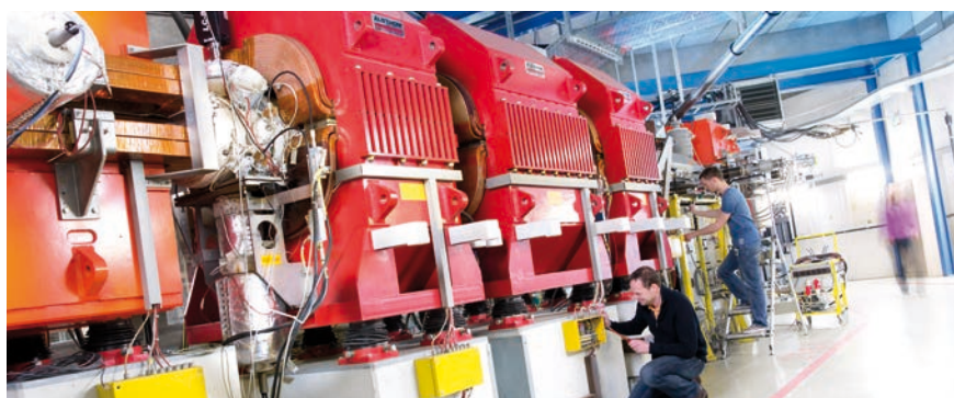
The experimental storage ring ESR at GSI.
