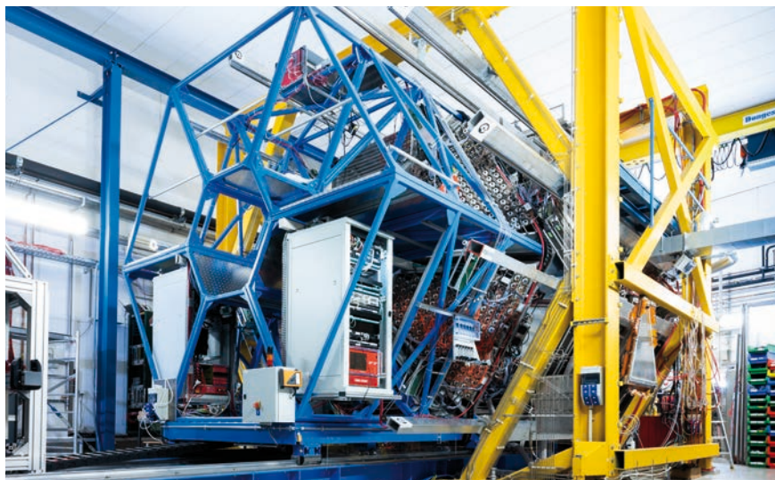
The ECAL on the rail system is connected to the existing HADES detector.
