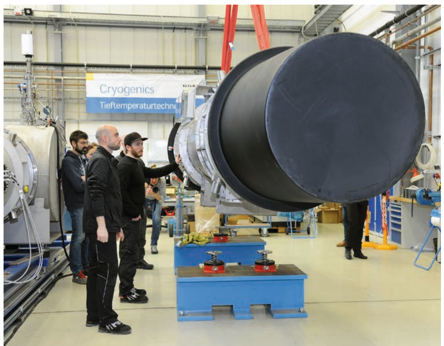
On the hook: With a crane the quadrupole module is carefully lifted to its place.
