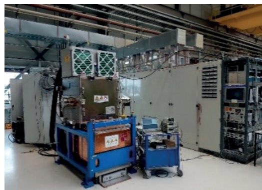
Figure 58. The 2 nd of series RF debuncher system during the commissioning at the GSI testing hall.
