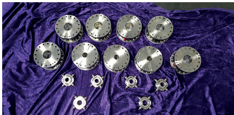
Figure 55. p-Linac Beam Position Monitors. Inter-Tank types (small), Beamline types (large).
