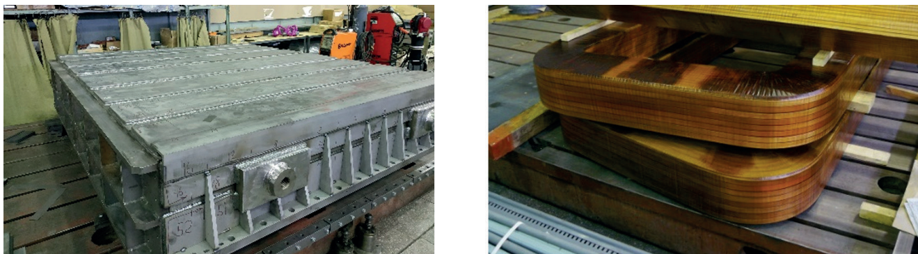
Figure 56. First completed upper plate of the dipole yoke (left) and first set of coils (right) at BINP.
