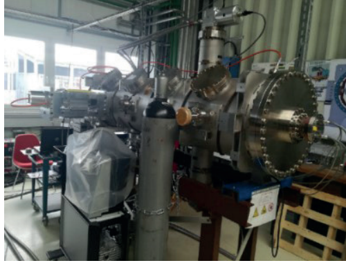
Figure 59. Assembled prototype slot-line pick-up prepared for cryogenic testing at the GSI test bench.
