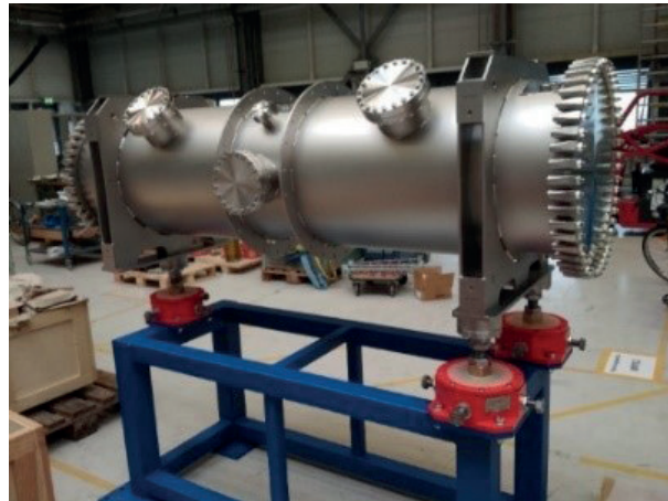
Figure 61. The Palmer pick-up vacuum tank at the GSI testing hall at the intensity of 108 ions/cycle.
