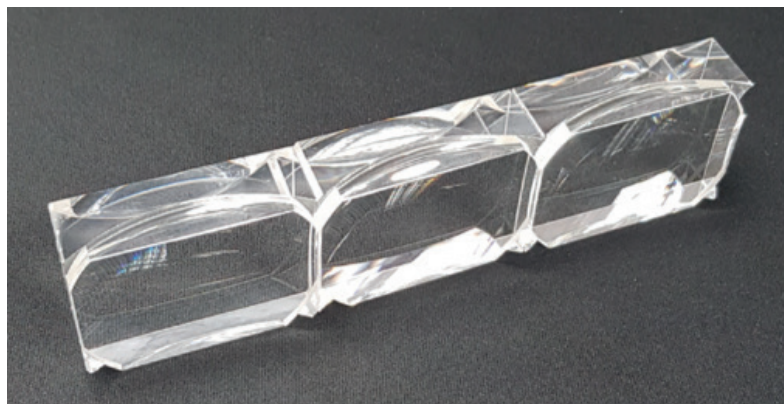
Figure 40. 3 layer-spherical lenses for the PANDA Barrel DIRC.
