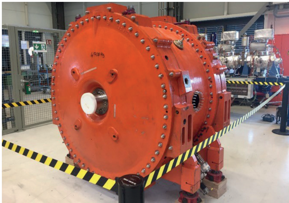
Figure 48. New SIS18 micro spill cavity for FAIR Phase-0.
