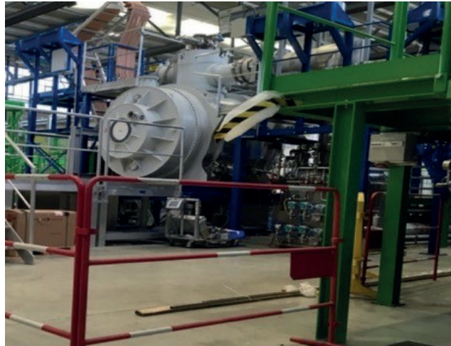
Figure 51. FoS SC short multiplet on its testing bench (CERN, Geneva, Switzerland).
