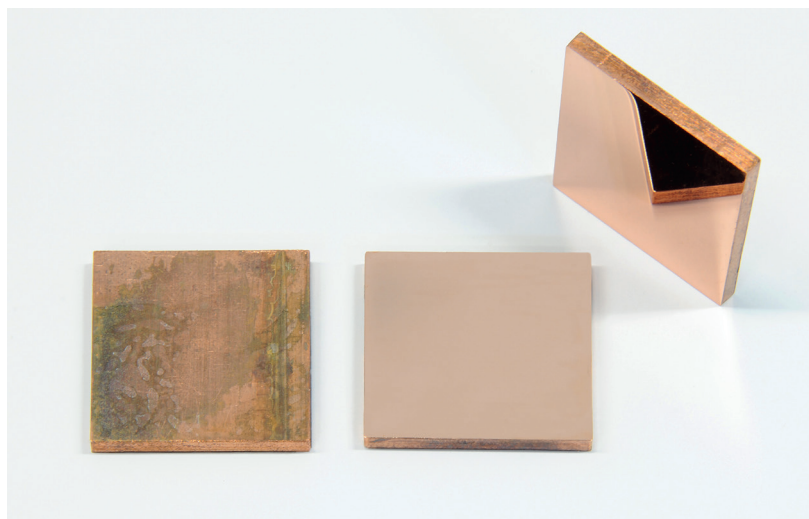
Figure 44. Starting material versus lapped and polished copper samples as part of the materials research test series, where the smoothest possible, pore-free surfaces are investigated, which ensure minimal adsorption and thus small desorption rates of residual gas particles in accelerator components (Photo: G. Otto, GSI)
