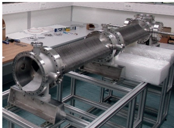
Figure 50. SIS18 cryogenic test chambers at ILK, Dresden.
