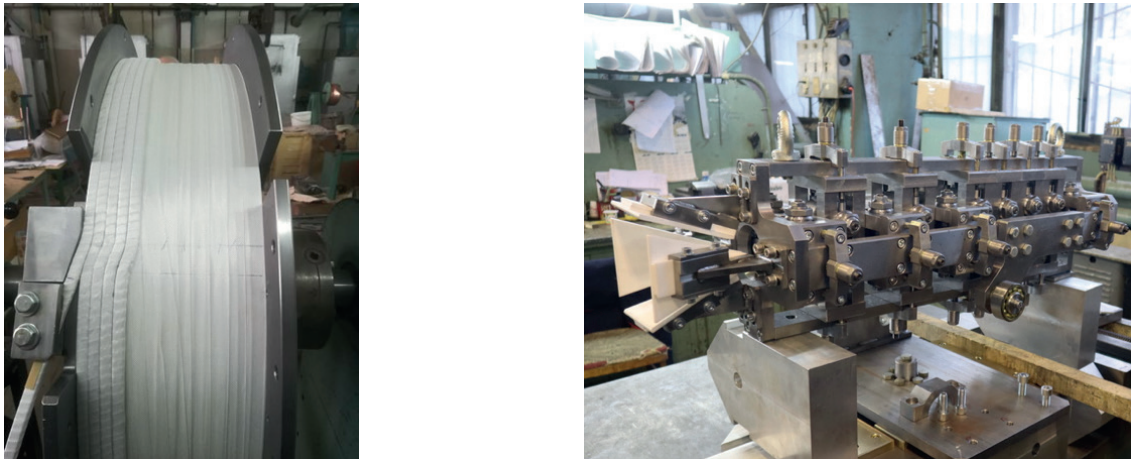
Figure 38. Sample coil winding with aluminium cables for the PANDA super-conducting magnet (left) and winding tool.
