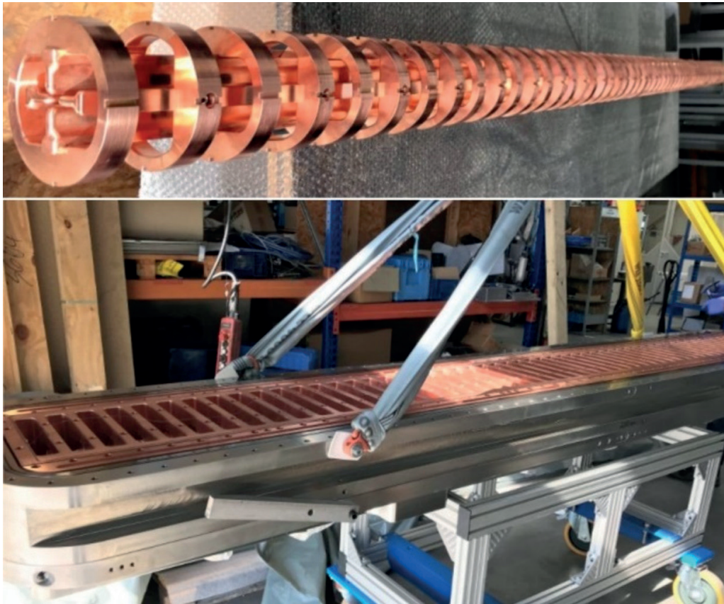
Figure 53. Full length RFQ electrode structure with rings (top). Assembly of the ladder structure inside the RFQ tank (bottom).
