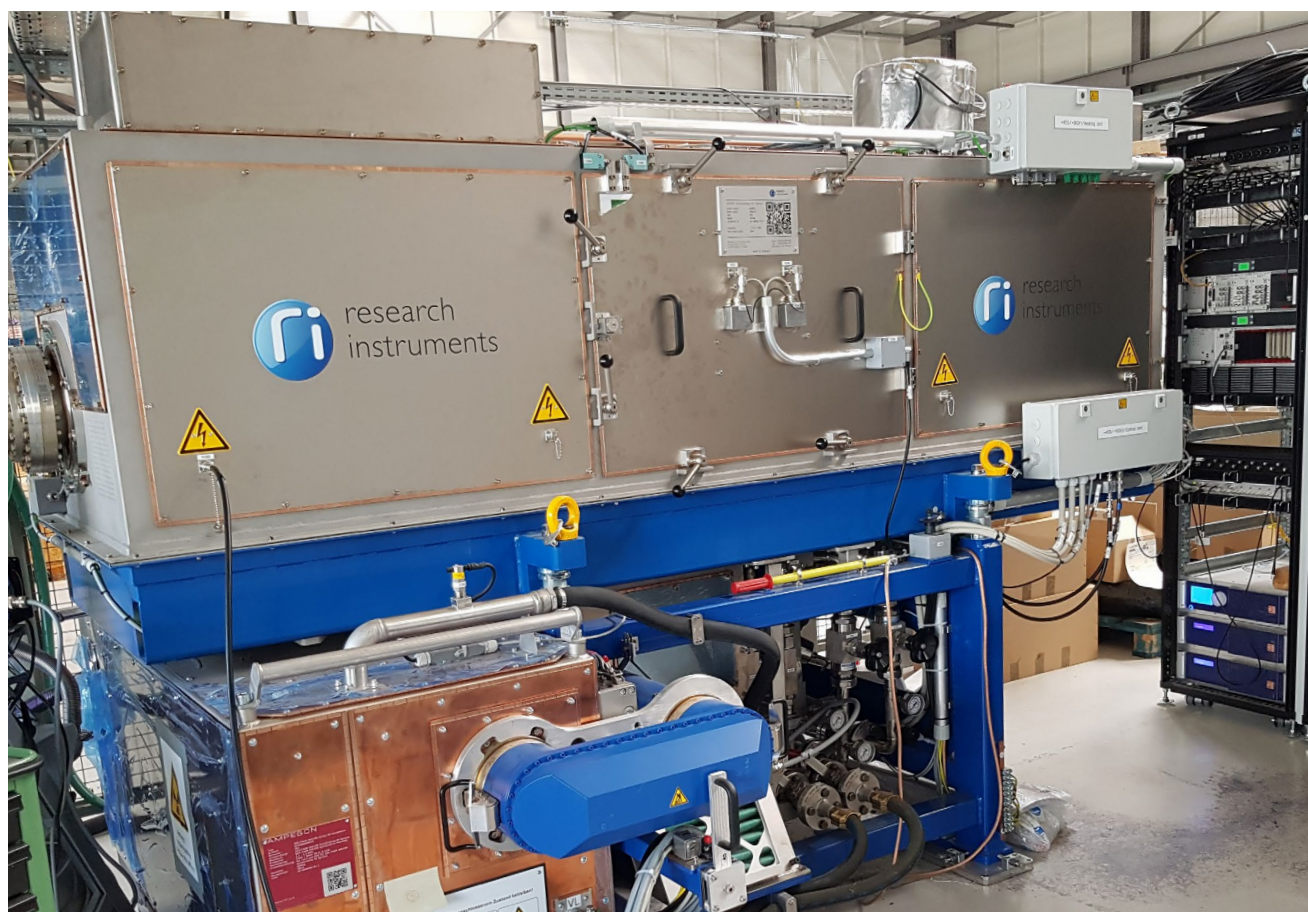
Cavity realised by RI Research Instruments including the electronics mainly developed by the GSI department "Ring RF" in the background.
