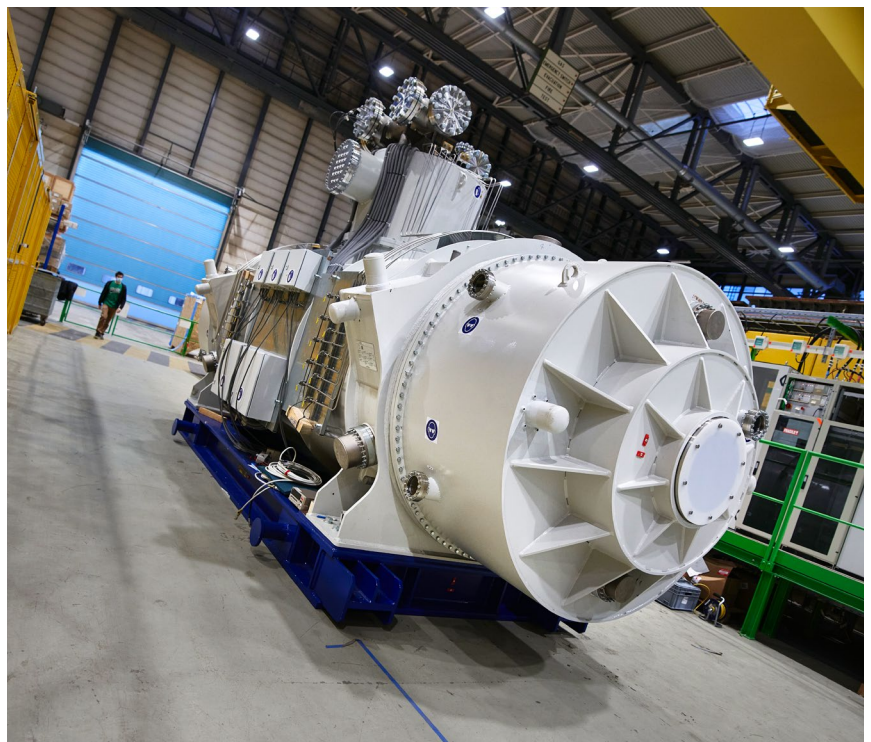
The long Super-FRS multiplet on site at the CERN test stand.
