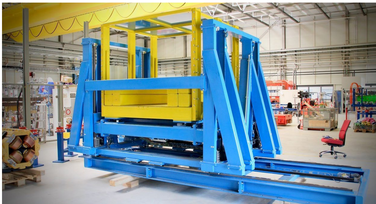
Manipulator for the PSD detector of the CBM experiment at FAIR.
