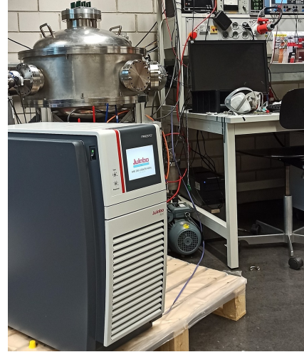
Figure 1: JULABO TM PRESTO A40 cooling system.
