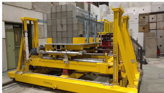
Figure 2: The upgraded NA61/SHINE MPSD which uses 13 CBM PSD modules.
