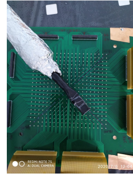
Figure 1: Setup of RPC with the finger scintillator and PCB P1.
