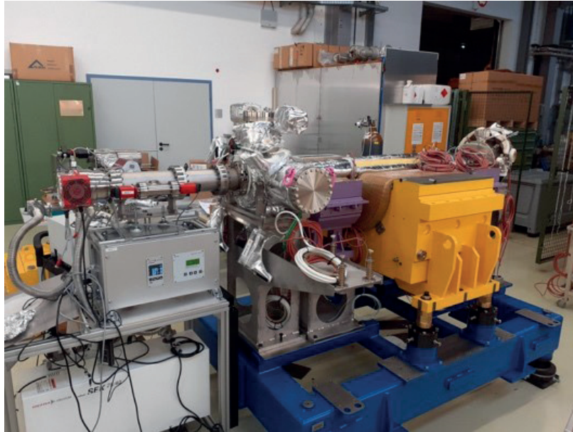
Figure 72. Components along the beam (left to right): Large pumping chamber 'fixed bearing', sextupole magnet, quadrupole magnet, beam position monitor with vacuum chamber extensions, sextupole magnet, small pumping chamber 'floating bearing'. All vacuum chambers or pipes are equipped with heating jackets. Turbomolecular pump attached to the pumping chamber 'fixed bearing' to allow immediate check of the vacuum assembly.
