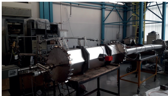
Figure 71. Mock-up installation for vacuum testing of the dipole and quadrupole/sextupole chamber assembly at BINP.
