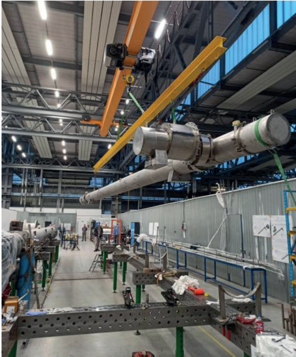
Figure 61. Lifting of a bypass line at company Kriosystem (Poland) in preparation of the delivery to FAIR.
