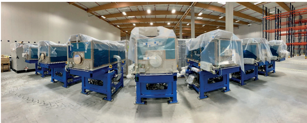
Figure 59. Series of ferrite-loaded acceleration cavities in storage area Weiterstadt.
