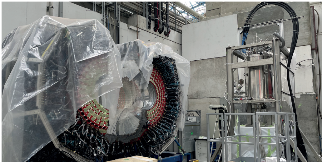
Figure 42. The WASA test stand in the Target Hall of GSI. The central detector is seen on the left, on the right side there is the cooling system with the s.c. solenoid underneath.
