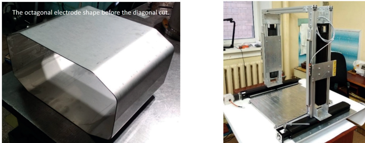
Figure 70. Testing sample of the re-designed octagonal BPM electrode (left) and the completed BPM test stand (right) at BINP.
