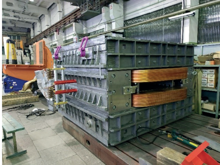
Figure 69. First of series CR dipole magnet assembled at BINP (Russia).
