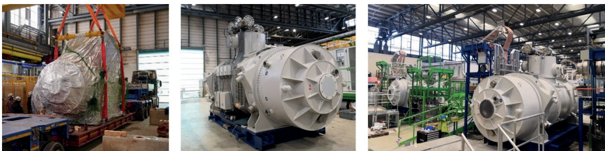
Figure 63. Left, middle: FOS sc long multiplet delivered to the testing station at CERN. Right: short (on the left side) and long multiplets (on the right side) on two testing benches.
