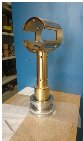
Figure 90. Prototype cryogenic insert for the room temperature ion catcher system in SIS18.
