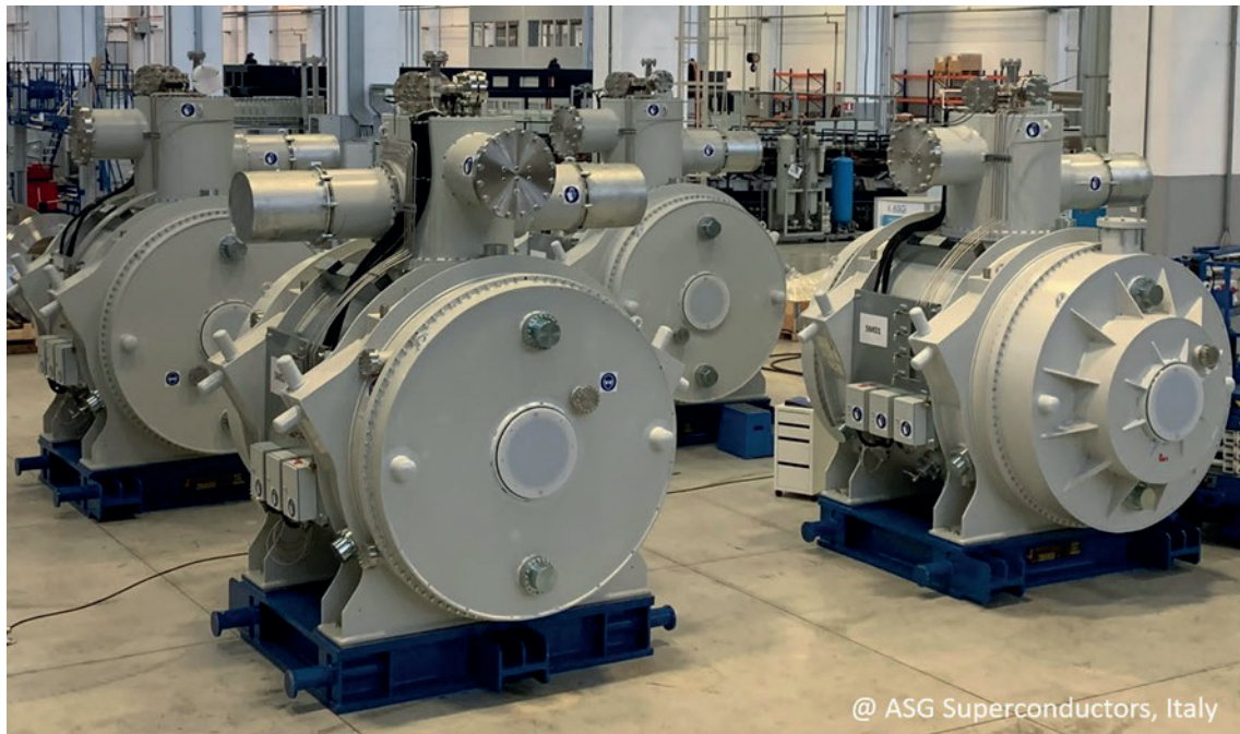
Figure 94. Executing the series production of SC multiplets at ASG in La Spezia (Italy).
