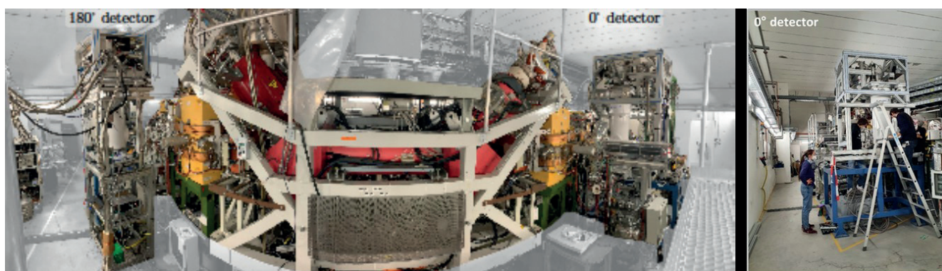
Figure 12. Implementation of a novel high-resolution, cryogenic \mu -calorimeters each equipped with a 64 pixel area. In the figure, one of the two \gamma -calorimeters is displayed at its final position at the 0 deg port at the CRYRING@ESR electron cooler (upper part).
