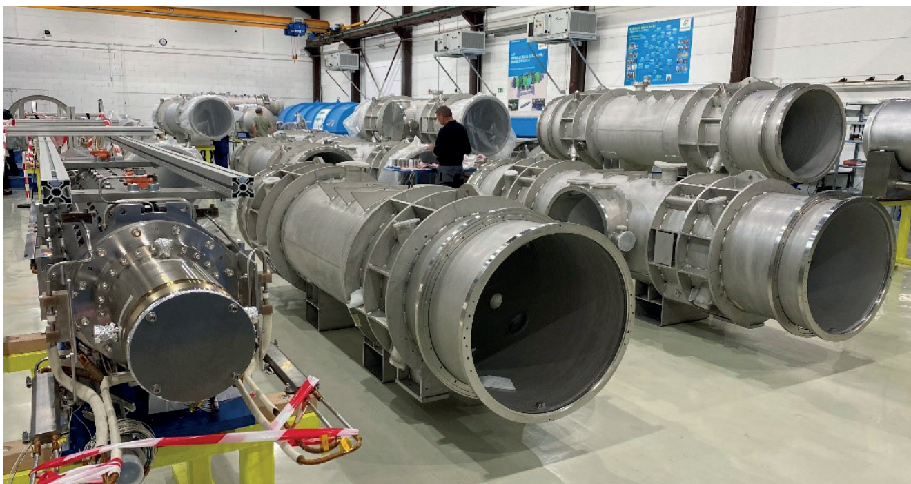
Figure 91. Quadrupole module integration at Bilfinger Noell, Würzburg.
