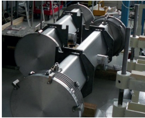
Figure 103. Wide hexagonal chamber prototypes at BINP workshop.
