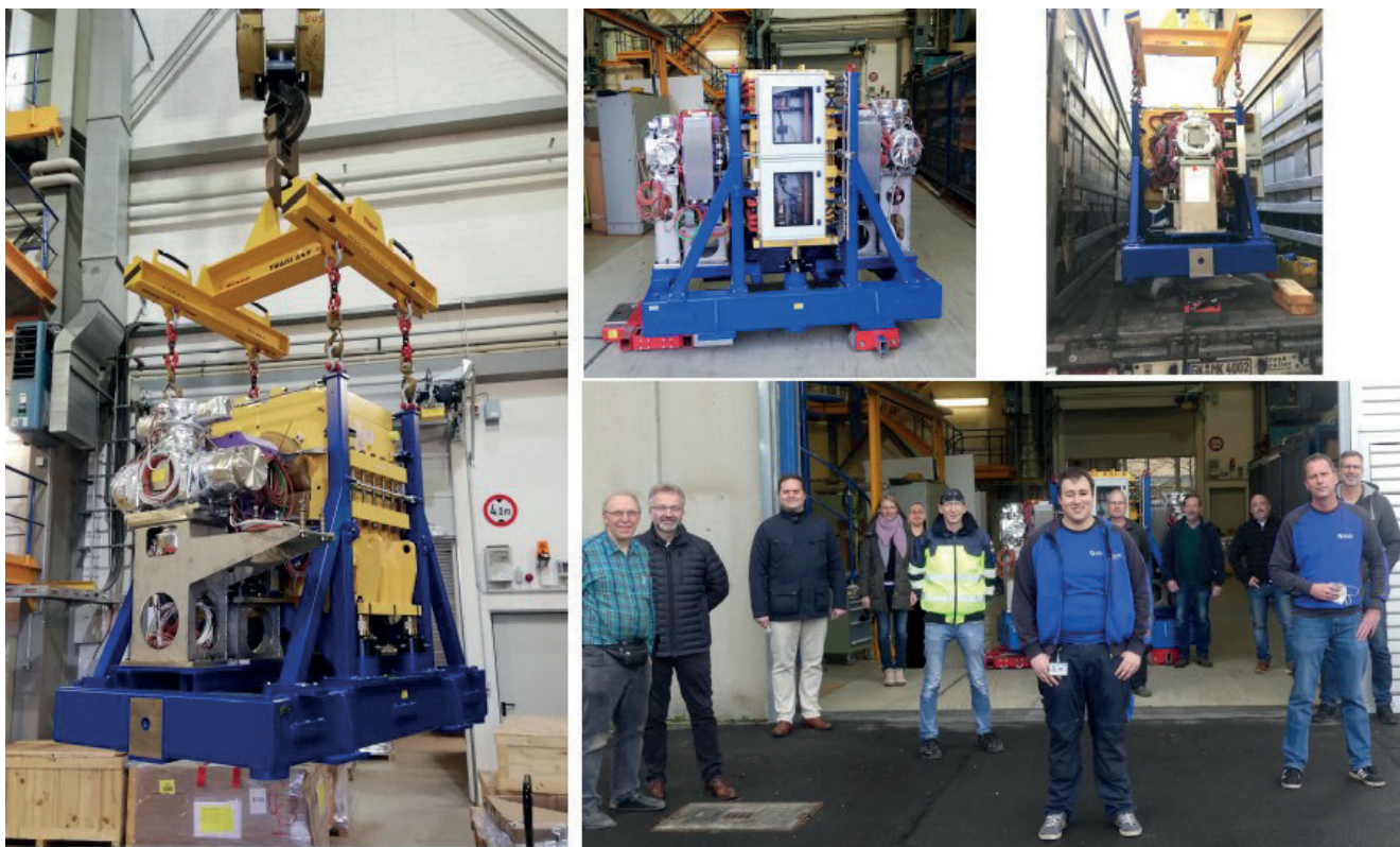
Figure 105. Loading the first HESR quadrupole assembly for transport to Weiterstadt.
