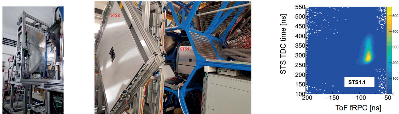
Figure 38. Left: Photograph of the front view of the two sectors of fRPC. Middle: Photograph of the back view of the two stations (STS1/2) of four double layers of self-supporting gas-filled straws. Right: Correlation of STS TDC time and time-of-flight information from fRPC from test run in February 2021.
