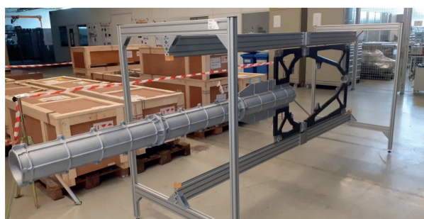
Figure 55. Assembled Central Space Frame (CSF) prototype (Photo by S. Koch, GSI).
