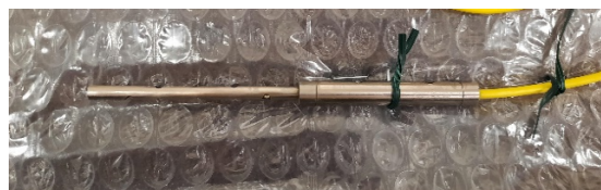
Figure 8: Temperature and humidity FBG-based FOS.
