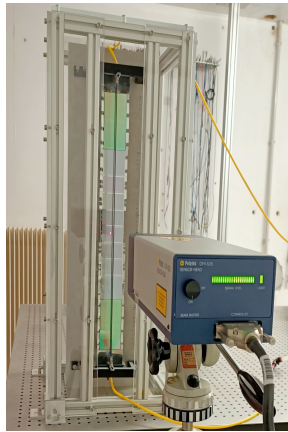
Figure 6: Setup for ladder vibration measurement.
