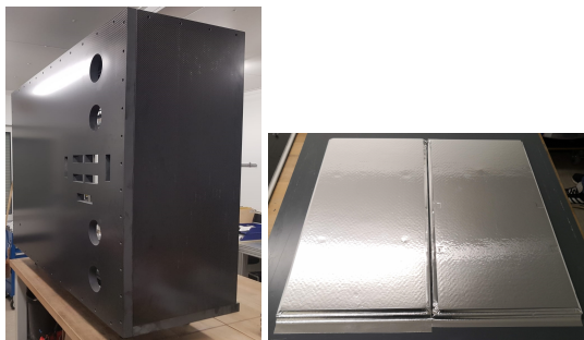
Figure 5: Left: CF-Foam sandwich panels mounted on the mainframe; Right: Vacuum bagging of aluminium foils on CF-foam panels.
