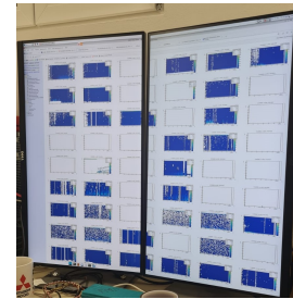
Figure 3: Picture of Online monitoring canvas for FEB by FEB electronics channel plots. Maximum of 54 FEBs can be connected under 6 CROBs. Blank space shows that particular FEB is not connected.
