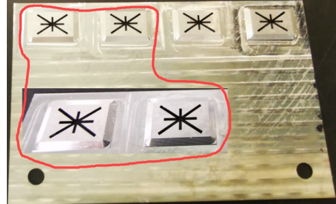
Figure 1: Step stencil and zoomed-in section.
