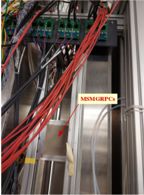
Figure 1: The counters installed in the experimental setup.
