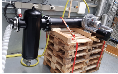
Figure 1: Picture of the prototype cooling system setup in the lab, consisting of a large water-air heat exchanger with water separator, fed by a small sidechannel blower to be used for the first tests (left).
