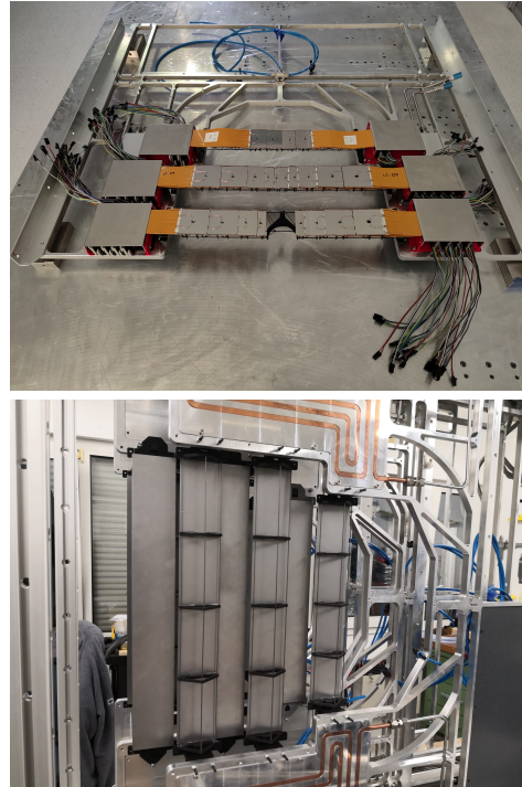
Figure 6: Top: 'Active' C-Frame with thermal dummy ladders; Bottom: 'Passive' C-Frame on the mainframe.
