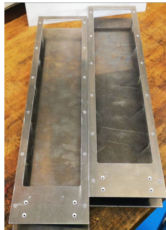
Figure 2: Two module carriers prepared to be equipped with signal distribution boards.
