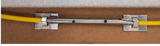
Figure 9: Humidity FBG-based FOS in an array.
