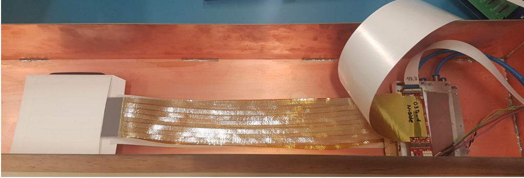
Figure 1: Part of the setup including the module, the shielding box, a cooling plate and necessary electronics for the read-out.
