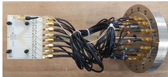
Figure 4: Prototype T0 detector build for the mCBM experiment. The diamond sensor is bonded on a PCB which is pneumatically driven into the beam-line in front of the target [3].
