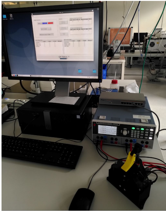
Figure 1: Complete setup with computer, power supply and FEB8 test box (from left to right).
