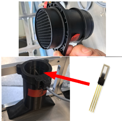
Figure 1: The BOSCH HFM7-R5 (top) is a pre-calibrated mass-flow sensor to be used for measuring the total cooling airflow into the CBM RICH air distribution system. FLW122 (bottom) is a "naked" mass flow sensor without further readout electronics. It comes without any pre-calibration (which will depend on the exact installation situation anyway), and will allow to measure air flow at different locations inside the camera.
