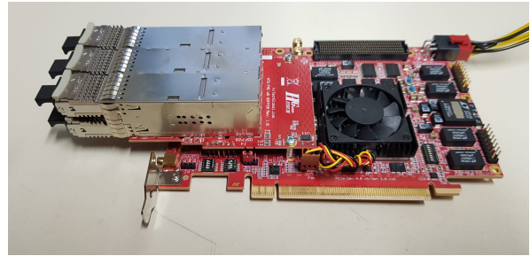
Figure 1: HTG-Z920 board with a mounted QSFP+ module for testing GTY functionality
