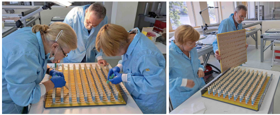
Figure 2: Assembling of the readout electrode.
