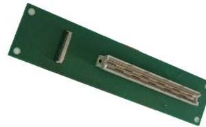
Figure 3: Signal distribution for the module carrier box.
