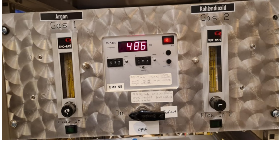
Figure 1: Gas Mixing Unit
