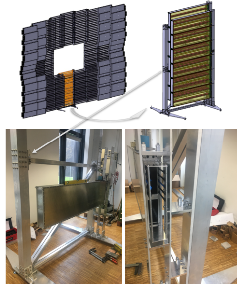
Figure 2: Mock-up stand simulating the lower part of the central column of the TOF wall. Lower photos show a stress test with heavy weights placed inside the module.
