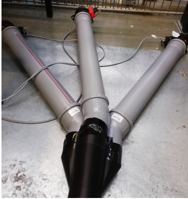
Figure 3: Setup of the first test measurement of the BOSCH mass air flow sensors: incoming air is equally distributed into three output channels through the three-way splitter (black), homogenised within conventional tubes that are attached (grey) and finally measured with the sensors.
