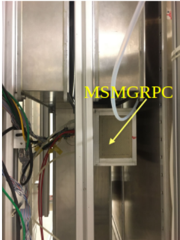
Figure 1: Direct flow P2 prototype in the mCBM setup.
