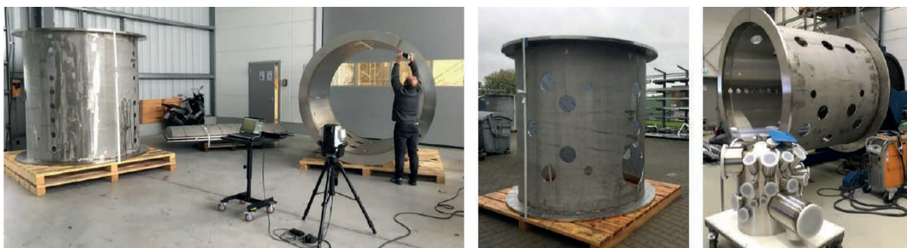
Figure 67. Production of the five cavity section mantles forming the first cavity
