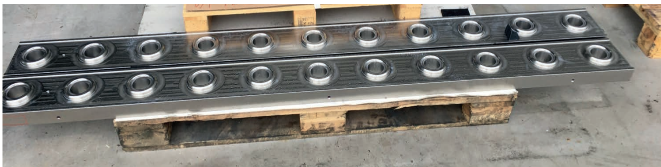
Figure 68. Interface assemblies to be welded onto the cavity mantle; they serve to install the drift tubes
