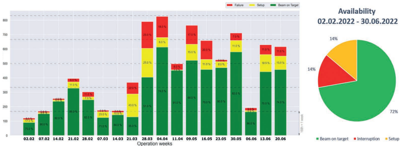
Figure 58. The diagram (left) shows the different event durations during the experimental beamtime 2022. Each bar represents a period of one week, starting from the date shown on the x-axis and ending on the following Sunday. The colors green, yellow and red depict beam on target, setup, and interruption respectively. In the case of experiments running in parallel, the times are summed up. Each of the horizontal dashed lines marks a one week period, so that the parallelism factor can be read on a weekly basis from the height of the bar. Between the end of March and end of June, there was an average of about four experiments in parallel operation. An exception is the week from June 6th, in which mainly machine experiments took place, which are not taken into account in this diagram. The parallel factor over the entire experimental beamtime is 2.6 and was lower than in previous year, which can be attributed to the exclusive proton beamtime. The right picture shows the overall availability for the experimental beamtime 2022.
