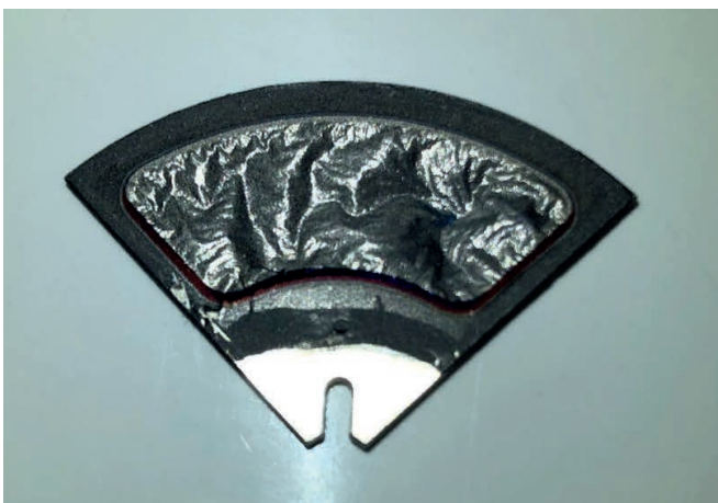
Figure 97. Left – Metallic uranium with 360\ \mu\text{g}/\text{cm}^2 on 40\ \mu\text{g}/\text{cm}^2 carbon backing; Right - \text{UO}_2 with 100\ \mu\text{g}/\text{cm}^2 (based on U) on 50\ \mu\text{g}/\text{cm}^2 carbon backing.
