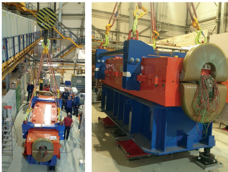
Figure 91. Air cushion tests on the dipole magnet on 20.12.2022 in the IKP test hall of Forschungszentrum Jülich. For safety reasons, the dipole was fastened to the indoor crane.
