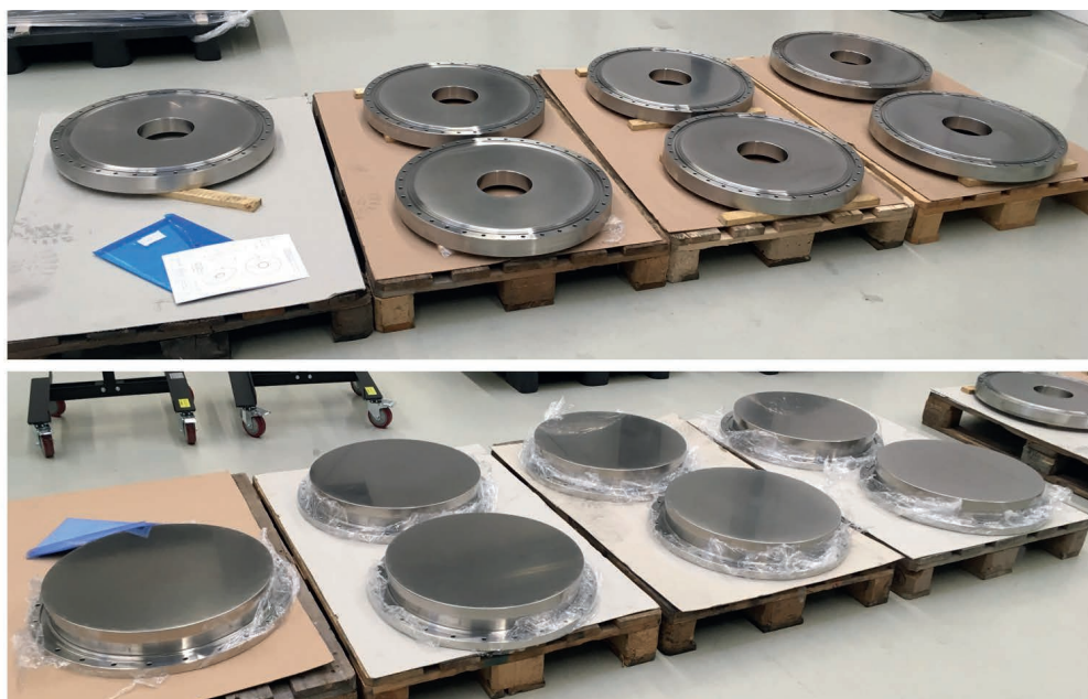
Figure 69. Flanges to provide for RF-coupling (upper) and to close the maintenance ports (lower)
