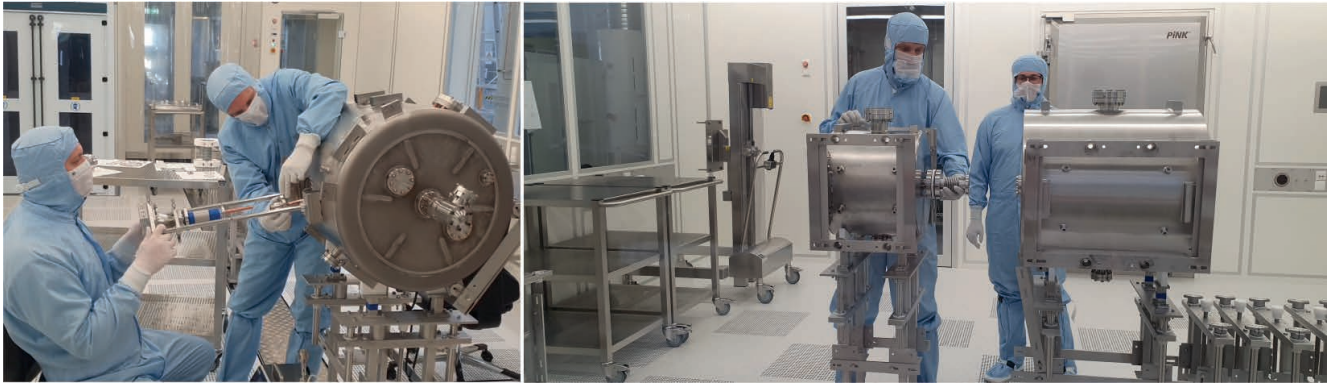
Figure 75. Integration of the rf-power coupler into a superconducting cavity (left); interconnection of the sc solenoid and the CH2 cavity (right).
