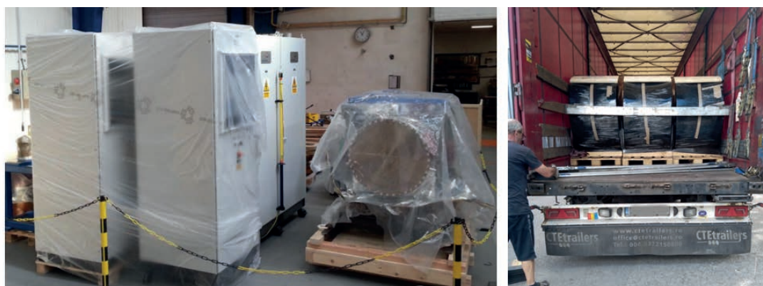
Figure 92. Injection equipment Tank B ready for packing (left) and on the truck (right). Four magnets with pulsers and cables are in Weiterstadt now. The magnets are housed in 2 vacuum chambers pairwise.
