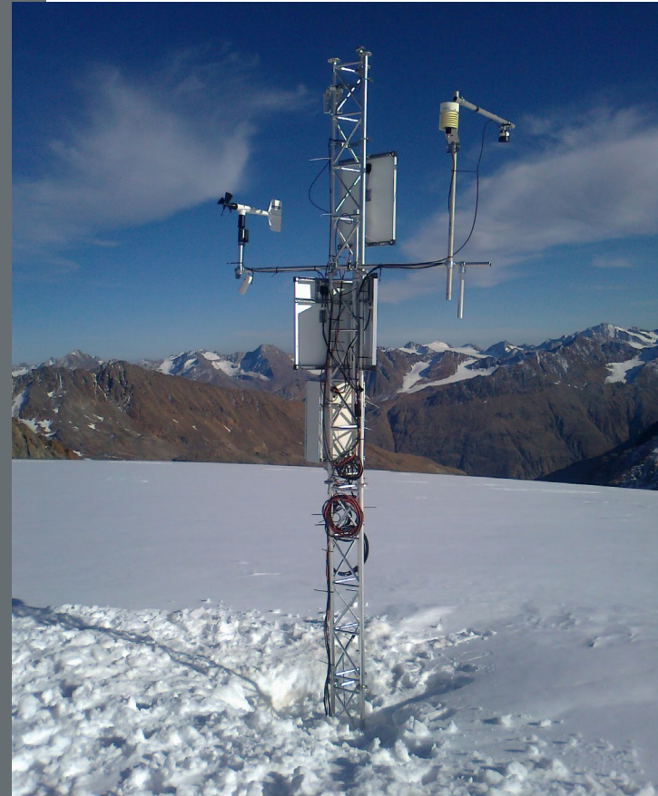
◀ Photo 6.2-2: Automatic weather station on the Vernagt high plateau at 3,450 m. At this station, measurements are carried out to continuously monitor the evolution of snow cover and record the key meteorological components.
