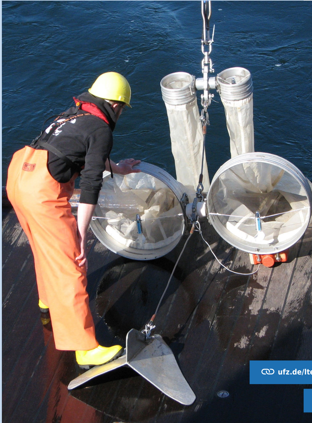
◀ Photo 3.16-2: Quantitative plankton net catches remain an integral part of long-term plankton observations. Depending on the target group, plankton nets with different diameters and mesh sizes are used. The picture shows a bongo net (combined with baby bongo).
