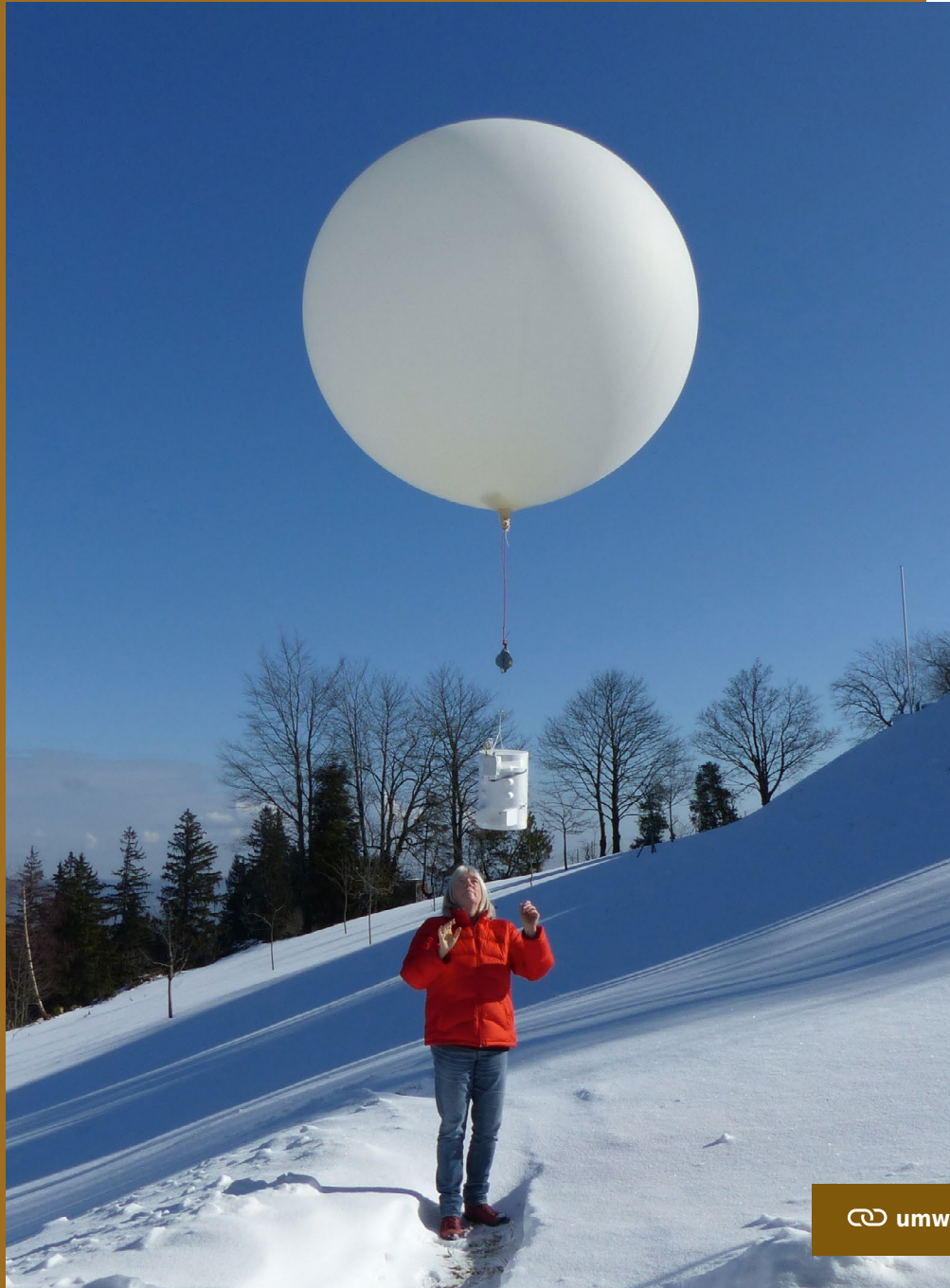
◀ Photo 2.14-1: Launch of a balloon-borne ozone sonde at the MOHp
