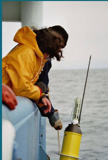
◀ Photo 3.2-2: Launch of an Argo deep float into the sea. Once deployed for 3 to 5 years depending on the design, the float will collect vertical profiles of temperature and salinity from the surface down to a depth of 2,000 m as well as information about current flow at around 1,000 m down in the ocean every 10 days and transmit these to the global data centre for Argo. At present, the Argo observing network is being extended to measure biogeochemical variables and include applications for profiles down to a depth of 6,000 m.
