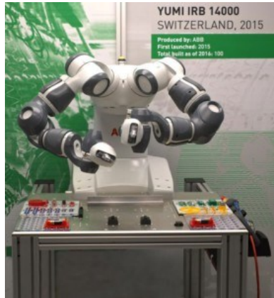
Figure 155: ABB YuMi robot (Image Anthony O'Neil under the CC-BY-SA 2.0 license)
