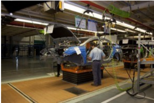
Figure 206: Hyundai moving walkable platform assembly line (Image Carol M. Highsmith in public domain)
