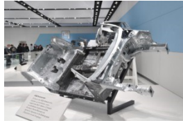
Figure 185: Volkswagen MQB floor assembly (Image Ra Boe under the CC-BY-SA 3.0 Germany license)
