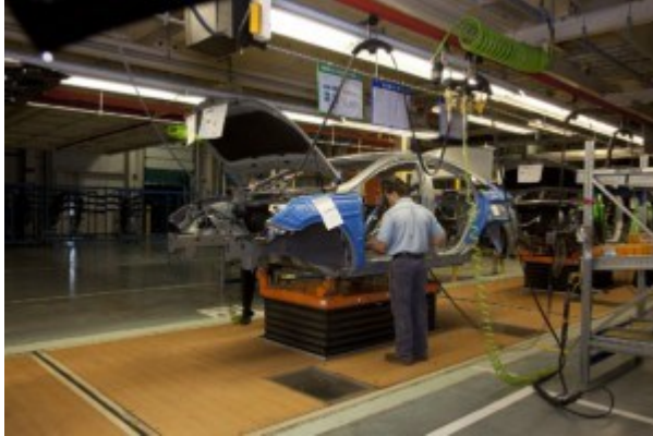
Figure 216: Hyundai moving walkable platform assembly line (Image Carol M. Highsmith in public domain)
