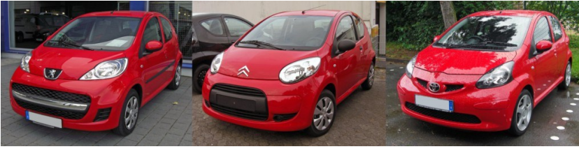
Figure 183: From left to right the Peugeot 107, the Citroën C1, and the Toyota Aygo (ca. 2009 models). Notice how the body is similar and only details differ. (Images M 93 in public domain)
