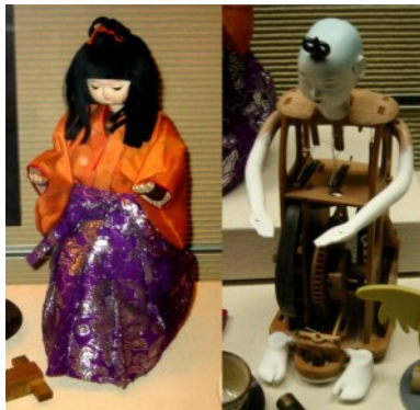
Figure 147: Karakuri Ningyo and its mechanism (Image World Imaging in public domain)
