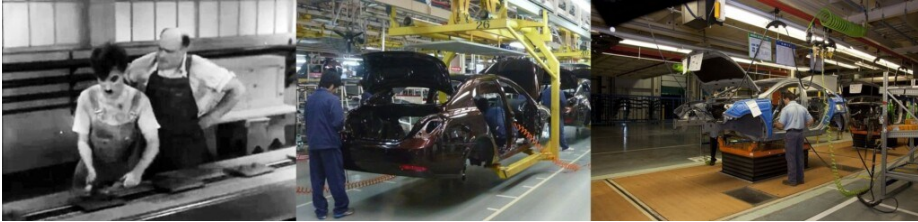
Figure 232: Types of Continuously Moving Assembly Lines (Image Charlie Chaplin in public domain; Siyuwj under the CC-BY-SA 3.0; Carol M. Highsmith in public domain)
