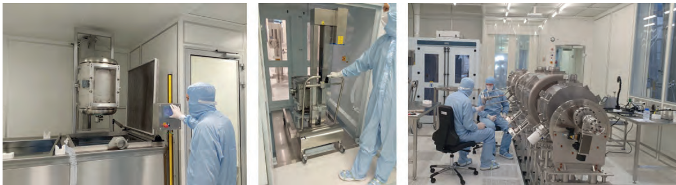
Figure 100. The CH0 cavity is lowered into the US bath using a special lifting frame (left). The solenoid S1 is set up in the HPR cabinet, aligned and prepared for rinsing (center). The power coupler is mounted to the coupling port of CH0 (right). All the activities shown carried out in the cleanroom laboratory at HIM.
