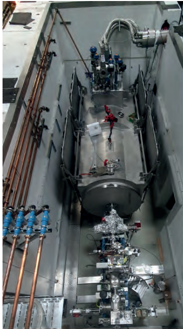
Figure 102. Left panel shows the first cryogenic module inside the test bunker at GSI. It is integrated into beamline and connected to cryogenic supply. Right panel shows the measured kinetic energy of accelerated \text{He}^{2+} ion beam.
