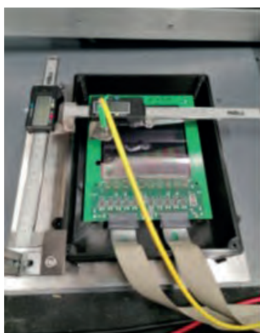
Figure 40. Setup for test of microstrip detectors with IR laser.
