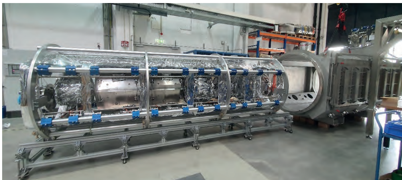
Figure 101. Fully assembled cold-string inside the segmented support frame, which is mounted on a rail system. This design enables smooth integration of the cold-mass into the cryostat. Here, the beam entrance is on the left-hand side of the cold-string.
