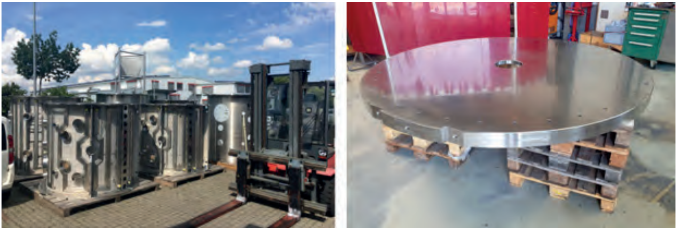
Figure 91. Tank sections of cavities AI and AIa at the supplier (left) and one of the four end plates after mechanical polishing (right).
