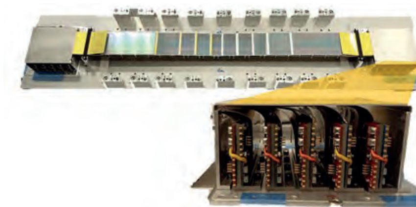
Figure 30. One of the first ladders of the series production on its mounting jig; the insert shows details of the FEB-box.
