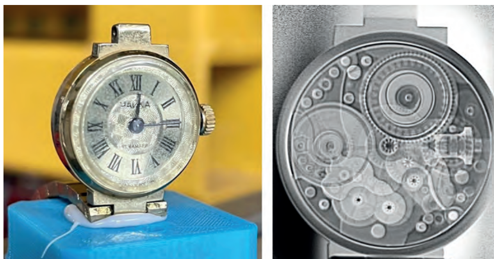
Figure 17. Carbon radiography of a small mechanical wristwatch captured with PRIOR-II using 975MeV/u ^{12}\text{C}^{6+} beams at the HHT experimental area.
