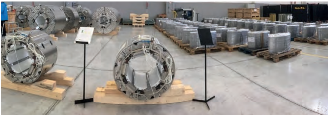
Figure 117. Storage of sc magnets at ASG, Italy
